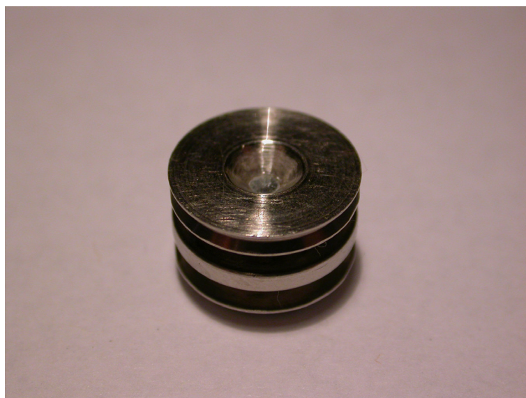
Figure 3.10: New designed stub for granular and powdered samples.
