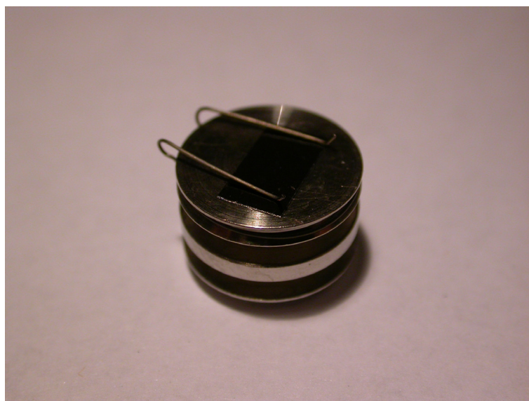
Figure 3.9: Standard stub with additional metal retaining clip.
