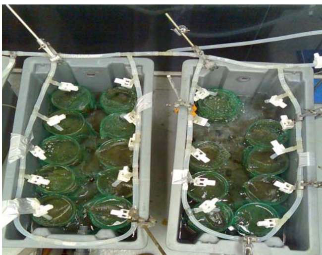
Fig 9.1: Experimental set-up showing exposure of N.virens to test sediments in 1 L glass beakers with flowing artificial sea water
