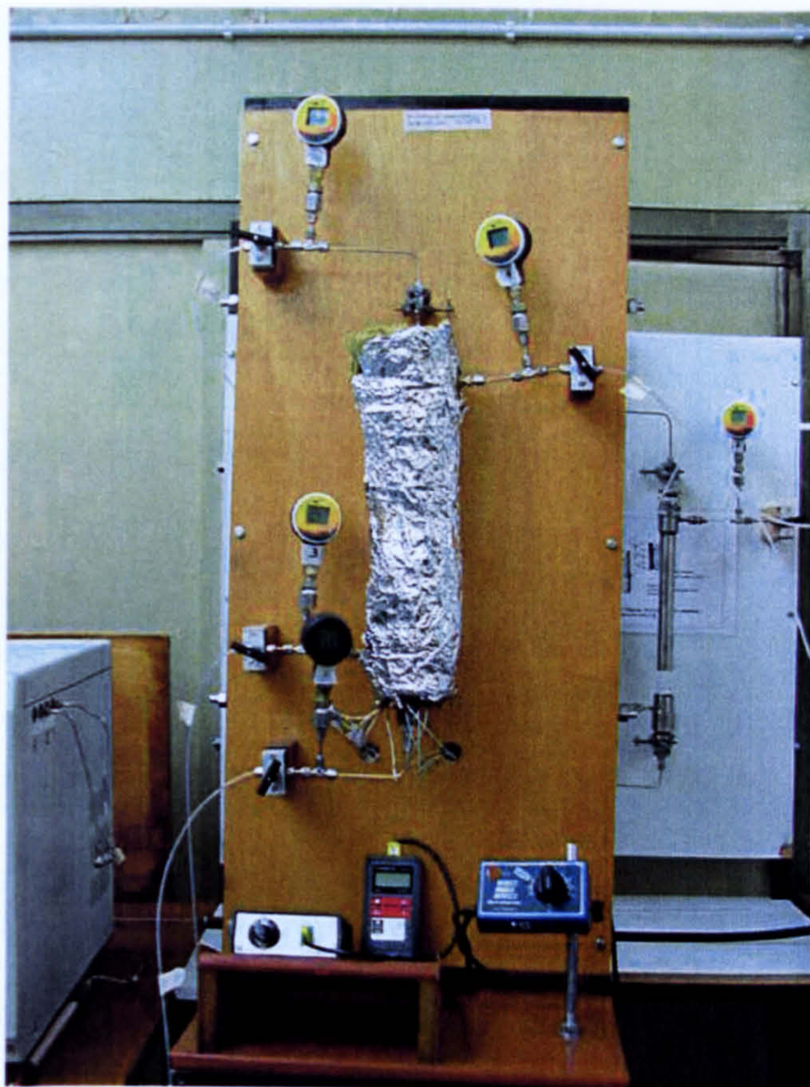
Figure 10: Pictorial view of the reactor section and heating system
