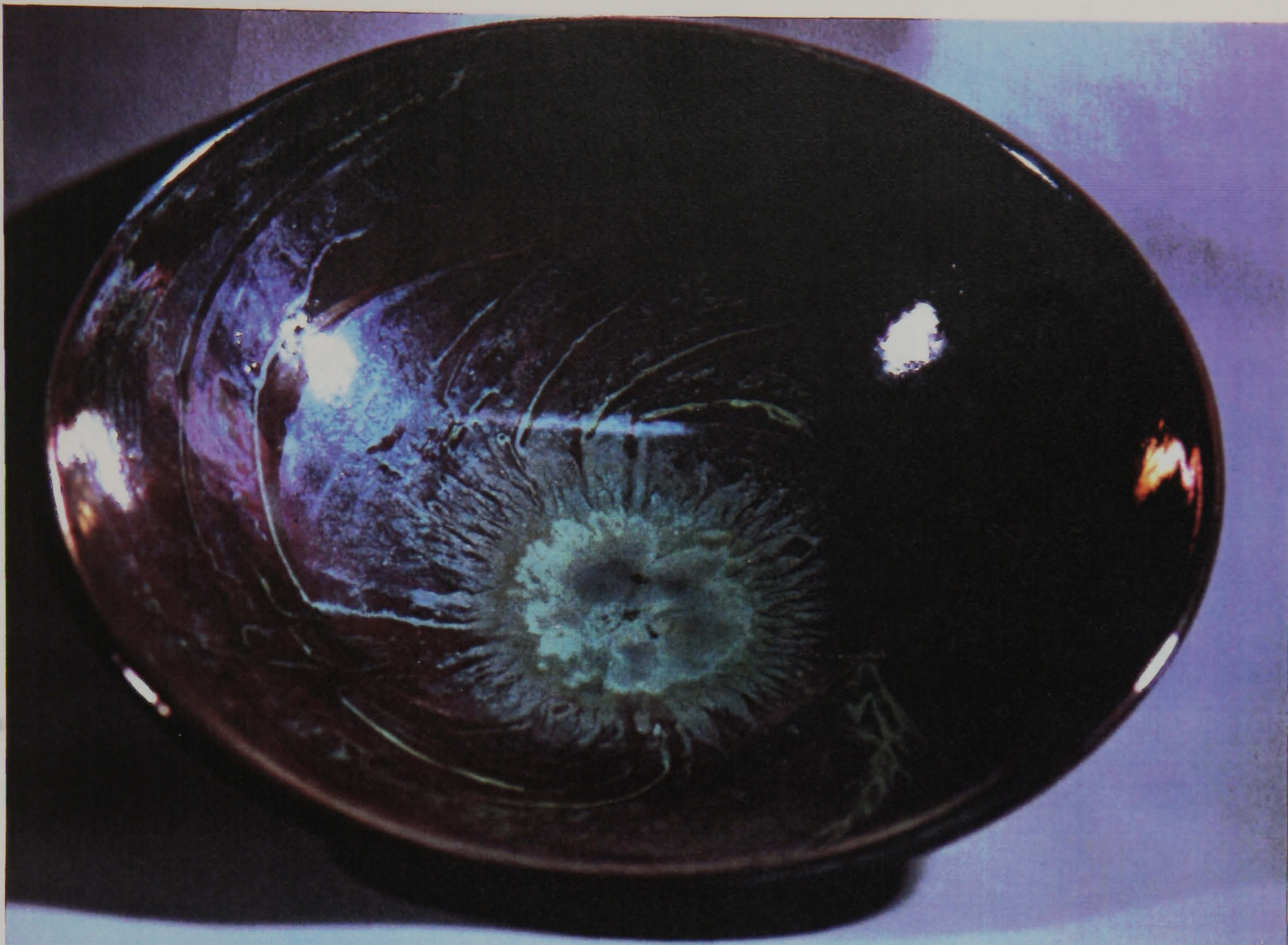
Figure 1.2 An example of a clay paste lustre used over a transparent glaze (#6, table 2.1). A black engobe has been used under the glaze. The clay paste was applied by brush and the bowl was fired in the down draft gas kiln described in section 5.2.1.
