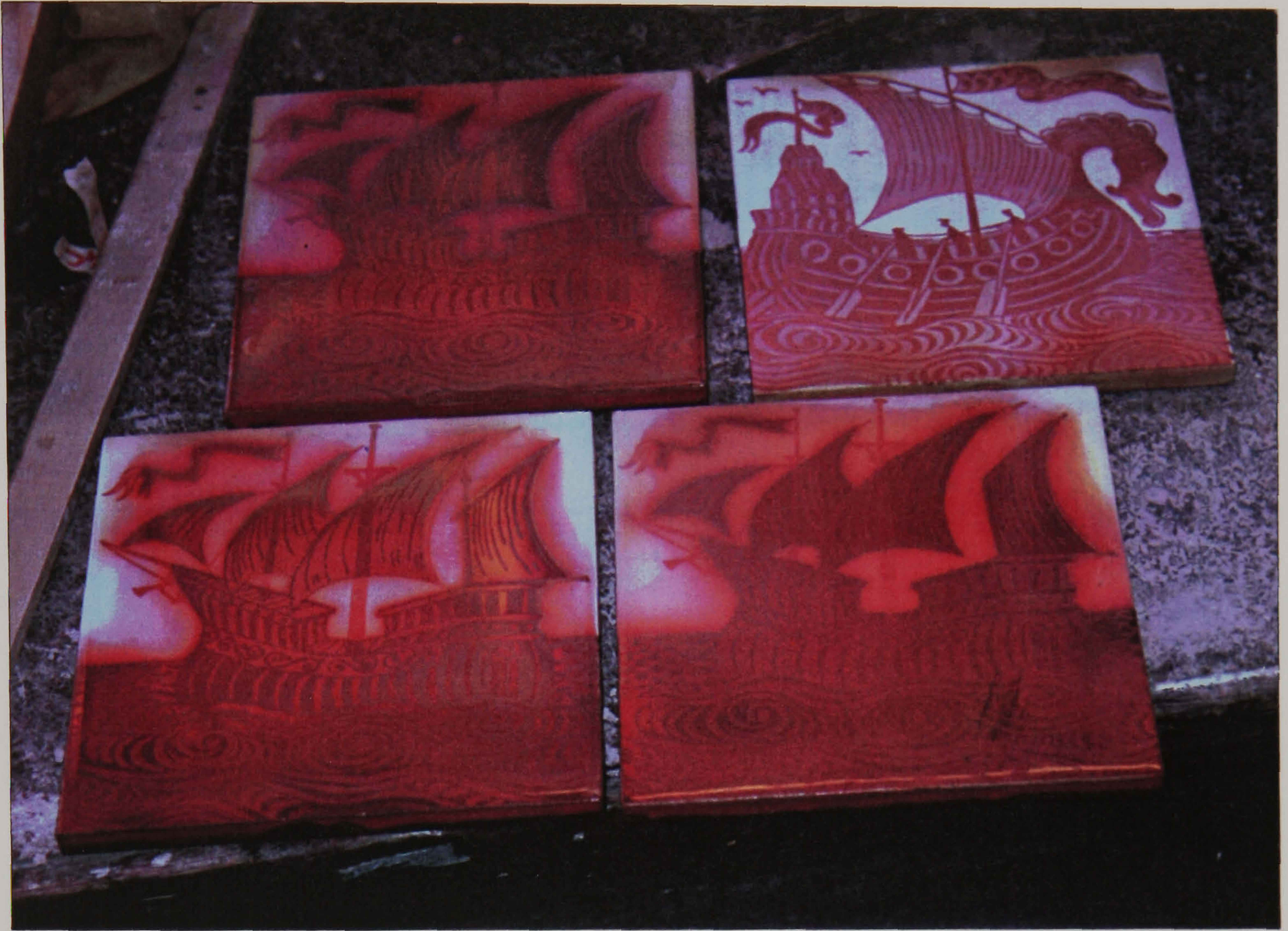
Figure 2.1 Screen printed tiles by Margery Clinton. The tiles were fired at differing temperatures. As the temperature increased more of the design is obscured by copper vapour.
