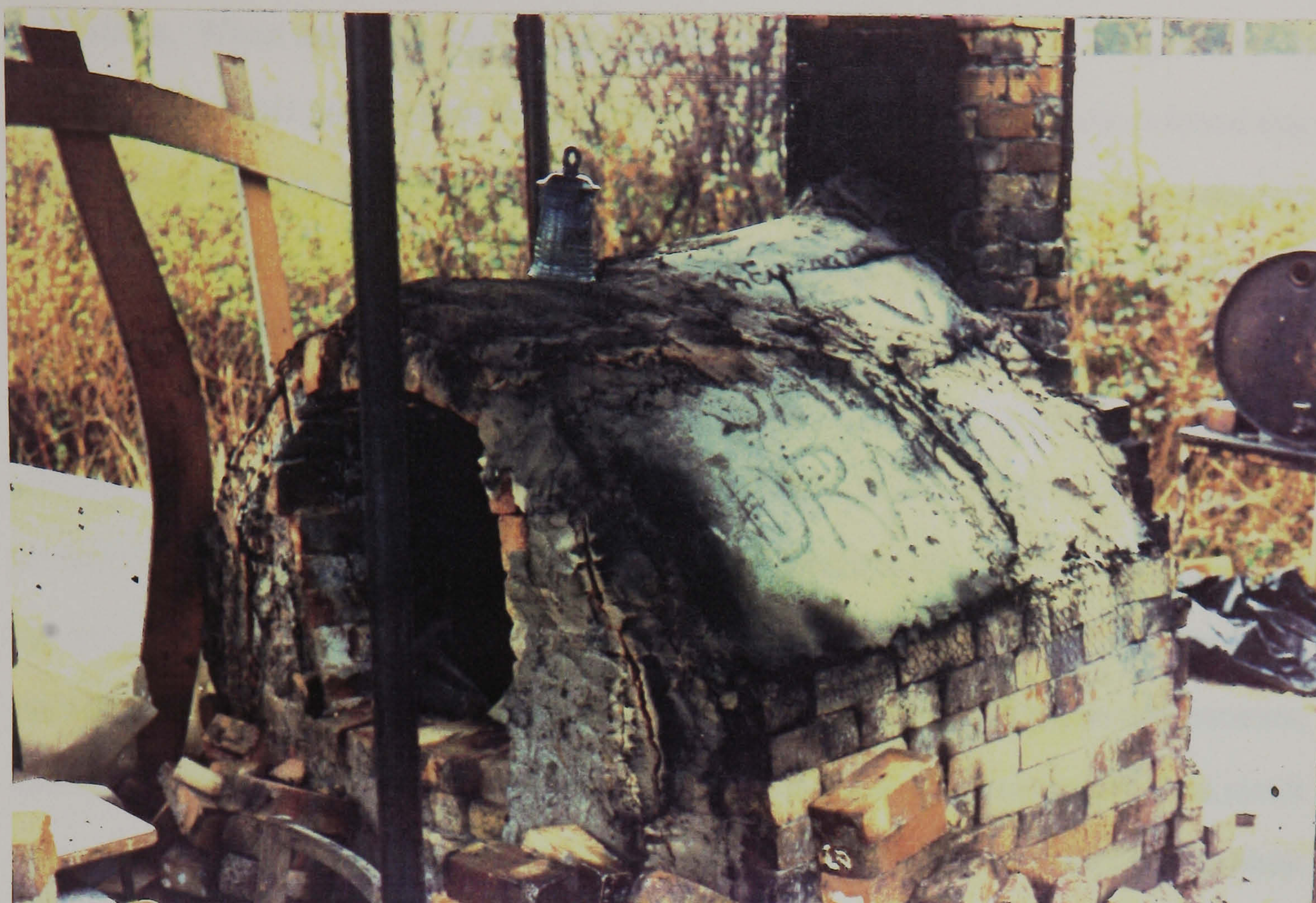
Figure 1.4 Conventional catenary arch salt kiln. The interior brick work has been badly affected by alkaline attack.
