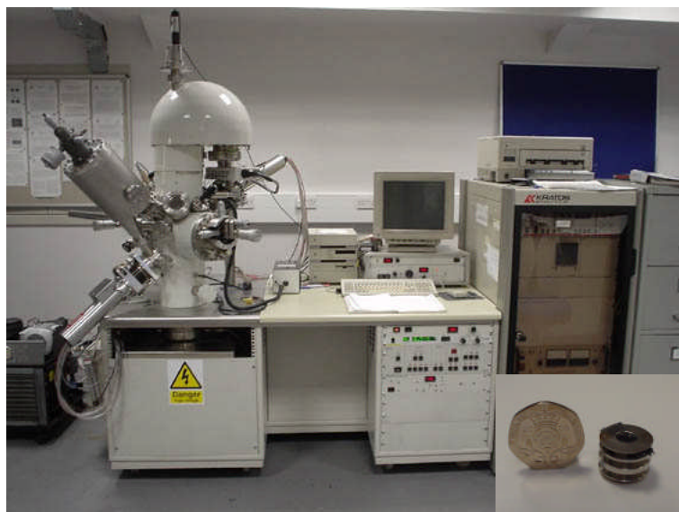
Figure 2.7 Kratos Axis x-ray photoelectron spectrometer and (inset) constant height stub.
