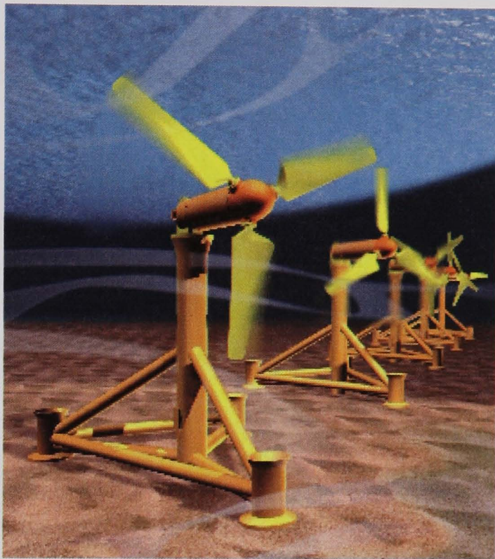
Figure 20: TGL Concept – Fully submerged tidal turbine
