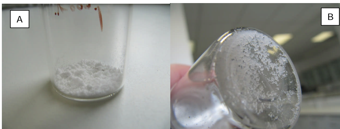
Figure 68. Images of, A. Batch 9 microspheres stored at 4°C for 1 week, and B. Batch 9 microspheres stored at 30°C, 75% RH for 1 week.
