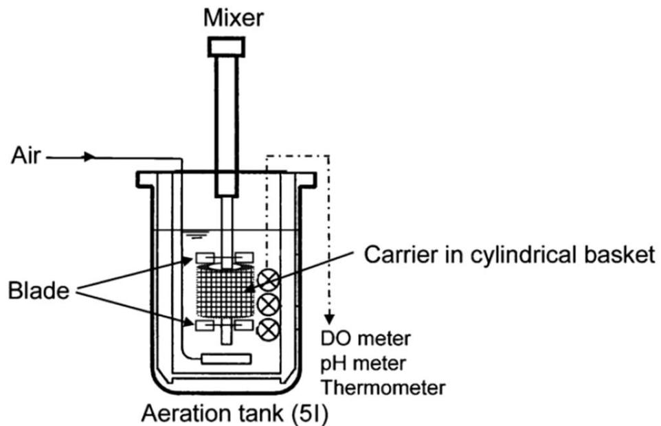
Figure 1.6 Bioreactor diagram using immobilised *Sphingomonas* sp. B9 for removal of MC from lake water (adapted from Tsuji *et al.*, 2006)
