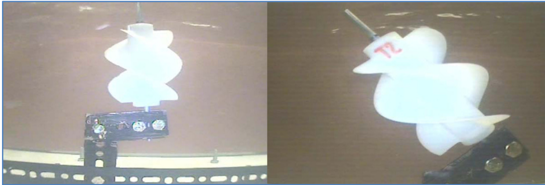
Figure 4.28: Blade trials with 'T2' in vertical position and at a 45 degree angle (copyright author)
