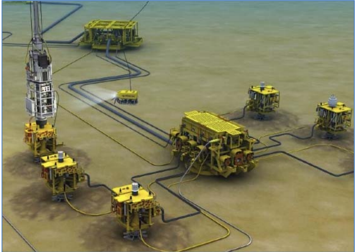
Figure 2.11: Example of central manifold surrounded by, and connected to, subsea trees (23)
