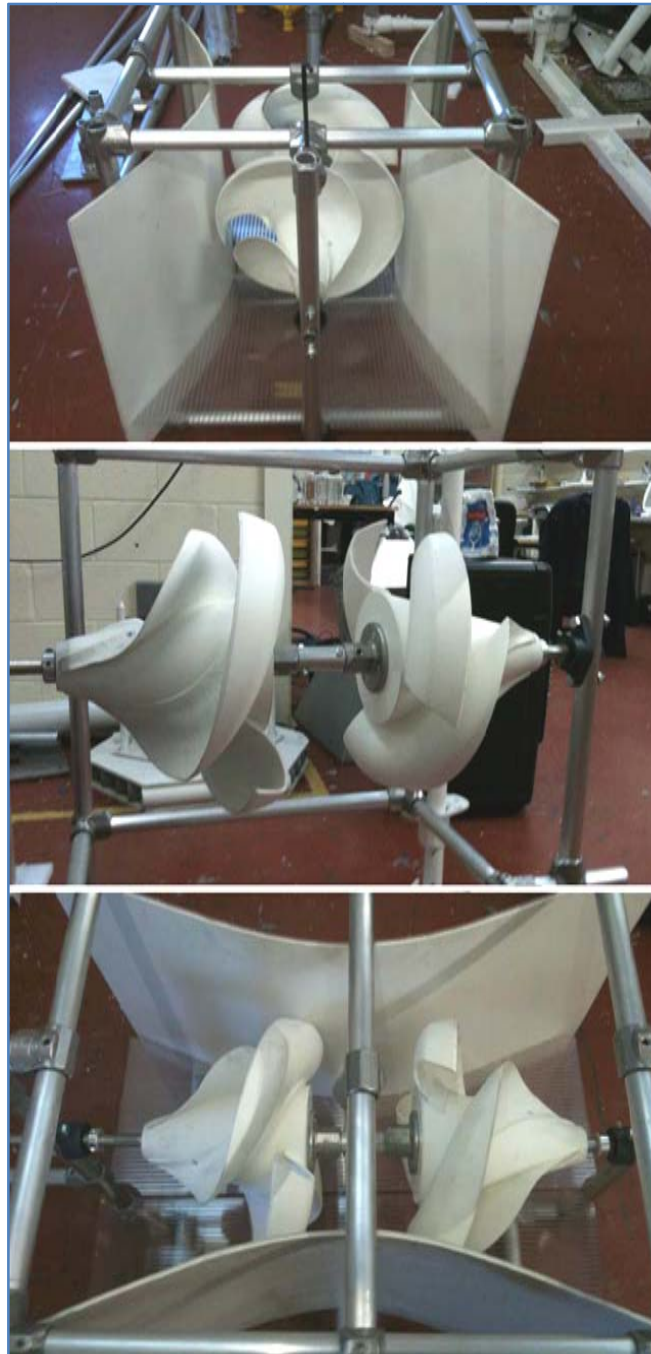
Figure 3.16: Prototype rotor/generator module
