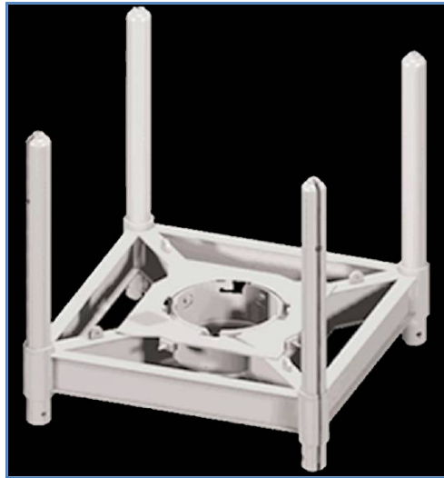
Figure 2.21: Schematic of subsea guidebase(11)
