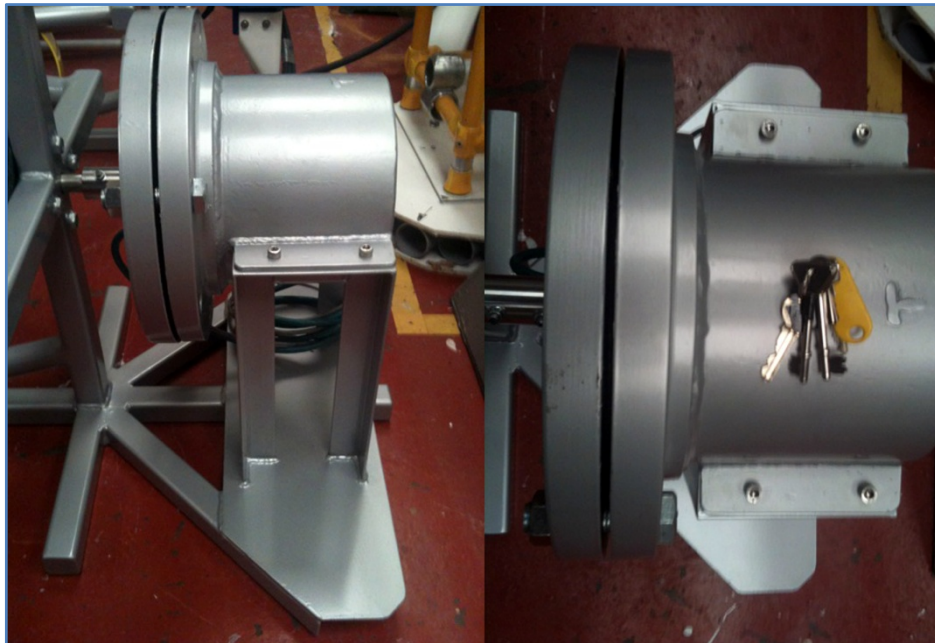
Figure 4.51: Final product for testing, marinised generator (copyright author)
