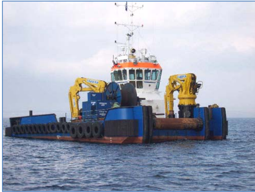
Figure 2.48: Damen 24m Multicat with twin 10MT cranes (54)
