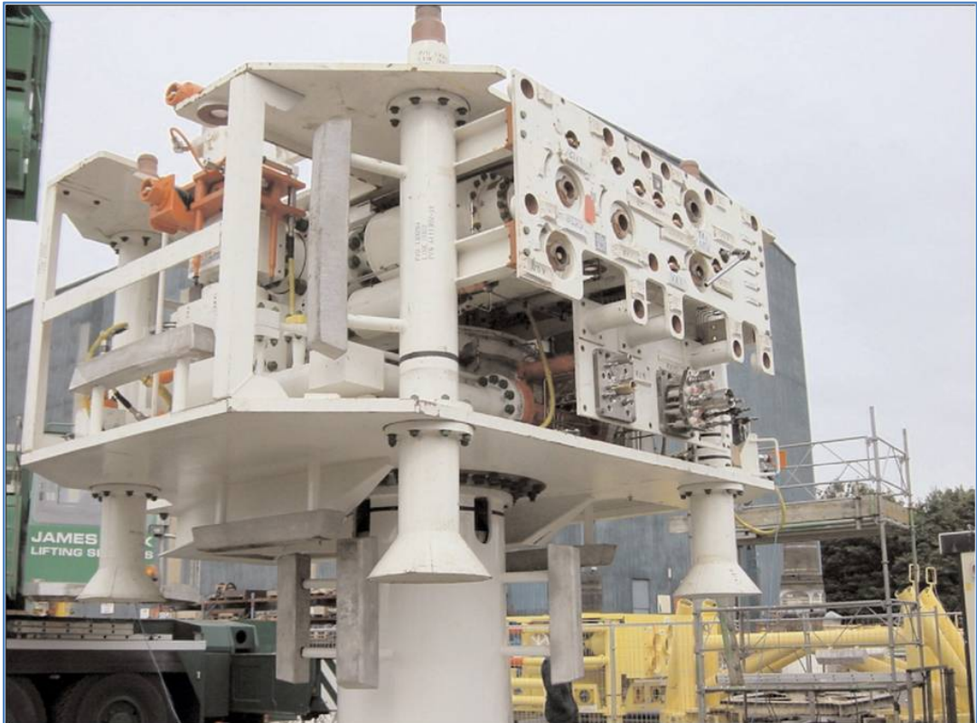
Figure 2.24: Tree being tested on dummy production guidebase (20)
