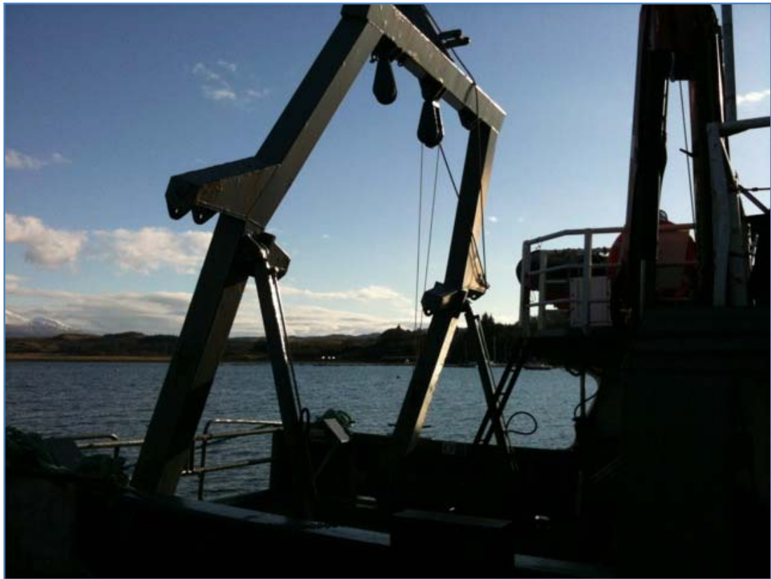
Figure 5.6: Oceanographic Vessel with 10MT A frame and large work area off stern (65)
