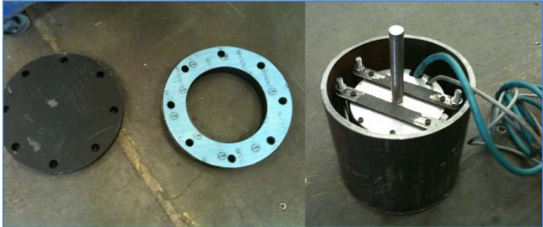
Figure 4.50: Generator housing construction (copyright author)
