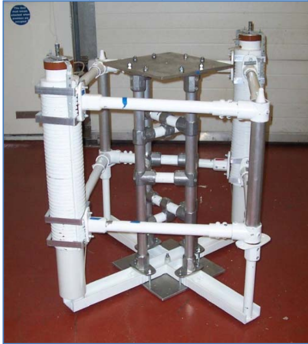
Figure 4.7: Completed frame, with guidebase and testing support structure (copyright author)
