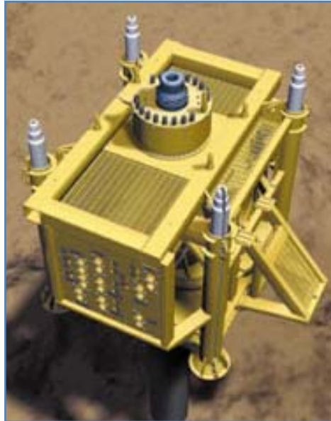
Figure 2.32: Final condition. Subsea tree attached to wellhead, ready for production (31)
