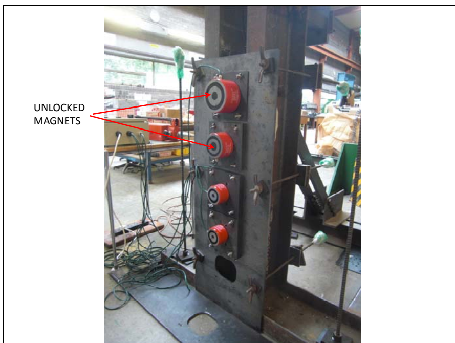
Figure 4.22: Vertical post removed, showing unlocked magnet arrangement (copyright author)
