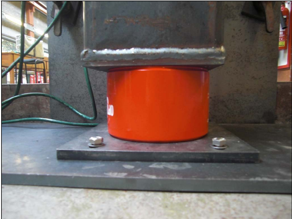
Figure 4.20: Actual test rig, front view, showing base magnet locked (copyright author)
