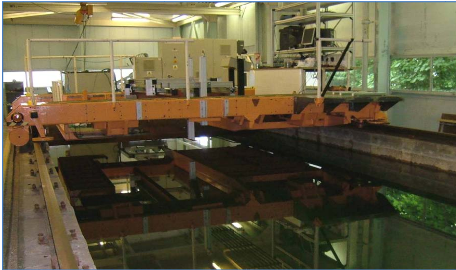
Figure 4.5: Strathclyde tow tank facility, showing towing carriage (copyright author)
