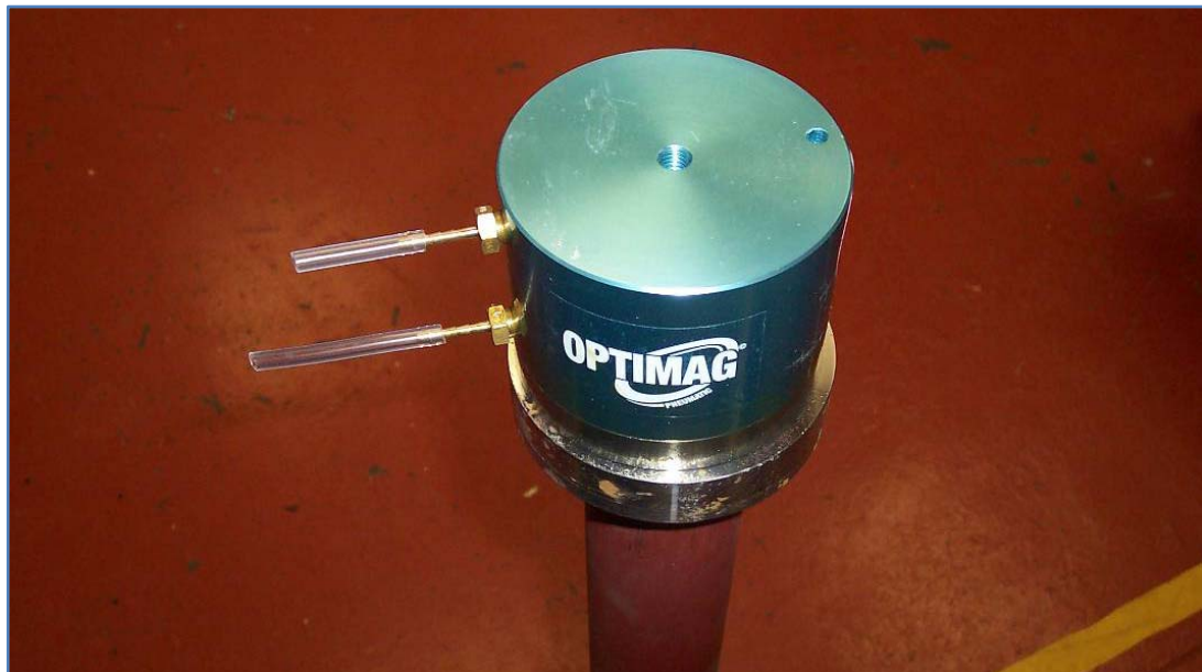
Figure 4.1: Pneumatically switchable permanent magnet being checked (copyright author)
