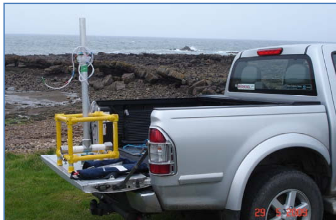
Figure 4.16: Magnet frame retrieved following one months submersion in seawater (copyright author)
