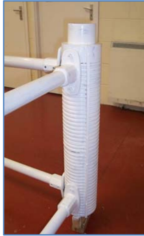
Figure 4.4: Guidepost and magnet housing corner-post sub-assemblies (copyright author)
