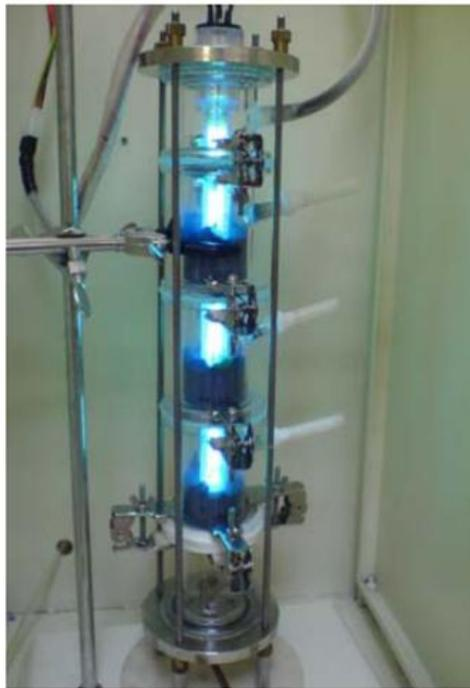
**Figure 21;** Image of three phase photocatalytic reactor used by Kuo *et al.* (2009) for the degradation of toluene
