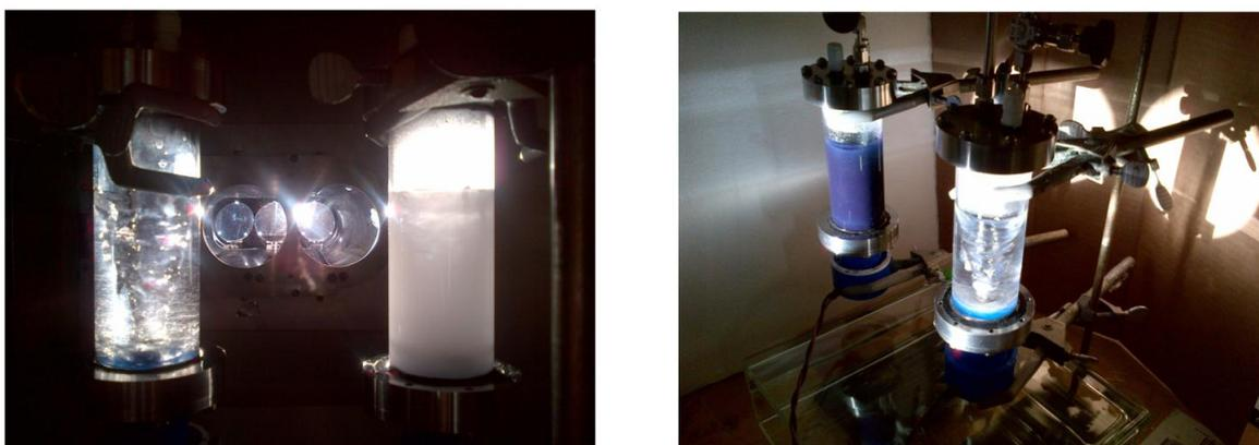
**Figure 89;** *PFPR under solar irradiation by the George Ellery Hale Solar Telescope*
