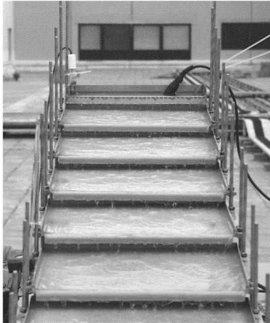
**Figure 48;** *Image of step-like SS structure used by Chan et al. (2003)*
