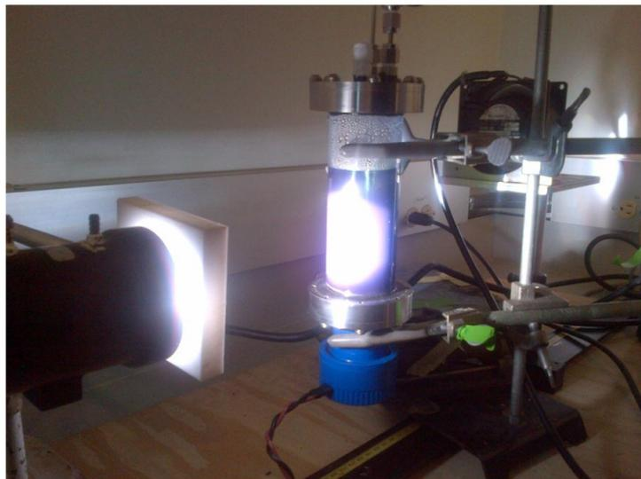
**Figure 78;** *PFPR Model II unit under irradiation from the 450 W Xe lamp*
