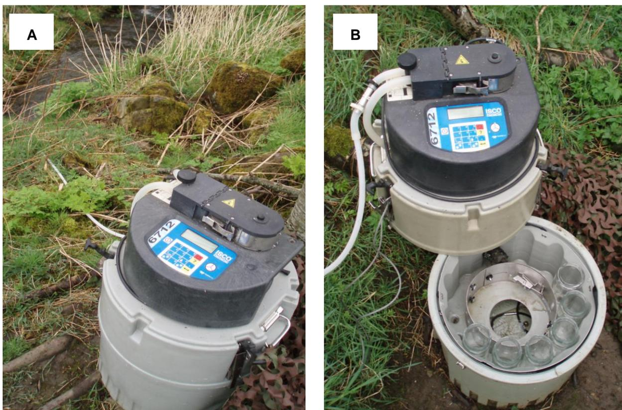
Figure 1-5 Automatic water samplers (autosamplers) at sample sites; Figure 1.5 B shows the tubing and bottles used to collect the waters samples.
