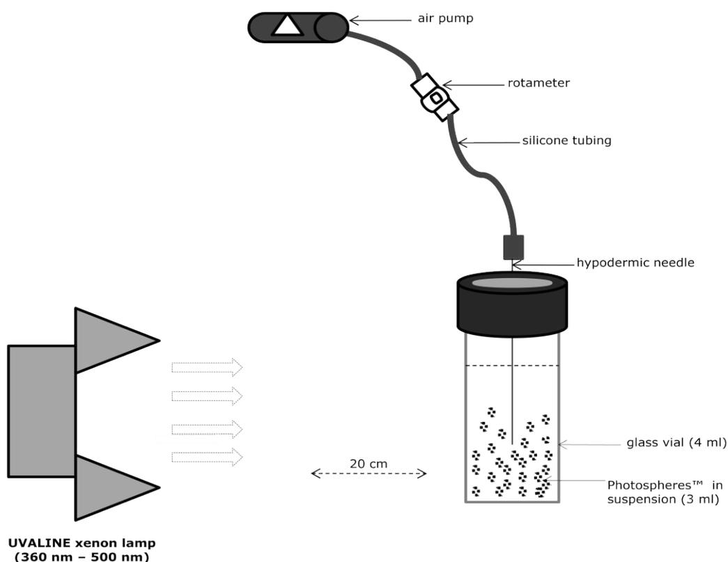
**Figure.4.5:** Experimental design of reactor model for the photodegradation of CYN by using Photospheres™ in sparged system.
