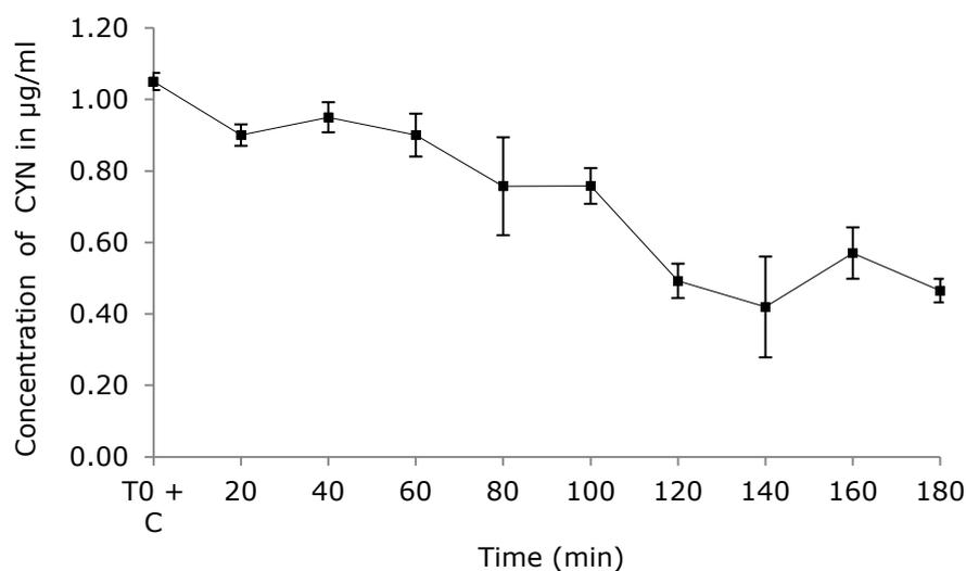
**Fig.4.17.** Photodegradation of CYN by using Photospheres™ with plate LED reactor (horizontal position). Duplicates were used for the experiments, (n=2); error bars equivalent to 1 standard deviation. All samples were concentrated by SPE prior to HPLC analysis.
