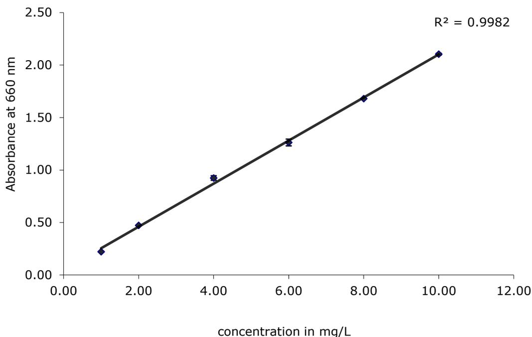
**Fig.4.8.** The calibration graphs for the proxy pollutant methylene blue (MB). Displayed with the graphs are the formula and the correlation coefficient ( $R^2$  value) determined at 660 nm. Triplicates were used, i.e.,  $n=3$ . Error Bars were equivalent to 1 standard deviation.
