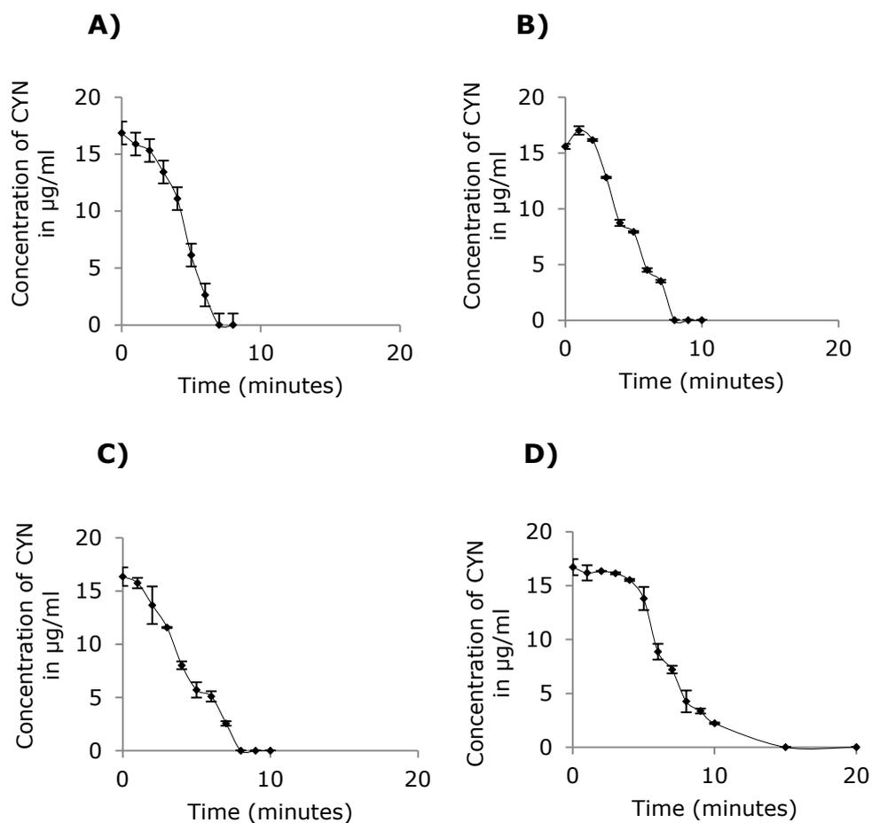
**Fig.4.16. A.** (0.8% w/v); **B.** (0.6% w/v); **C.** (0.4% w/v); **D.** (0.2% w/v) Photocatalytic degradation of CYN (20 µg/ml) by titanium dioxide variant photocatalysts™ at distance of 20 cm. Duplicates were used for the experiments, (n=2); Bars equivalent to 1 standard deviation.
