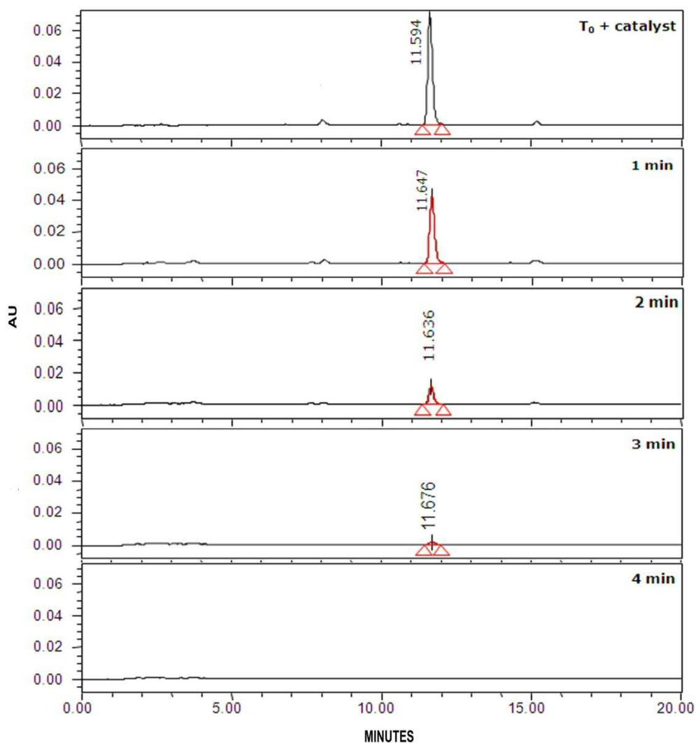
**Fig.4.11.** Chromatograms analysed by HPLC for the degradation of CYN with Degussa P25 catalyst at a light intensity  $1735 \mu\text{mol s}^{-1} \text{m}^{-2}$
