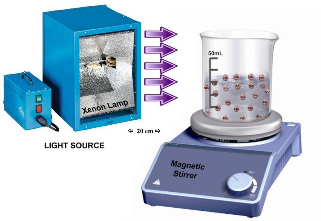
**Fig.4.4.** Standard experimental design using a Xenon lamp with unidirectional irradiation of the reaction vessel (50 ml glass beaker) containing aqueous suspension of TiO<sub>2</sub> in the presence of test sample.
