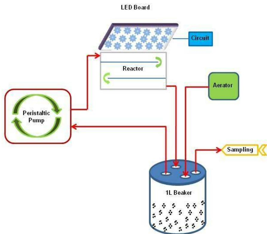
**Fig.4.6.** Schematic representation of novel LED photo reactor
