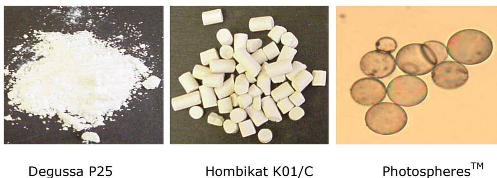
**Fig.4.3.** Different types of titanium dioxide photocatalysts.
