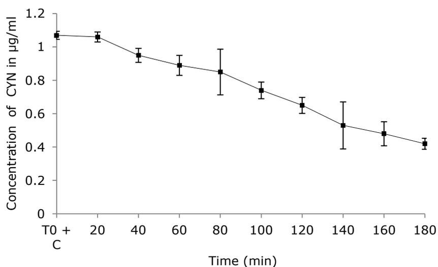
**Fig.4.18.** Photodegradation of CYN by using Photospheres™ with newly constructed LED reactor (vertical position). Duplicates were used for the experiments, (n=2); error bars equivalent to 1 standard deviation. All samples were concentrated by SPE prior to HPLC analysis.
