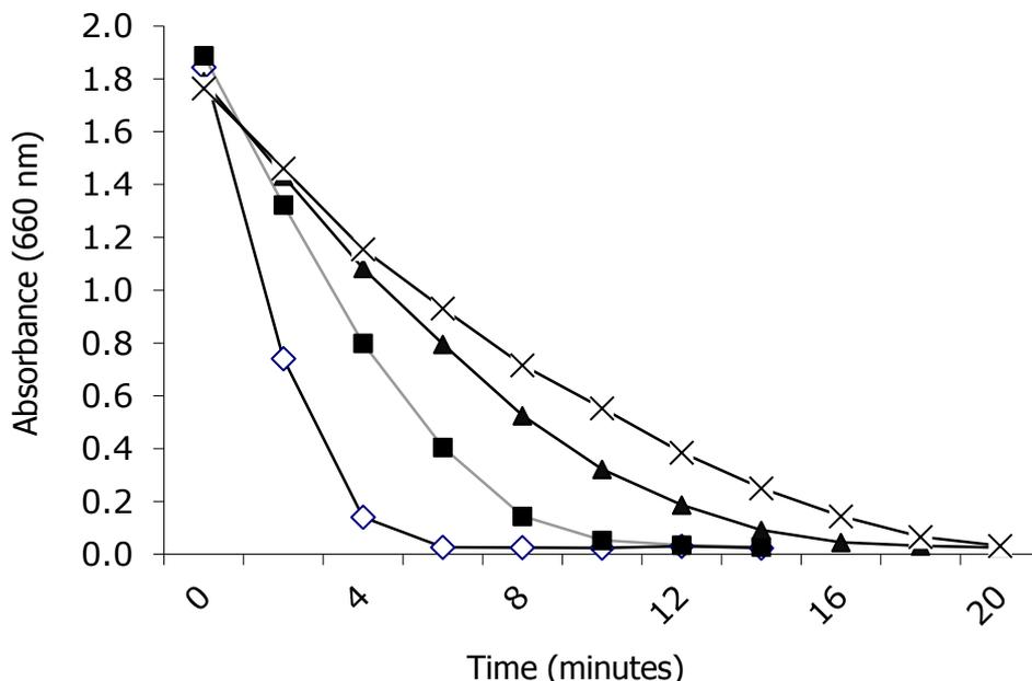
**Fig.4.9.** Photocatalytic degradation of methylene blue (10 mg/L) by using titanium dioxide catalyst P 25 (1 g/L) at range of different light intensities ( $\diamond$  1735  $\blacksquare$  1230  $\blacktriangle$  690  $\times$  415 ( $\mu\text{mol s}^{-1} \text{m}^{-2}$ ). Triplicates were used, i.e.,  $n=3$ . Error bars equivalent to 1 standard deviation.
