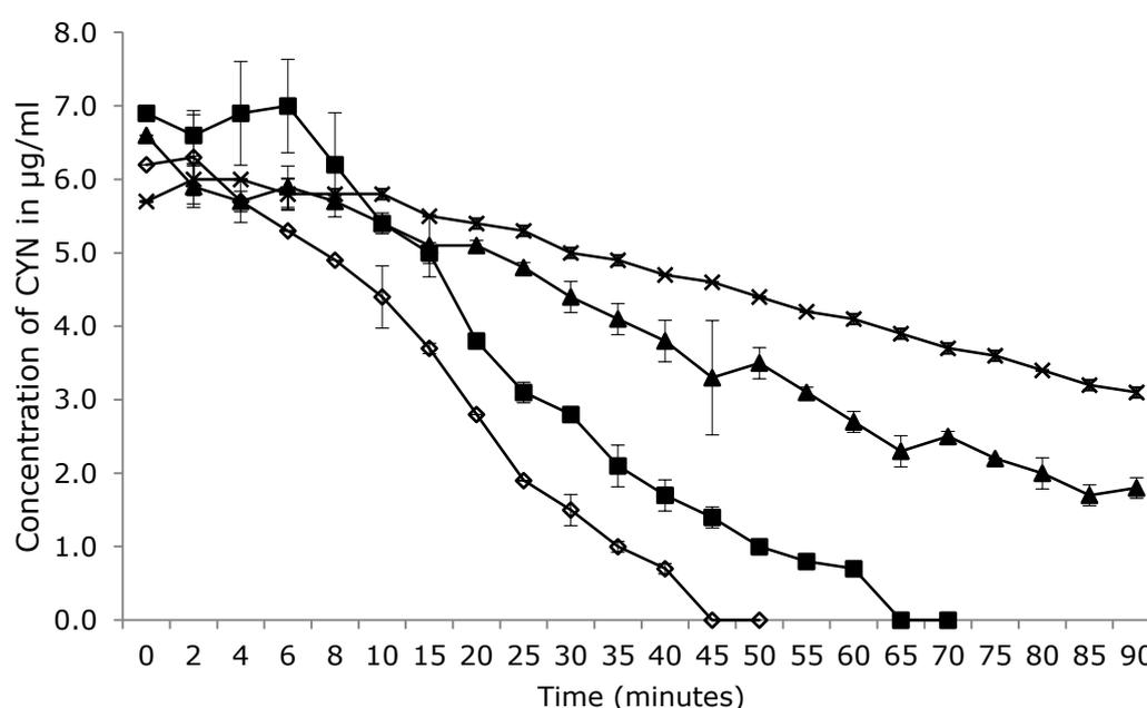
**Fig.4.12.** Photocatalytic degradation of cylindrospermopsin by using Hombikat K01/C catalyst load at a range of light intensities (◇ 1735 ■ 1230 ▲ 690 × 415  $\mu\text{mol s}^{-1} \text{m}^{-2}$ ) Triplicates were used in the experiments, i.e.,  $n=3$ . Bars equivalent to 1 standard deviation.
