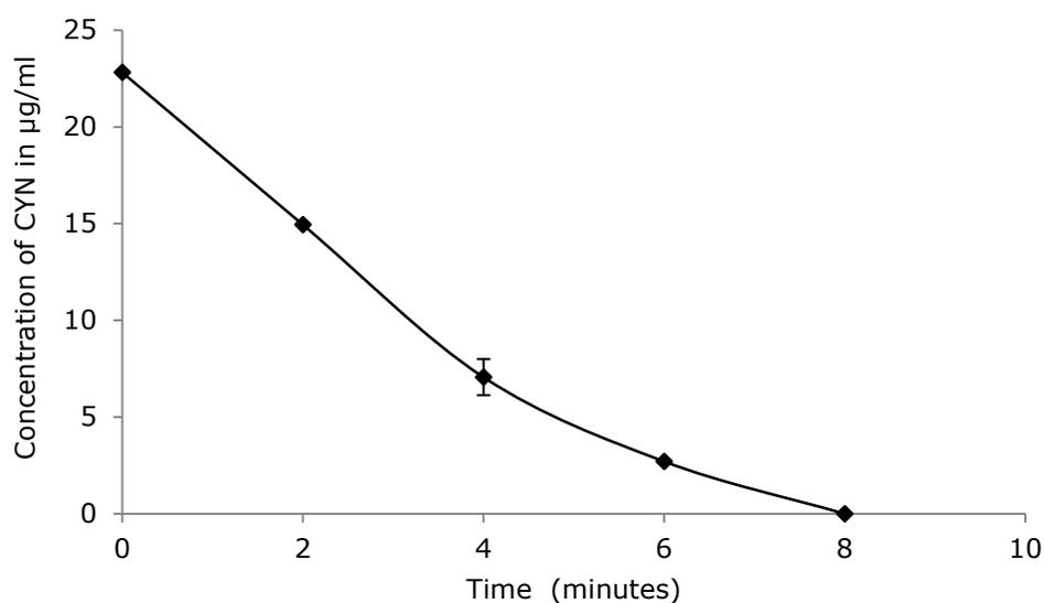
**Fig.4.14.** Photocatalytic degradation of cylindrospermopsin by using  $\text{TiO}_2$  P25 Degussa catalyst with a light intensity  $1230 \mu\text{mol s}^{-1} \text{m}^{-2}$ . Duplicates were used for the experiments, ( $n=2$ ) ; error bars equivalent to 1 standard deviation.
