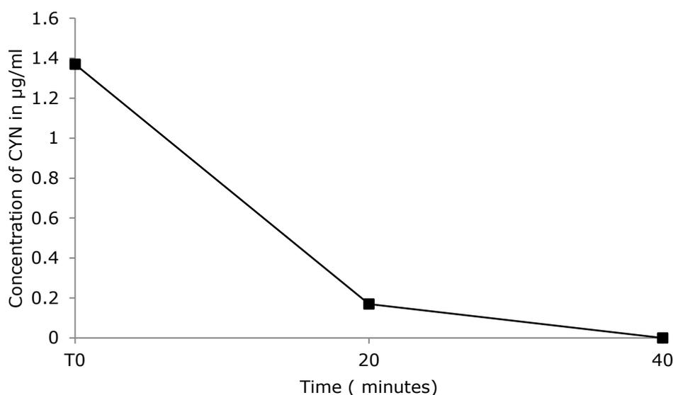
**Fig.4.19.** Photodegradation of CYN by using Photospheres™ with newly constructed reactor with UV xenon lamp as light source (reactor placed in vertical position). Duplicates were used for the experiments, (n=2); error bars equivalent to 1 standard deviation. All samples were concentrated by SPE prior to HPLC analysis.
