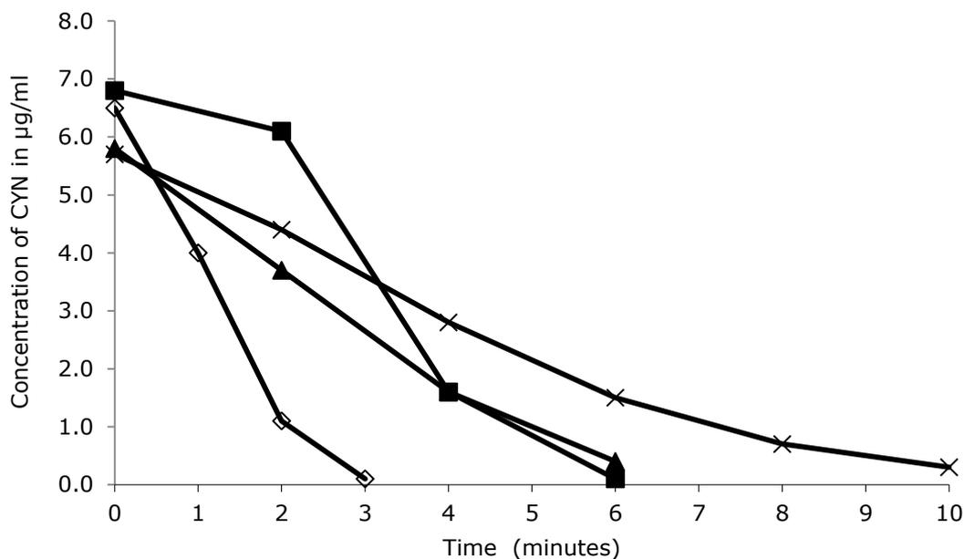
**Fig.4.10.** Photocatalytic degradation of cylindrospermopsin by using titanium dioxide catalyst P 25 Degussa at a range of light intensities (◇ 1735 ■ 1230 ▲ 690 × 415  $\mu\text{mol s}^{-1} \text{m}^{-2}$ ) Triplicates were used in the experiments, i.e., n=3. Bars equivalent to 1 standard deviation.
