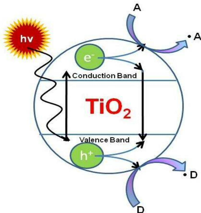
**Fig.4.1.** Hypothetical photocatalytic reactions occurring upon UV irradiation with TiO<sub>2</sub> alone. Note: A and •A represents acceptor molecules before and after reduction (for e.g., O<sub>2</sub> and •O<sub>2</sub>). D and •D represents donor molecules before and after oxidation, respectively (for e.g., OH<sup>-</sup> and •OH). (Modified from Krishna *et al.*, 2006)
