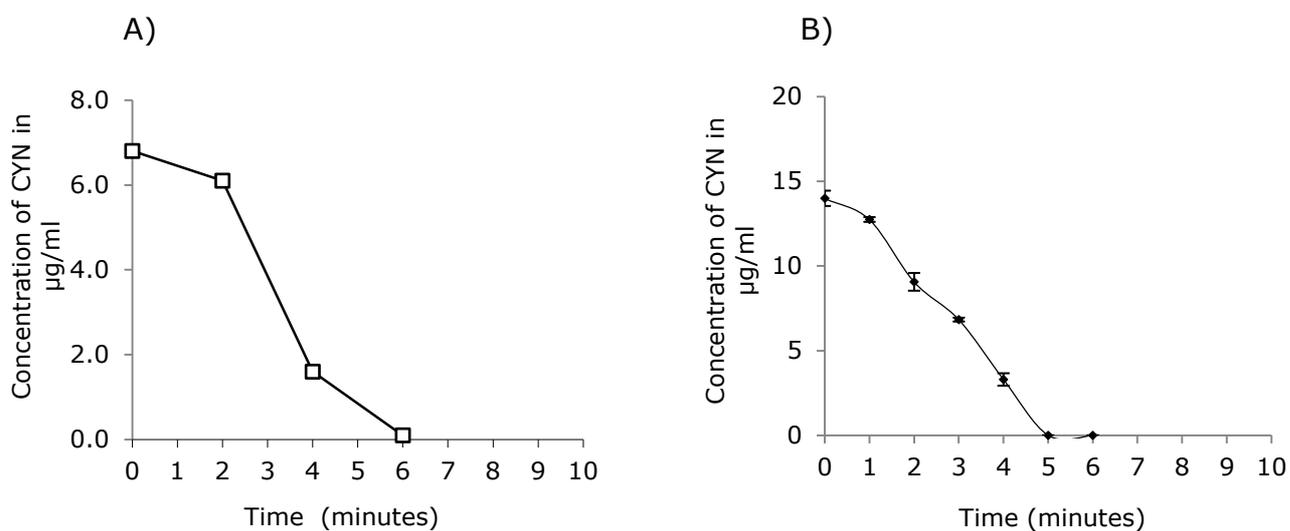
**Fig.4.15.** Comparison between two catalysts used for the photodegradation of CYN. With Degussa P25 (A) and Photospheres™ (B).
