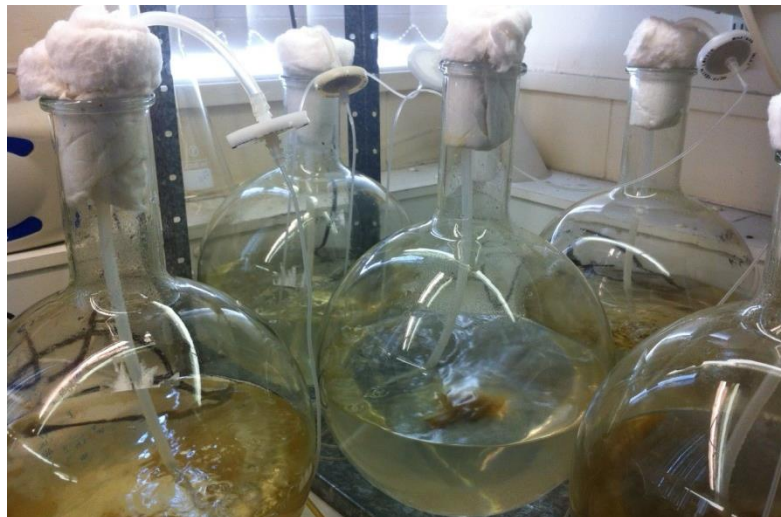
Figure 2.1 Prorocentrum lima CCAP 1136/11 grown in 10 L round flask under continuous exposure to light and filtered sterile air sparging.
