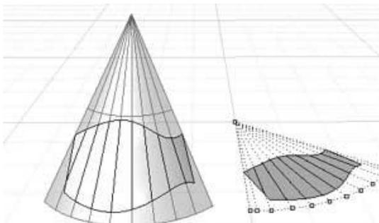
Once the underlying surface is developable, it can be trimmed in many ways using other geometries or intersecting planes.
