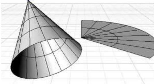
A developed surface is the consequence of unrolling a form where a modifier has been applied.
