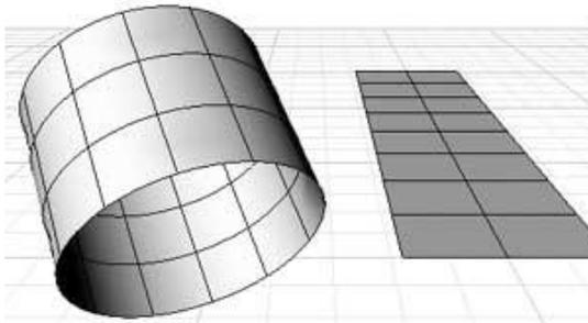
Developable surfaces can be formed by rolling a flat sheet of material without stretching it.
