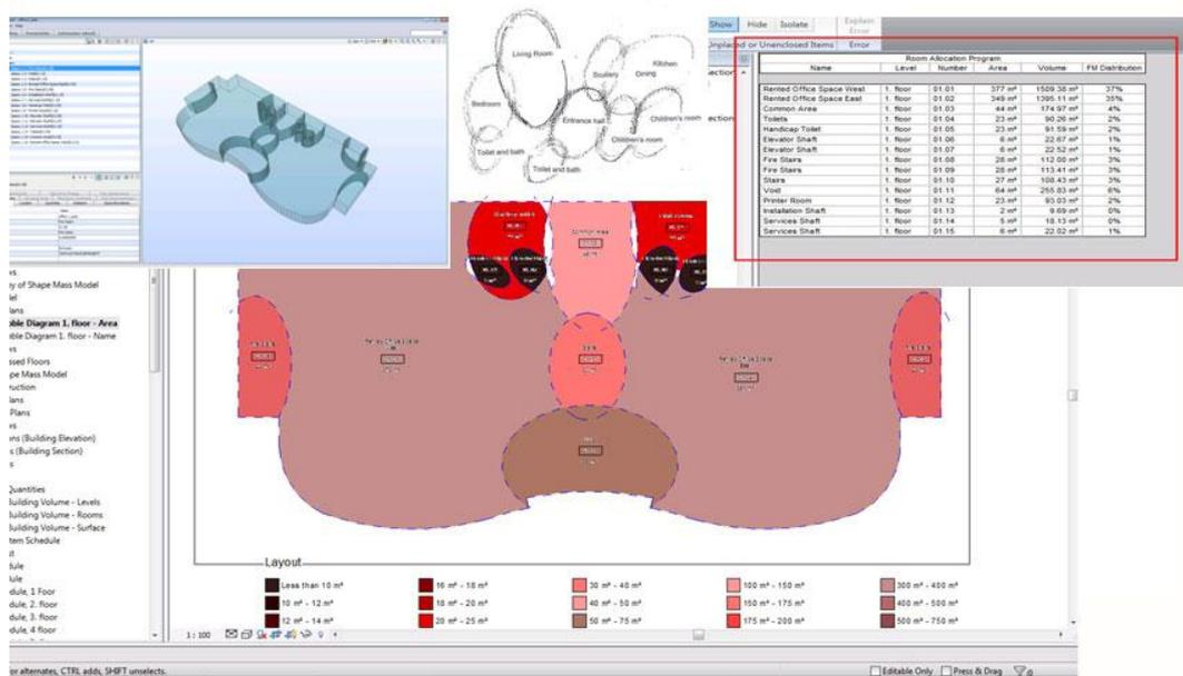
Figure 53 The bubble diagram can be imported into Revit using room separators as curved lines. These then can be populated with data, extracted as schedules and priced.
