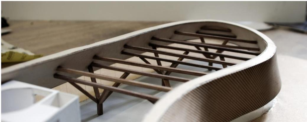
*A working model, showing the structural system and curved skin assembled*
