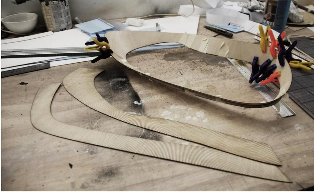
*A working model, showing that the developed shapes assemble into the correct form*
