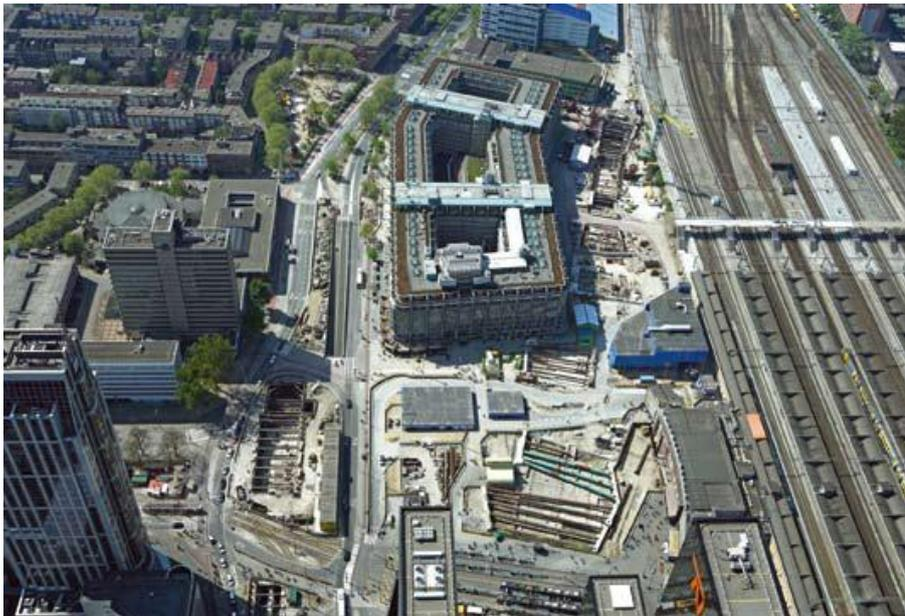
Figure 42 Work in progress. Left: the building pit for the new Weenatunnel. Right in front: the building pit for the underground
