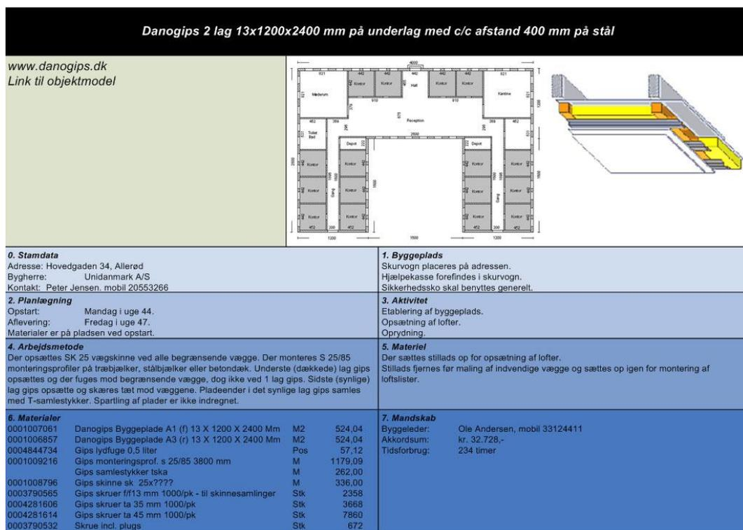
Figure 54 This is a Production Card, aimed at the sub-contractor. The plan shows where the work is to be done, the 3D view what is to be done and the table informs the worker where to go, when to go, what the specification is, what materials to bring, what is available to do the work and the manpower. Courtesy of Produktdata.dk
