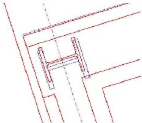
Figure 2 Differences in size and location of columns. Electronic overlay comparing two different drawings that had been approved for construction (architect's drawing – red, structural engineer's – blue). Source: [www.productioninformation.org/images/final/FigS12.gif](http://www.productioninformation.org/images/final/FigS12.gif)
