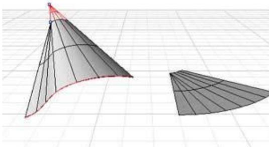
Developable surfaces can be created with parallel ruling lines by extruding any curve. Developable "cone-like" surfaces can follow any curve and can be created by lofting the curve to a point.
