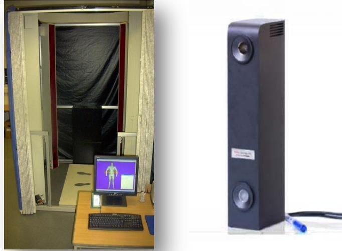
Figure 2. L: Hamamatsu BLS Scanner R: Artec L portable scanner
