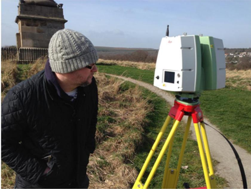
Fig. 1. 3D high definition laser scanner.
