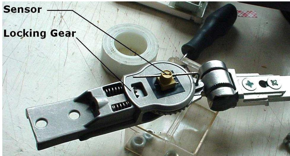
*Figure 5: the flexion/extension axis parts*
