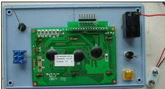
Figure 5: Control devices trial fitted
