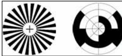
*Figure 1: Example of a forty-eight segment disk (left) and three-bit Gray code disk (right).*
