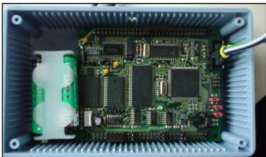
Figure 7: Microcontroller and battery pack test fit
