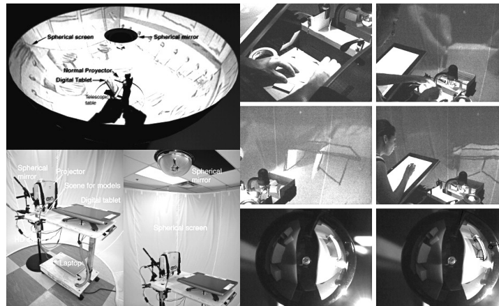
Figure 4.2: Immersive spherical graphical template – spherical sketch- captured image – spherical sketch over the image (Dorta, Pérez et al. 2008).
