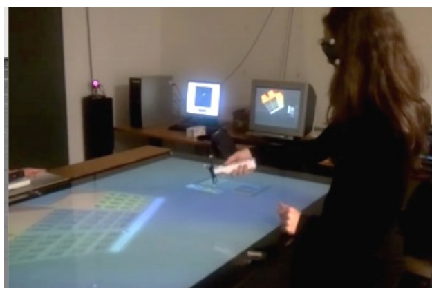
Figure 3.10 Kinect camera and Gametrak for direct 3D modelling (Araujo, Jorge et al. 2012). pp. 419-428.
