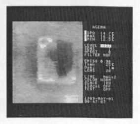
Figure 2.5.1: Internal view of the vent blowing cold air into the room (blue).
