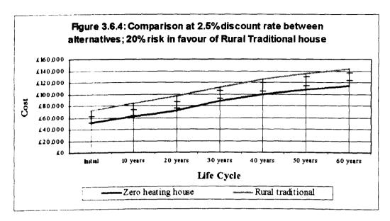
As the discount rate increases, up to 10% in *figure 3.6.2*, the life cycle curve gradually becomes horizontal. Due to the capital saving, the 'zero heating' family home will remain the preferred alternative at higher discount rates also. Occupancy costs at discount rates at 10% or higher have little or no significance after the first twenty to thirty years.
