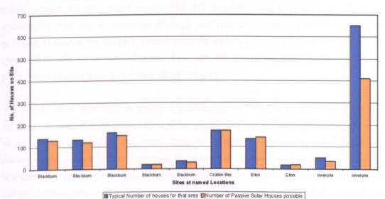
Number of Homes using Current Methods of Construction against Max Number of Passive Solar Houses on Sites Around the North East of Scotland at Latitudes between 57'11-57'25
