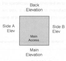
Fig 6.5.2.1 : The naming of elevations for the housing database
