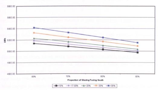
kWh of Passive Model dependant on Glazing to Floor Area Ratio (Double Glazed)
