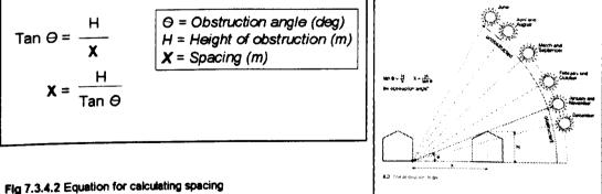
Fig 7.3.4.2 Equation for calculating spacing (Yannas, [1], 1994, p52)
