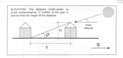
Fig 6.4.2.1 : Diagram of the overshadowing distance of passive solar designs (Yannas, [1], 1994)
