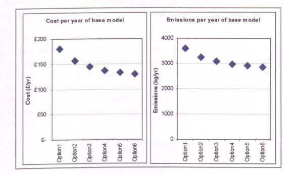
Fig 6.7.1.3 : Cost and emissions of a home with increasing thermal efficiency
