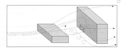
Fig: 3.4.5.5; Typical air flow pattern in mixed use development (Smith, et al, 1982)
