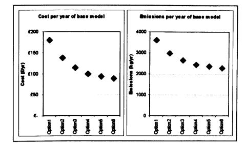
Fig 6.7.3.2 : Cost and emissions of a home combing better air-tightness with greater thermal efficiency
