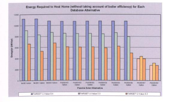
Fig 6.7.5.8 Energy required (without addition for boiler efficiency) for each database alternative
