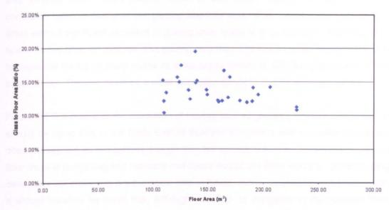
Fig 6.5.3.4 : Floor area against glass to floor area ratio of each house type (Roof-space homes only)
