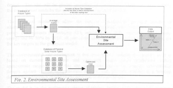
In addition to the databases created for standard and passive housing types, databases have been embedded into the assessment procedure so as to select appropriate housing types. These databases are needed to determine elements of simplified housing types, such as storey height and house footprint, in order to establish key passive solar trade-offs between current methods of construction and passive solar.
