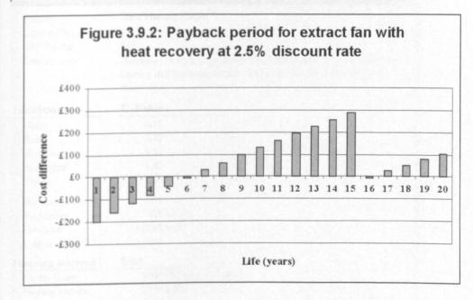
Due to the life cycle of the heat recovery unit, in this example, being 15 years the heat recovery unit is briefly not economic before achieving payback within the 16 year. It should also be noted that since the heat recovery unit requires more regular removal, disposal and subsequent installation additional costs for such work will created through builders work and overheads.
