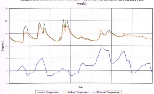
Comparison of External and Internal Temperature in the Zero-Heat House (one
