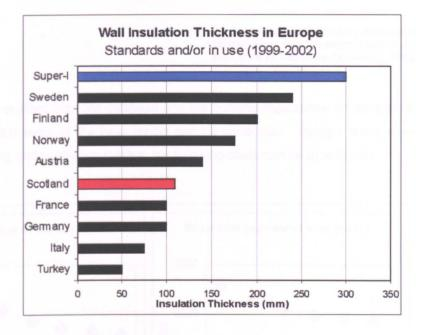
Fig 6.7.1.1 : Wall insulation thickness in various European countries (adapted from various sources)
