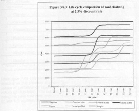
From figure 3.8.3 clay roof tiles are the best alternative between 55 and 65 years. This is due to the life cycle of clay roof tiles being 65 years enabling this alternative, for a brief period, being the best alternative. Clay roof tiles provide quite a low capital cost with average life span occupancy cost schedule. Therefore for the purposes of this study, which is intended to last 60 years, clay roof-tiles are the best alternative.
