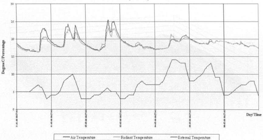
Figure 7.4a: Comparison of External and Internal Temperature in the Zero-Heat House (week 2)
