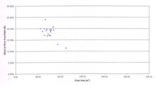
Correlation between floor area and glass to floor area ration (for Terraced and Semi-detached housing in Scotland)
