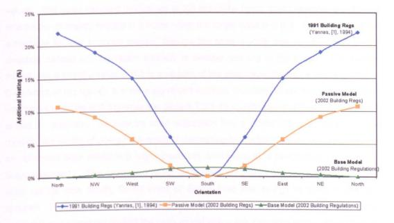
Additional Heating Input for Different Orientations for Three Different Models
