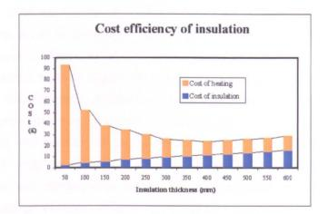
Fig 6.7.1.2 : Cost efficiency of insulation (Source:- Borer, Pat; The Whole House Book, The Centre for Alternative Technology, 1998)
