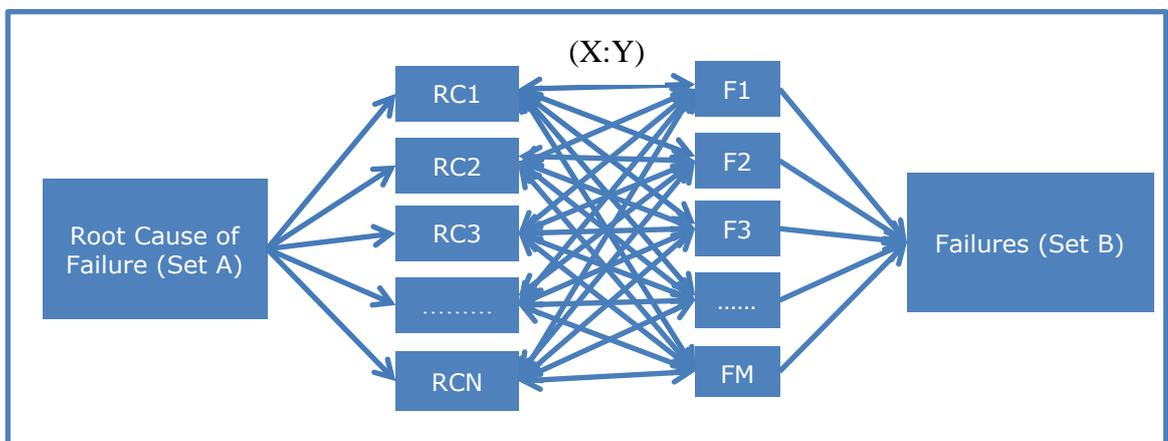
**Figure 3.19 Estimating the probability of a failure if root cause and failures are related by generic X:Y relationship**
