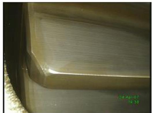
Picture 4: Planet wheel, sun wheel-active flank
