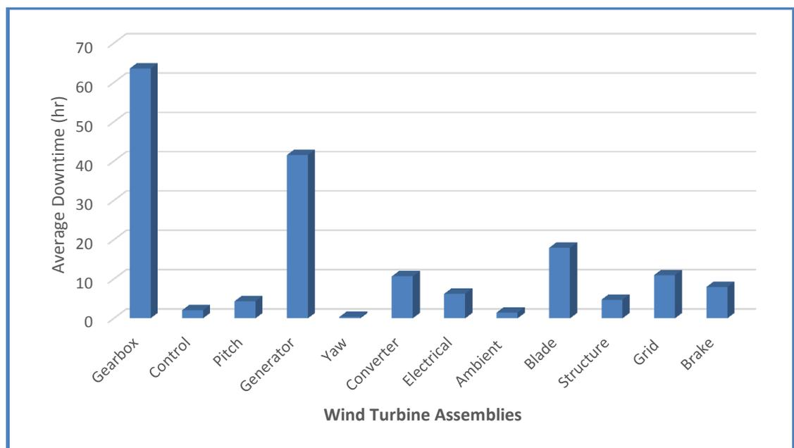
**Figure 2.3 Plot of wind turbine assemblies and their average downtime (Source: Quail and McMillan, 2012)**
