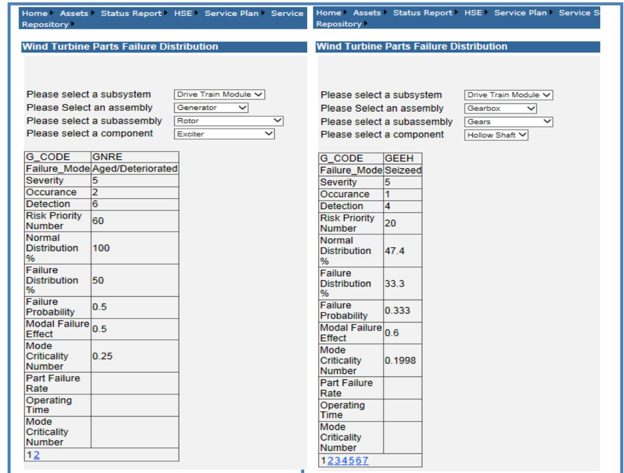
**Figure 4.11 Shows OWT-MOT capability to display information about failure distribution for two different instances**
