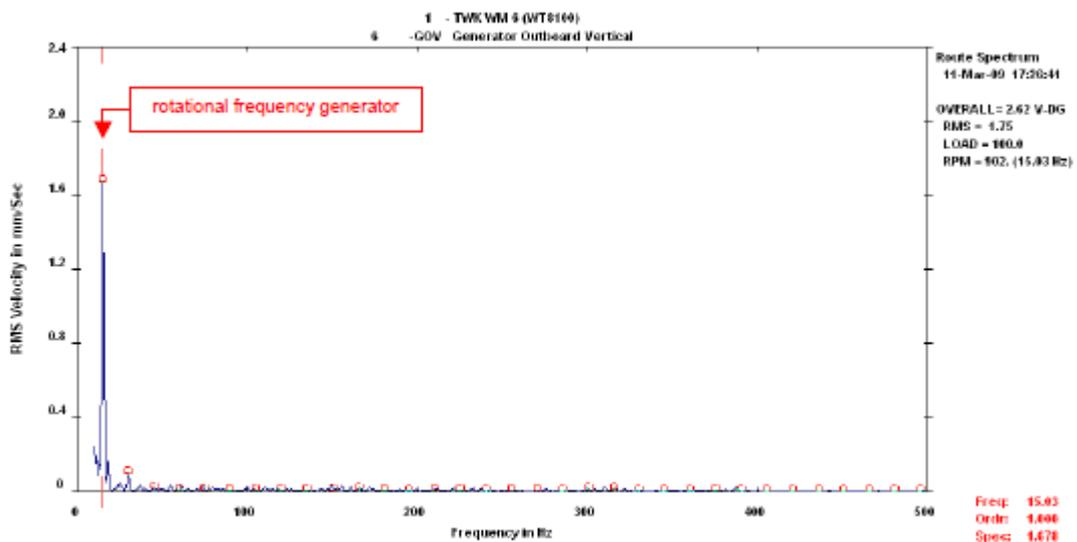
Figure 1: Spectrum at generator, non-driven end, vertical
