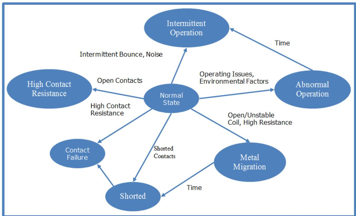
**Figure 3.23 Shows the transitions between failures due to various root causes of failures (Example 2: Case of a Relay)**
