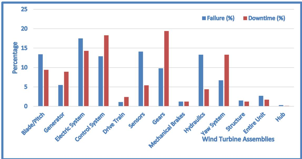
Figure 2.4 Plot of the percentage failure and percentage downtime of Swedish wind turbines during 2000-2004 (Source: Ribrant and Bertling, 2007)
