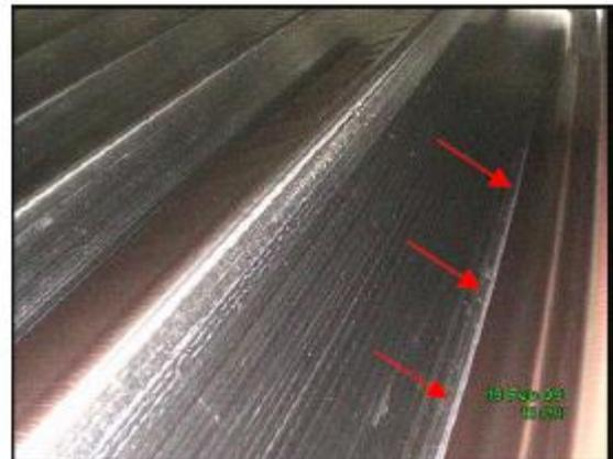
Picture 14: high speed planetary stage, ring gear, active flank
