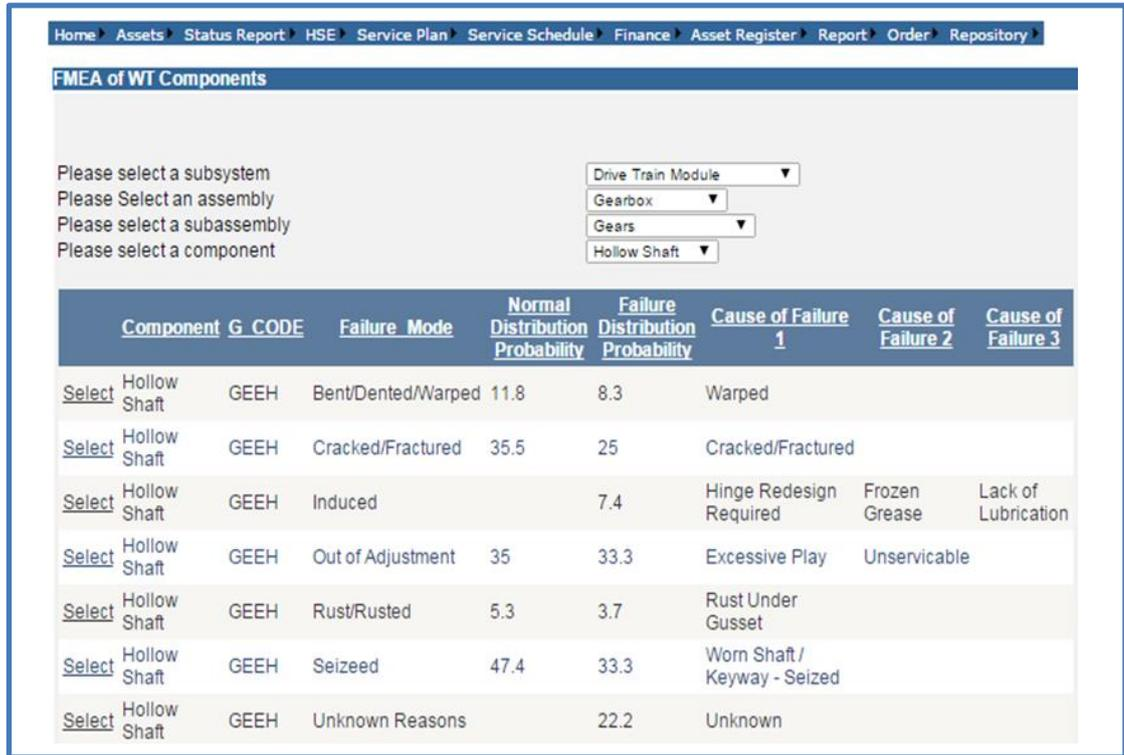
Figure 4.10 (b) Screenshot shows some results obtained from development of failure analysis tool module of OWT-MOT (Gear Hollow Shaft)
