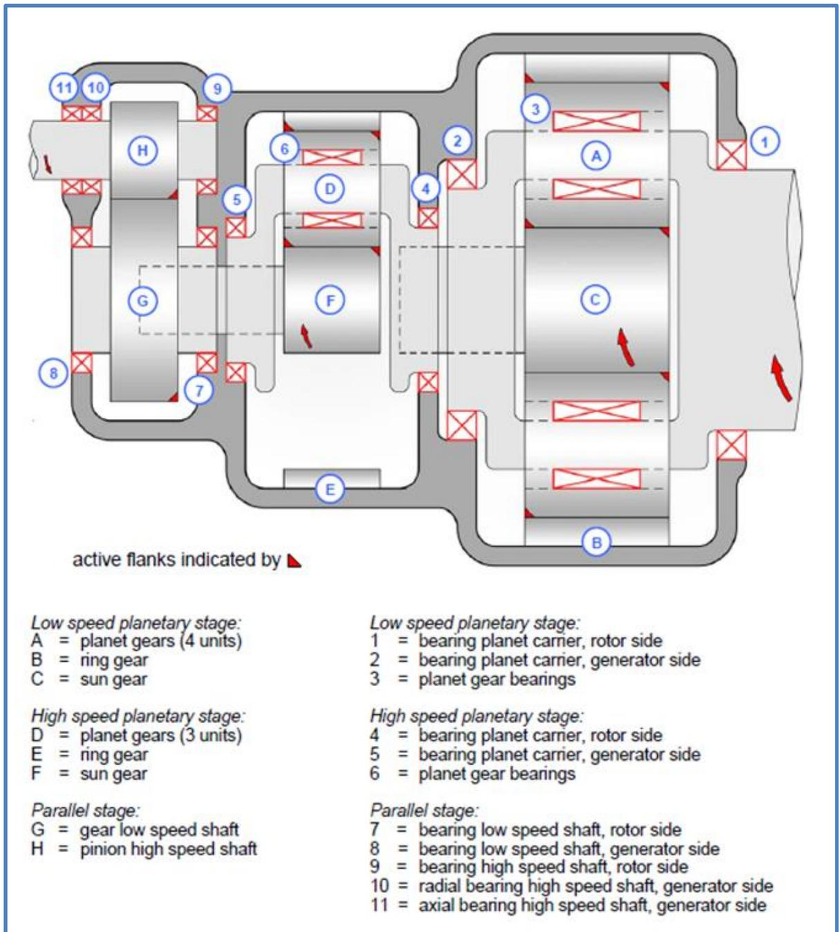
**Figure 3.4 Schematic diagram of a Planetary Gearbox of WT**
