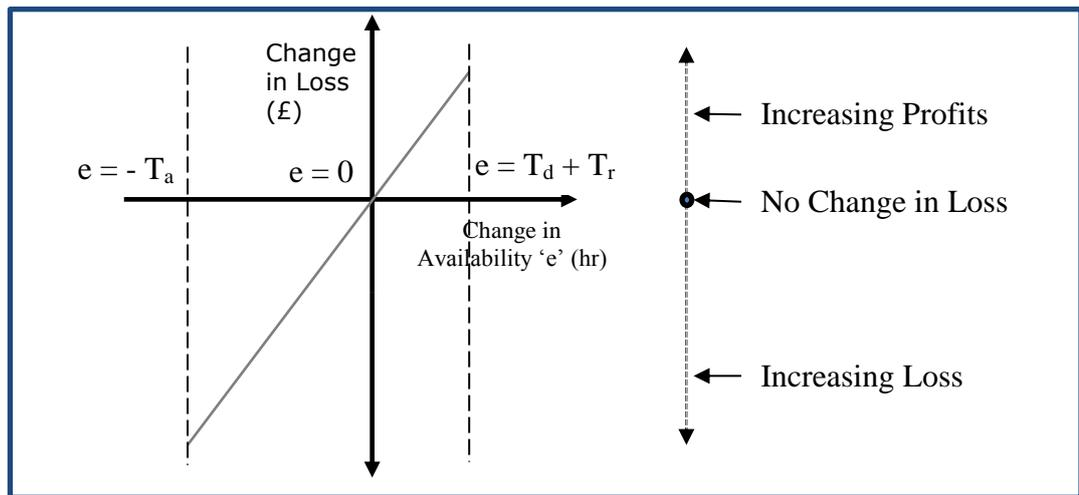
**Figure 5.2 Schematic shows variation in loss with changing availability**
