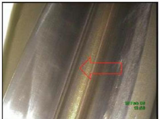
Picture 12: high speed planetary stage, planet gear, sun gear-active flank
