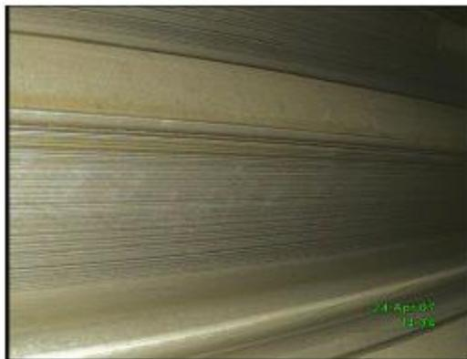
Picture 9: Ring gear, active flank
