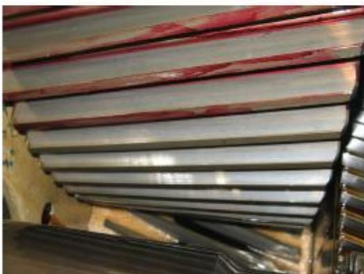
Picture 13: Gear first intermediate shaft, active flank
