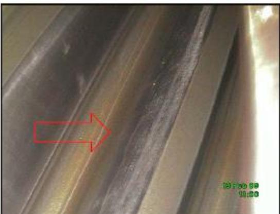
Picture 11: high speed planetary stage, planet gear, ring gear-active flank
