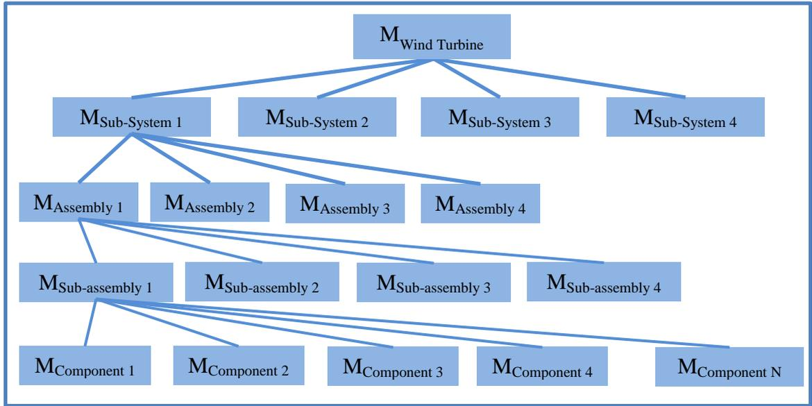
**Figure 2.7 Shows the hierarchical method for evaluating the reliability of a WT (M = Reliability)**
