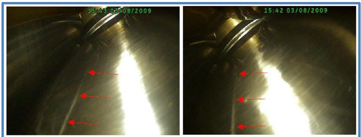
**Figure 3.7 (a) Shows the frequency spectrum depicting initiation of failure of radial bearing on intermediate shaft of gearbox on the generator side (b) visual pictures of the bearing showing development of surface fault (Source: Stork Technical Services, UK)**
