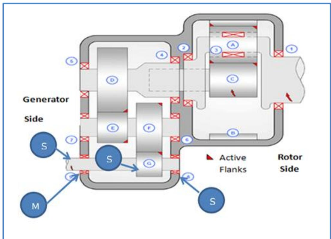
**Figure 5.5 Demonstration of MASTER Failure (M) and SLAVE Failure (S) concept (from Figure 3.4)**
