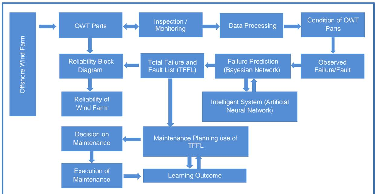
Figure 3.27 A modified scheme for planning CBM for OWT that uses intelligent processes to predict failures
