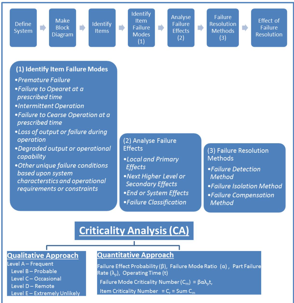
**Figure 2.9 Shows the standard process for doing FMEA and CA**
