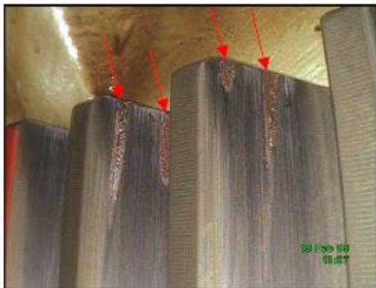
Picture 15: high speed planetary stage, ring gear, inactive flank
