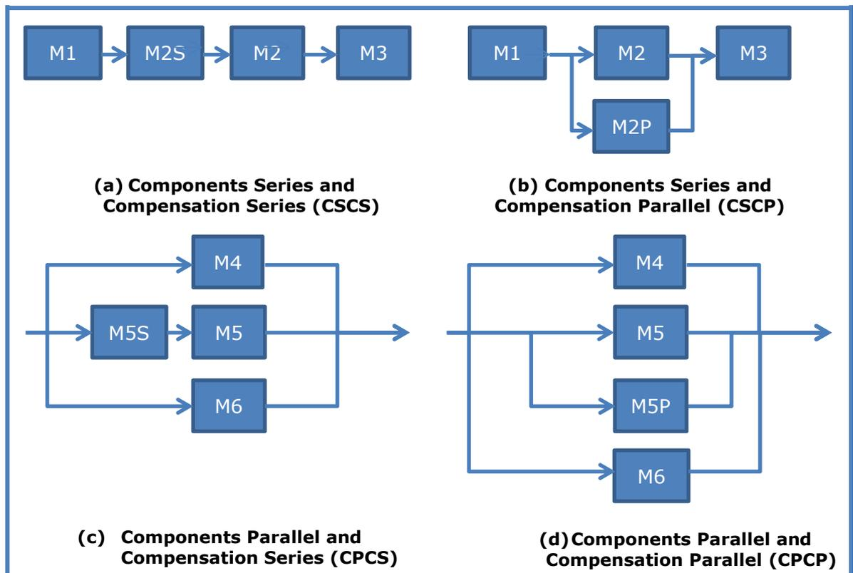
Figure 2.8 Shows different configurations for implementing compensatory provisions (M2S, M5S = series compensations, M2P, M5P = parallel compensations)
