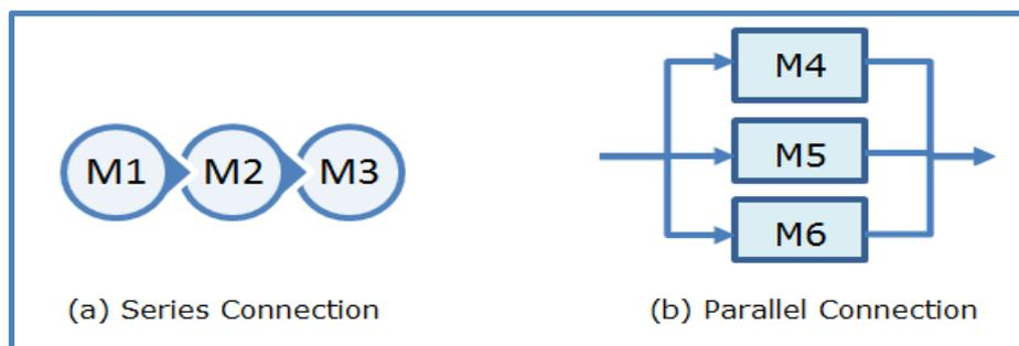
**Figure 2.6 Shows reliability calculation for (a) series and (b) parallel connected modules**
