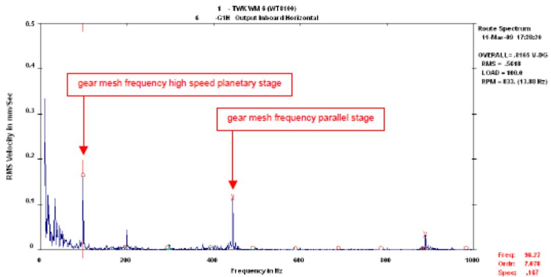
Figure 2: spectrum at high speed shaft, generator side, horizontal
