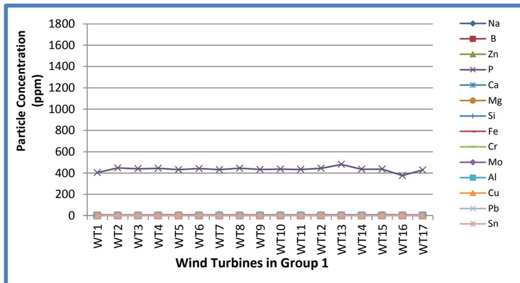
**Figure 3.8 Shows variation in particulate concentrations of lubricating oil in the Gearboxes for Group 1 WT**
