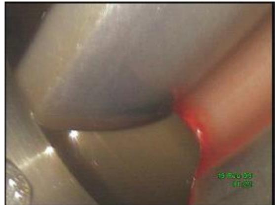
Picture 8: low speed planetary stage, sun gear, active flank
