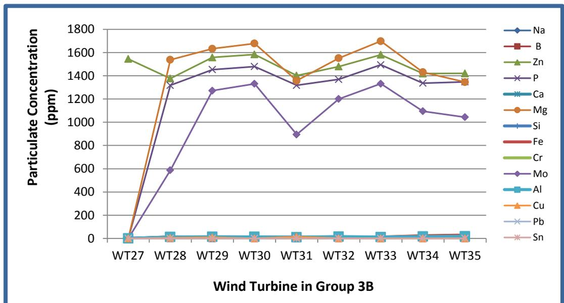
Figure 3.10 Shows variation in particulate concentrations of lubricating oil in the Gearboxes for Group 3B WT
