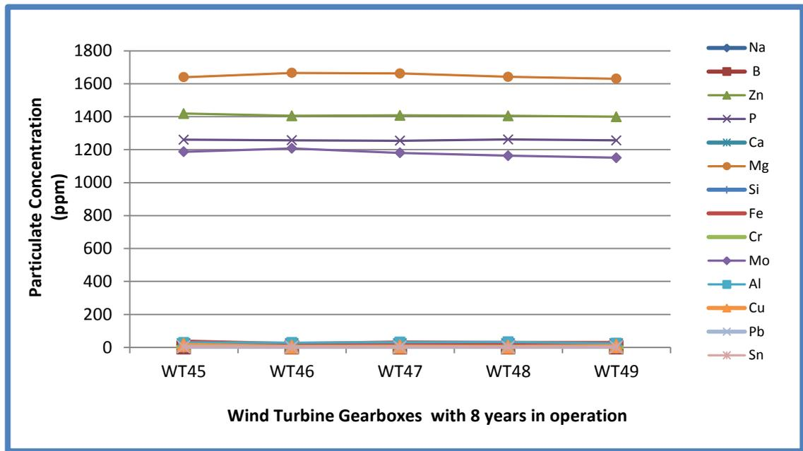
**Figure 3.11** Shows variation in particulate concentrations of lubricating oil in the Gearboxes for Group 6 WT
