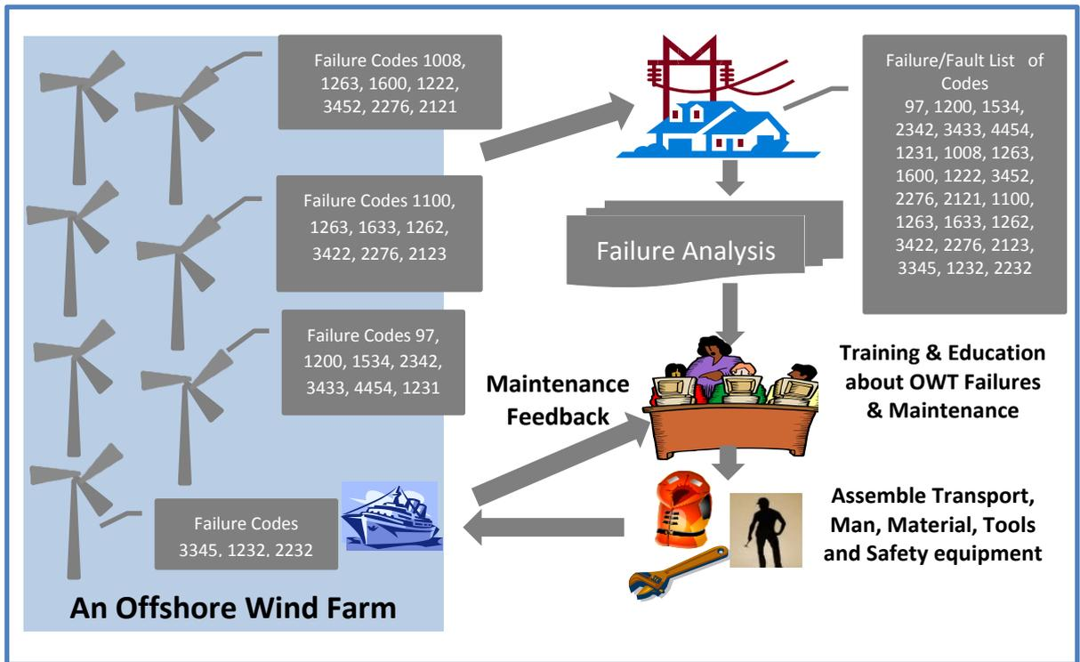
Figure 3.26 Scheme shows the processes involved in planning CBM for OWT
