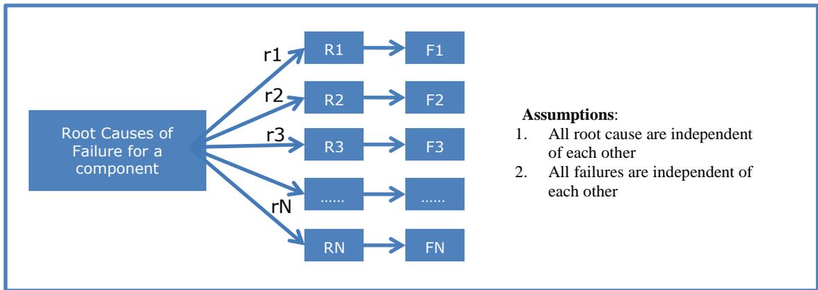
**Figure 3.18 Estimating the probability of a failure if root causes and failures are related by a 1:1 relationship**
