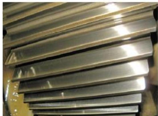
Picture 18: parallel stage, gear low speed shaft, active flank
