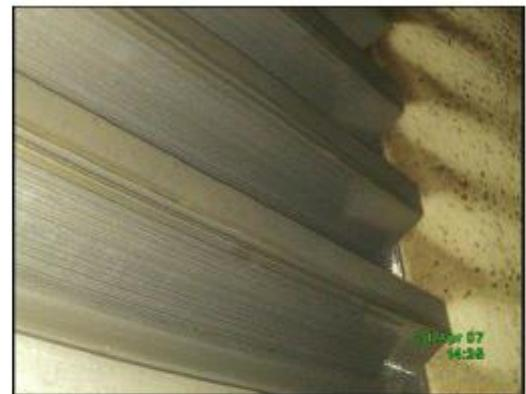
Picture 10: Ring gear, active flank
