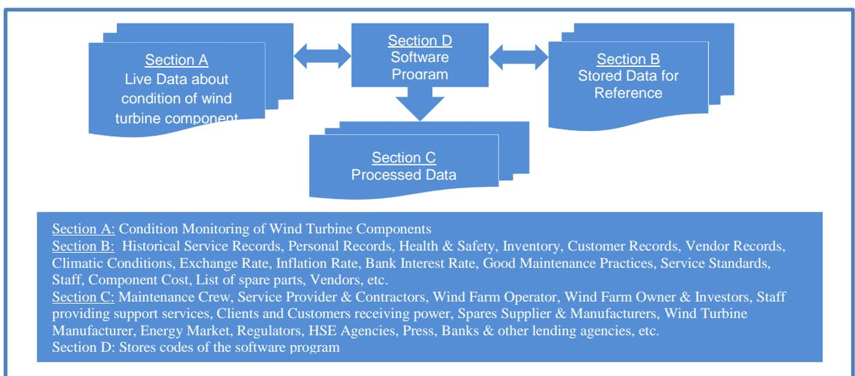
**Figure 4.4** Design of database section for OWT-MOT
