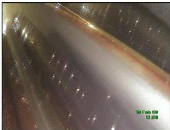
Picture 17: high speed planetary stage, sun gear, inactive flank
