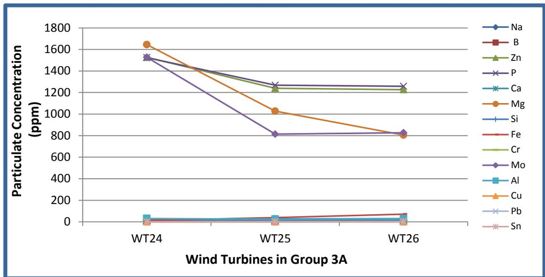
Figure 3.9 Shows variation in particulate concentrations of lubricating oil in the Gearboxes for Group 3A WT
