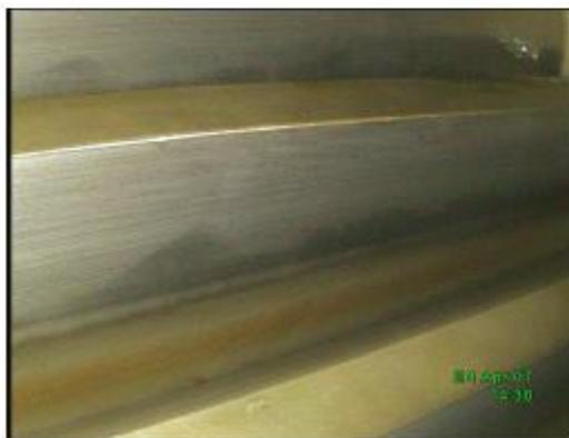
Picture 3: Planet wheel, ring gear-active flank
