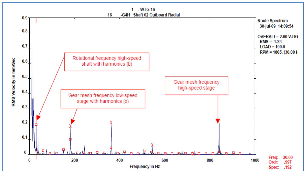
**Figure 3.5 Shows the frequency spectrum at intermediate shaft measured in the vertical direction on the rotor side**
