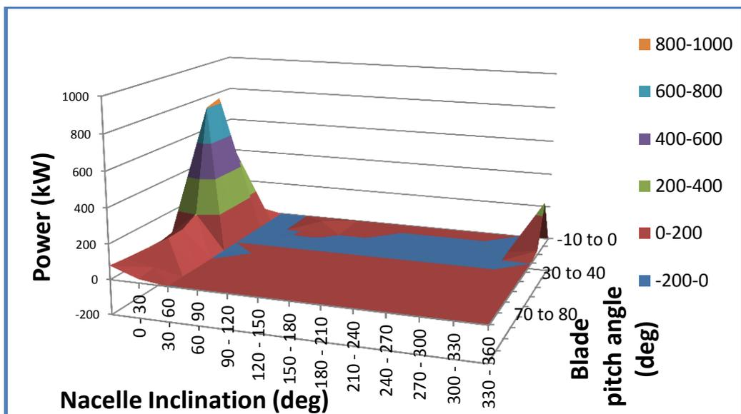
Figure 3.2 Shows the effect of nacelle and blade inclination (with incoming wind direction) on power generation capability of V52 WT
