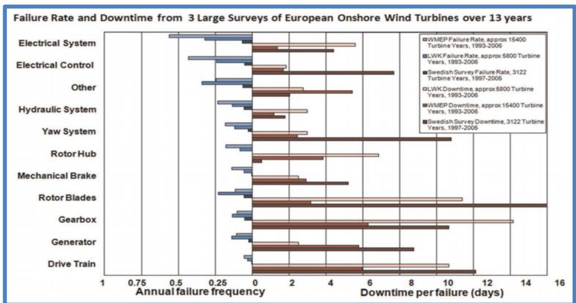
Figure 2.5 Plot of Failure/Wind Turbine/Year and downtime results for 25322 wind turbine year (Source: Chen, Matthews and Tavner, 2014)
