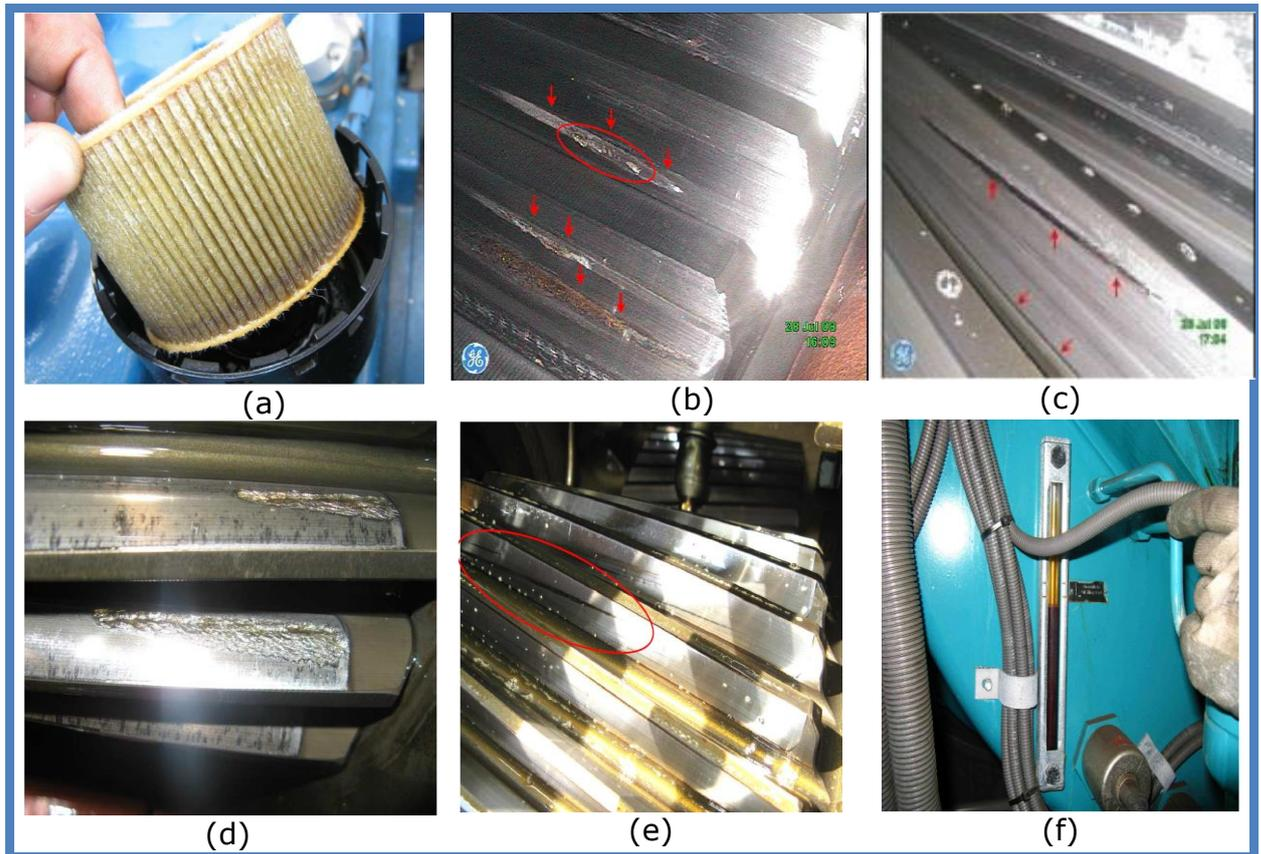
**Figure 3.13 Shows images obtained from visual inspection of wind turbine gearbox**
