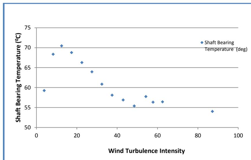
**Figure 3.3 Shows the effect of wind turbulence intensity on Shaft Bearing Temperature**
