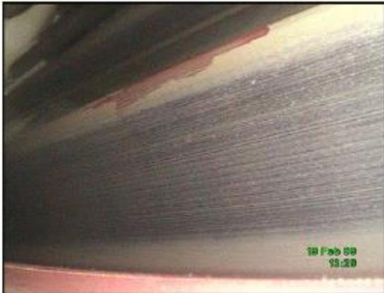
Picture 7: low speed planetary stage, ring gear, inactive flank
