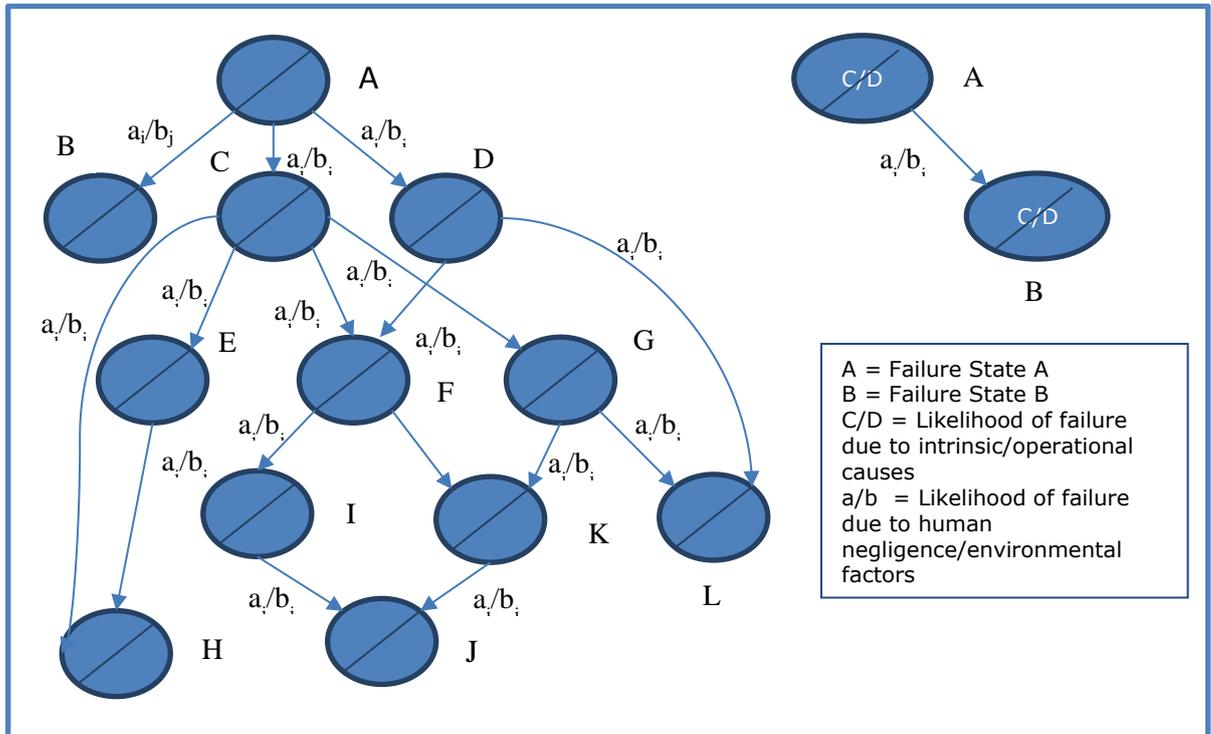
**Figure 3.20** Shows a schematic diagram of relationships between failures in OWT components
