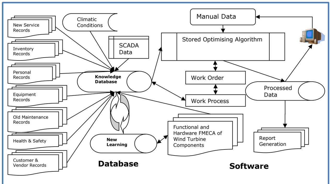
**Figure 4.1 Design framework for OWT-MOT software package**
