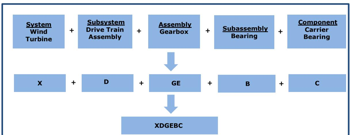
Figure 3.25 A hierarchical naming convention for wind turbine components
