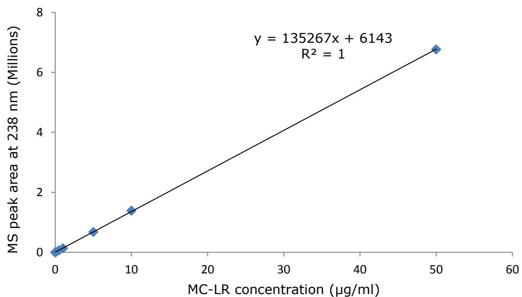
**Figure 2.1** MC-LR calibration curve obtained from HPLC-PDA analysis at 238 nm.
