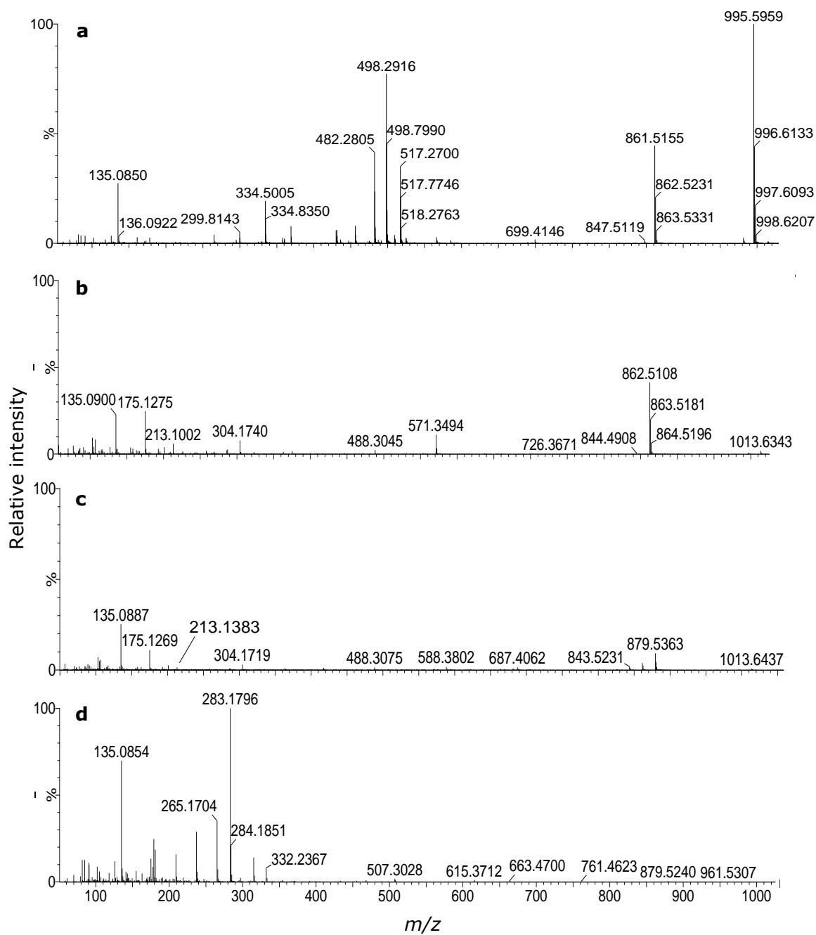
**Figure 4.5** Mass spectra at high collision energy (20 – 55 V) of (a) cyclic MC-LR, MC-LR degradation products (b) A and (c) B and mass spectrum at low collision energy (6 V) of MC-LR degradation product (d) C.
