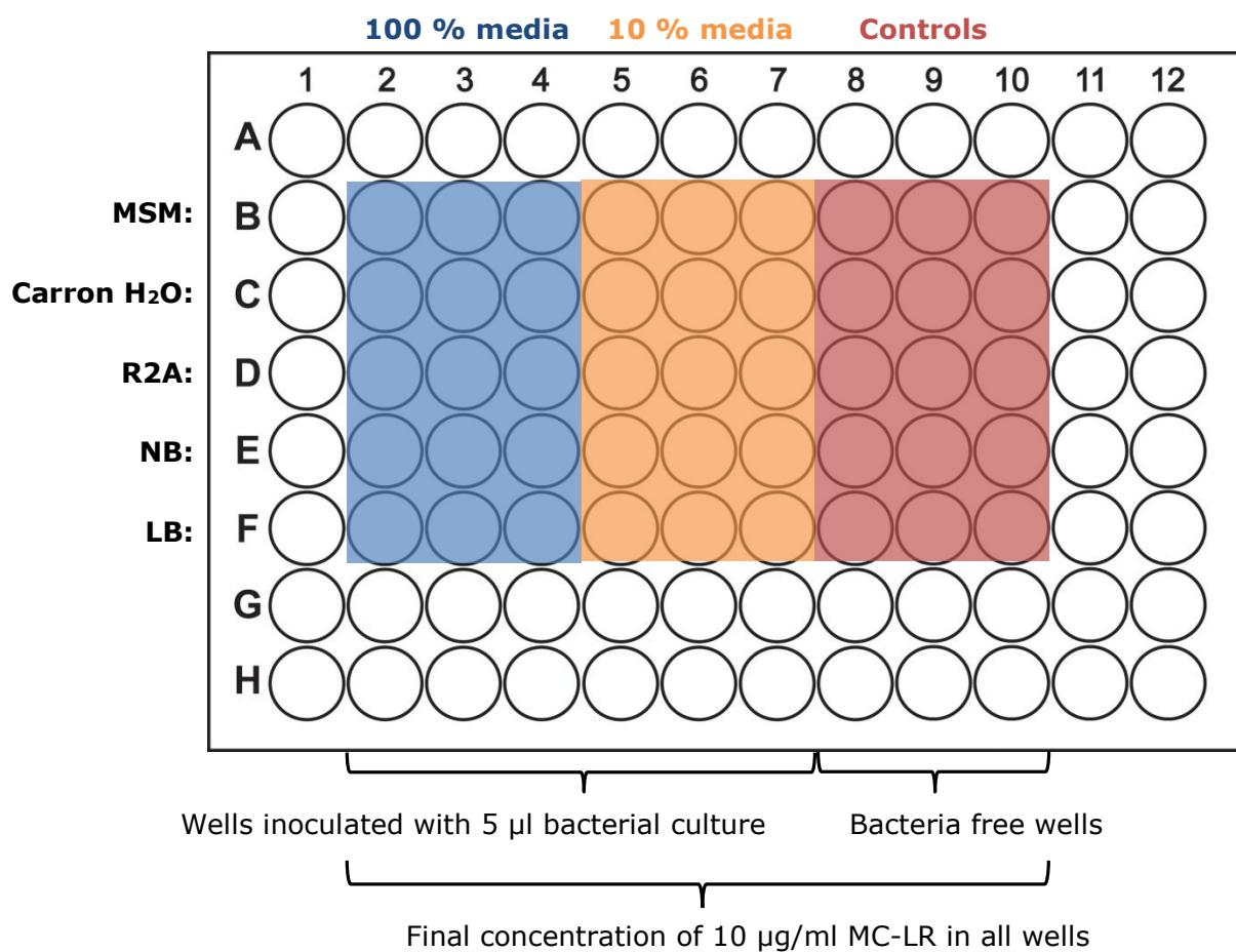
**Figure 4.1** Composition of the MC-LR degradation assay carried out in four 96 well plates each containing a different culture: (1) *P. toxinivorans* (2007), (2) *P. toxinivorans* (2015) (3) *Rhodococcus* sp. and (4) *Pseudomonas* sp..
