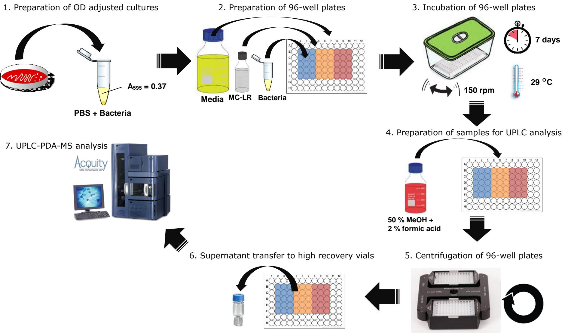
**Schemata 4.1** 96-well plate based method testing the effect of different growth media on bacterial MC-LR biodegradation.
