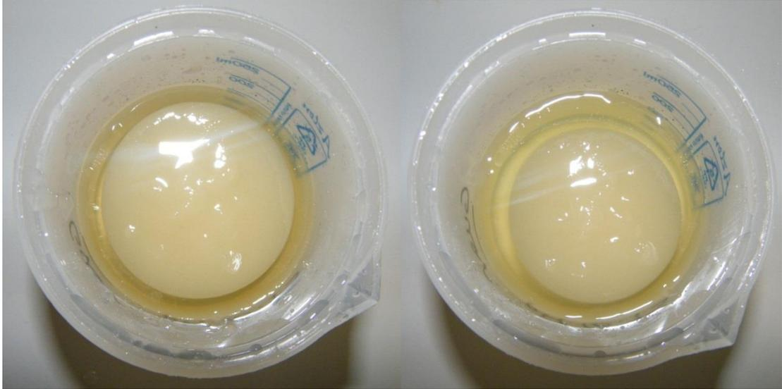
**Figure 3.13** *Guar gum in 2.0g/cm<sup>3</sup> Cs/K formate, initially hydrated at low pH before adding 13.1g/L carbonate to simulate std. brine conditions, photographed after 1 hour (left) and then overnight (right)*
