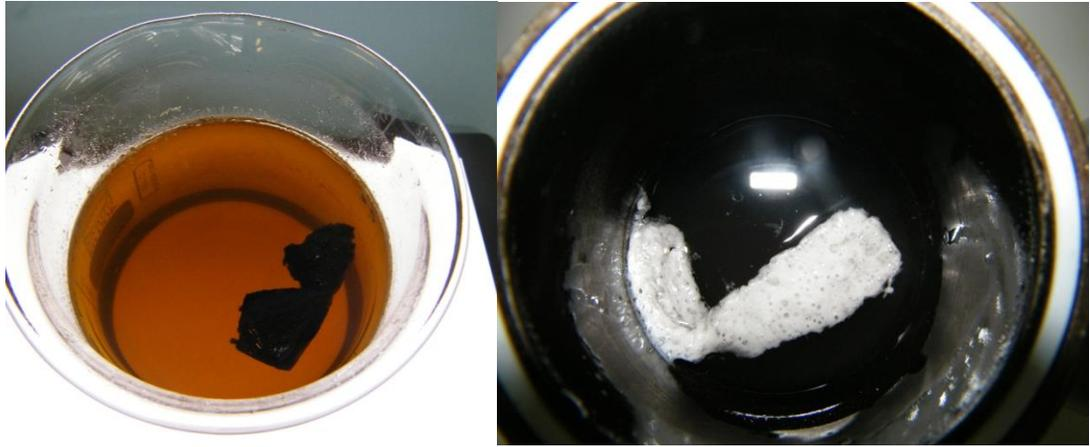
**Figure 3.34**  $2.0\text{g/cm}^3$  Cs/K formate and  $5.7\text{g/L}$  HE300 (left) and Driscal D (right) Polymer "ball" after dynamic ageing for 16 hours @  $185^\circ\text{C}$
