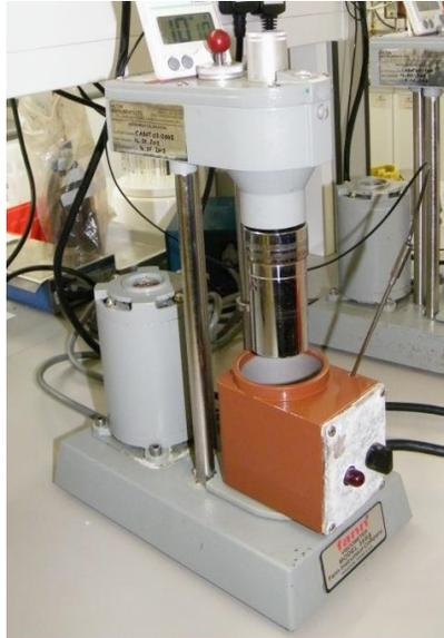
**Figure 2.3** *Fann35 Viscometer (Photograph taken in CSF Laboratory)*
