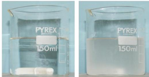
Figure 1 1.85 g/cm<sup>3</sup> cesium formate with 5% PEG 400 at room temperature (left) and heated to 60°C (right)
