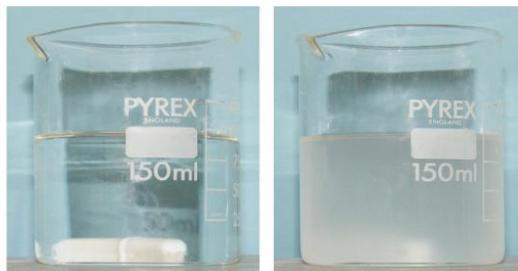
Figure 1 1.85 g/cm³ cesium formate with 5% PEG 400 at room temperature (left) and heated to 60°C (right)
