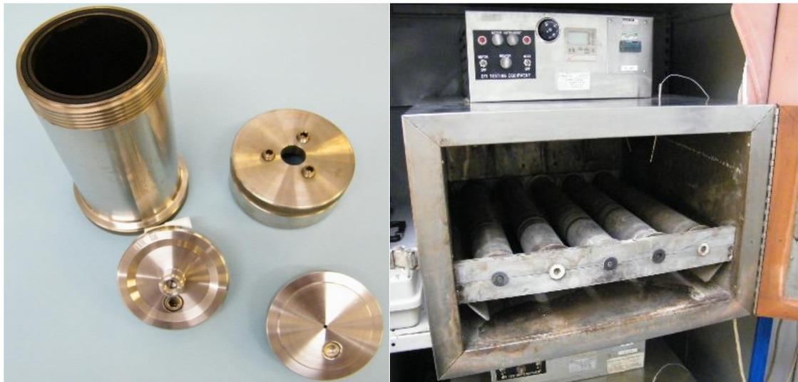
**Figure 2.4** *Temperature resistant cell for dynamic ageing (left) and inside a hot-rolling oven (right), CSF Laboratory, Aberdeen*
