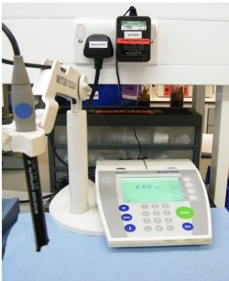
**Figure 2.1** *Mettler Toledo glass electrode pH meter (photograph taken in CSF Laboratory)*
