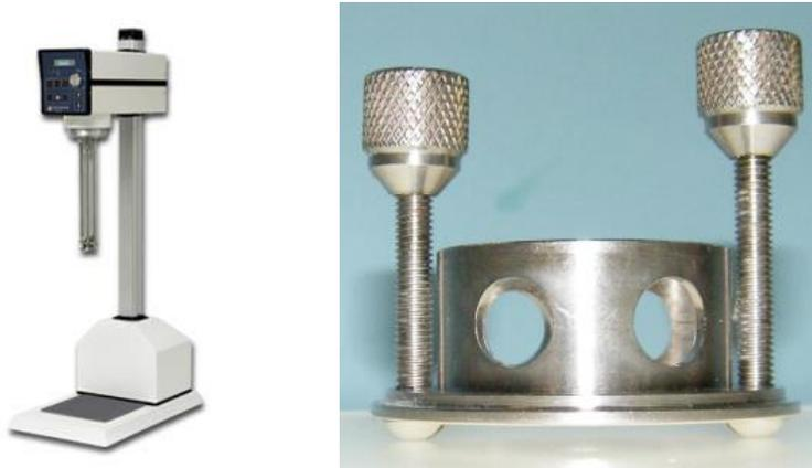
**Figure 2.2** *Silverson mixer (left) and shearing head (right) for water-based drilling fluids*
