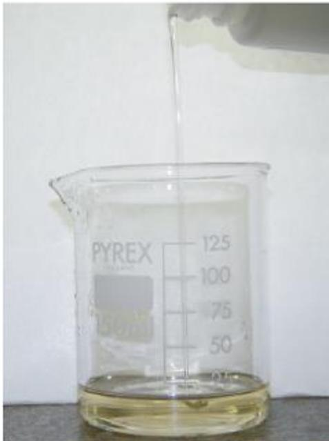
Figure 1. Clear solution of cesium formate in MEG – density 2.22 g/cm<sup>3</sup>.
