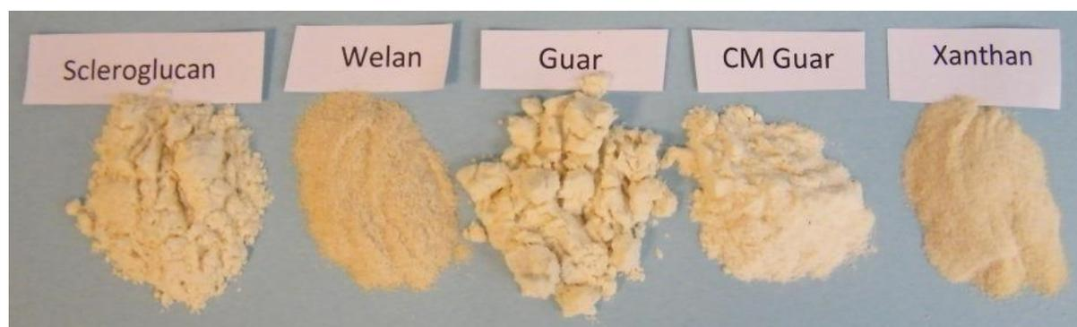
**Figure 3.3** Dry polymeric materials before addition to solution (photograph taken in CSF Laboratory)
