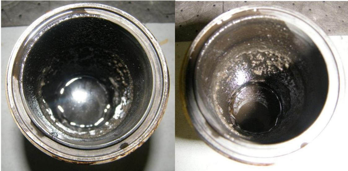
**Figure 3.43** *Mineralized xanthan gum in hot-rolling cell after dynamic ageing for 64 hours @ 250°C (Photograph taken in CSF Laboratory)*
