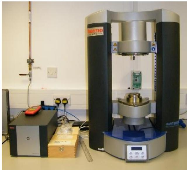
**Figure 2.6** *Haake MARS III HPHT Rheometer (Photograph taken in CSF Laboratory)*
