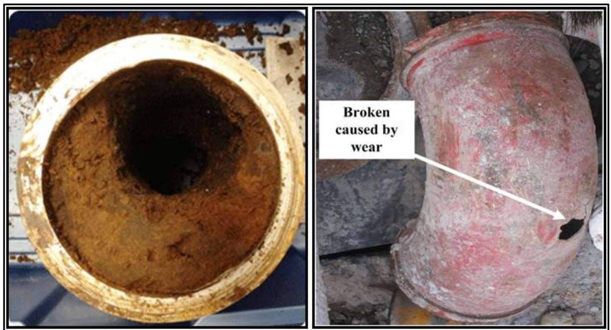
Figure 1.2: Images of plugged pipe by sand and damage caused by wear (Andrzej and Susan 2001)
