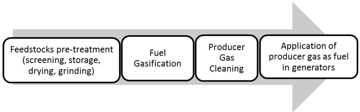
Figure 3.2: Gasification Processes for Electricity Generation (Adopted from: Demirbas 2009; Bocci et al. 2014; IRENA 2012)
