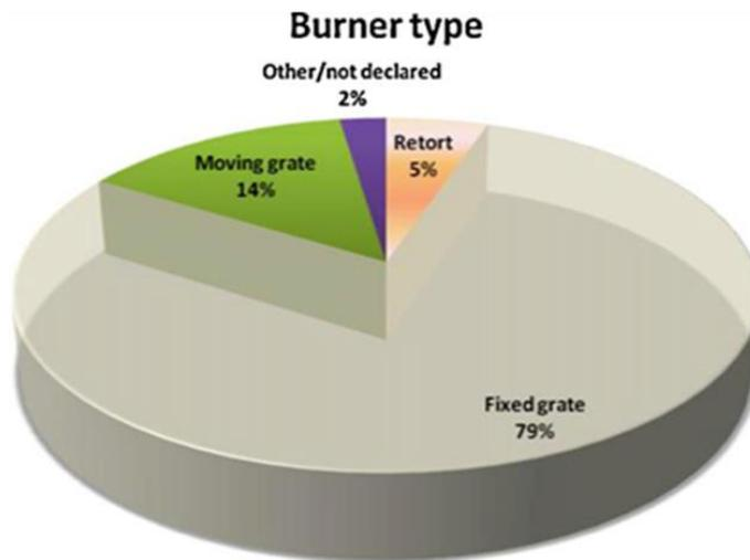
Figure 3.4: Burners types as applied in the Industry (Miguez et al. 2012)
