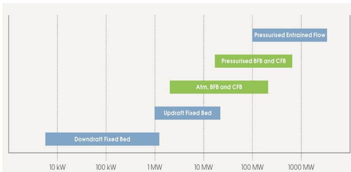
Figure 3.1: Gasifier reactor capacities by forms (IRENA 2012)
