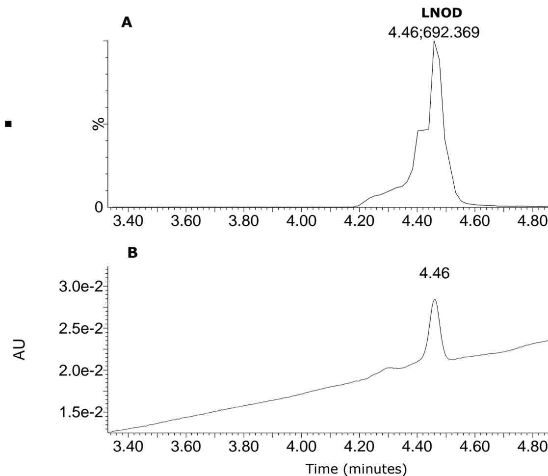
**Figure 3. 14** LNOD ( $0.5 \mu\text{g mL}^{-1}$ ) in 50% aqueous MeOH. UPLC-QToF-MS chromatogram extracted at  $m/z$  692 (A) and UPLC-PDA chromatogram extracted at 238 nm (B).
