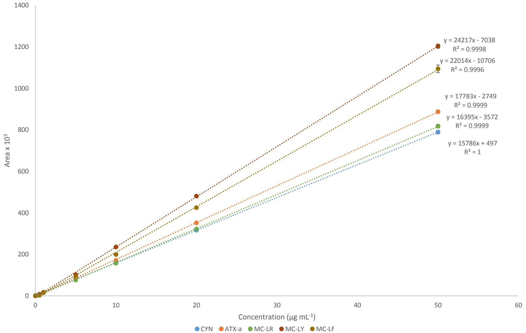
**Figure 2. 22** Cyanotoxin calibration obtained after HPLC-PDA analysis monitored at 262 nm (CYN), 228 nm (ATX), and 238 nm (MCs).
