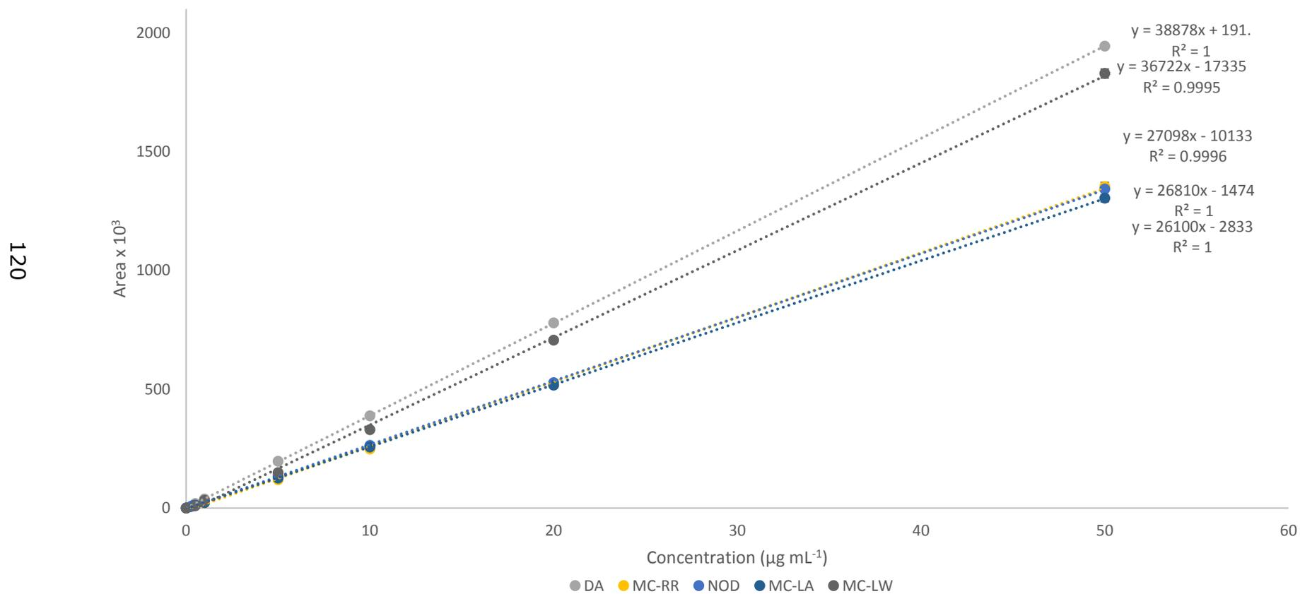
**Figure 2. 21** Cyanotoxin calibration obtained after HPLC-PDA analysis monitored at 238 nm.
