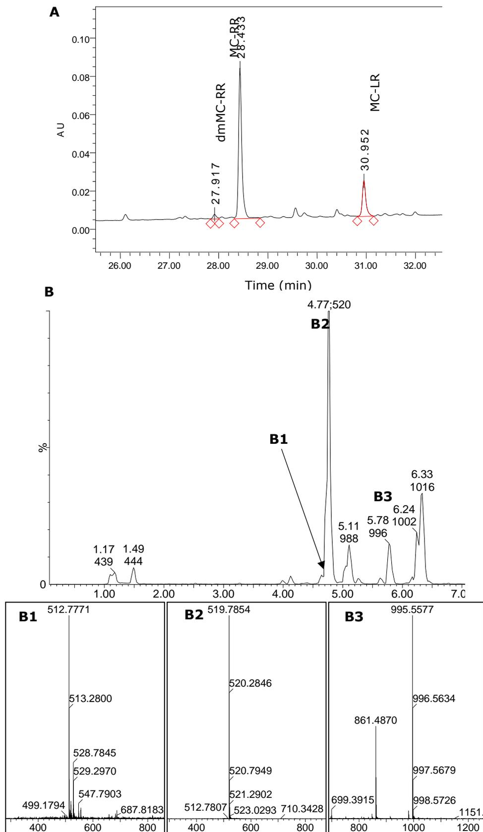
**Figure 2. 26** HPLC-PDA chromatogram monitored at 238 nm (A). TIC UPLC-QToF-MS chromatogram (B) and Mass spectrum (base peak) of dmMC-RR (B1), MC-RR (B2), and MC-LR (B3) detected in *M. botrys* NIVA CYA 161/1.
