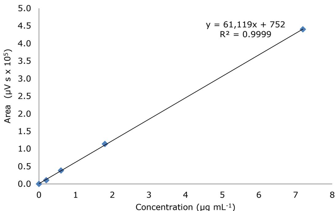
**Figure 2. 6** Calibration of DA using water as the sample solvent obtained by HPLC-PDA (240 nm)
