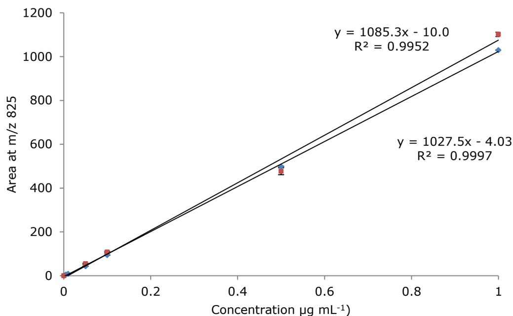
**Figure 3. 11** Calibration of NOD (0.001-1 µg mL<sup>-1</sup>) in 50% aqueous MeOH (blue) and negative mussel extracts (red) utilising UPLC-QToF-MS at m/z 825. Error bars represent standard deviation (n=3).
