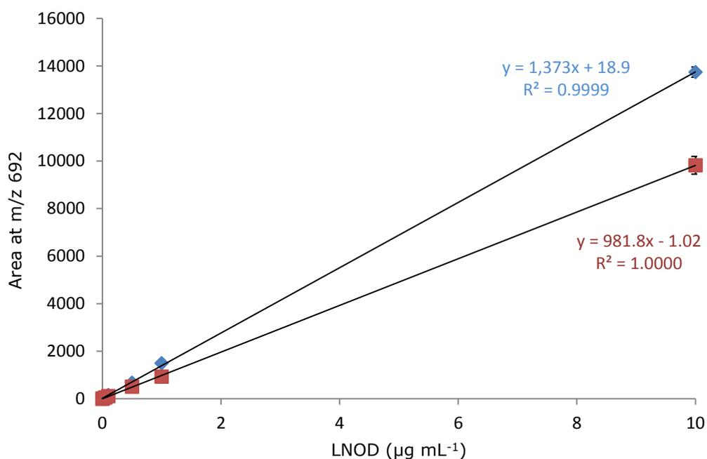
**Figure 3. 13** Calibration of LNOD in 50% aqueous MeOH (blue) and negative mussel extracts (red) utilising UPLC-QToF-MS at m/z 692. Error bars represent standard deviation ( $n=3$ ).
