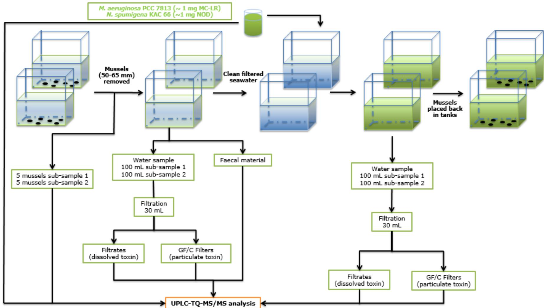
**Figure 5. 4** Schematic illustration of sampling procedure of exposure tank. Control containers were treated identically except for shellfish diet being added to each tank rather than cyanobacteria.
