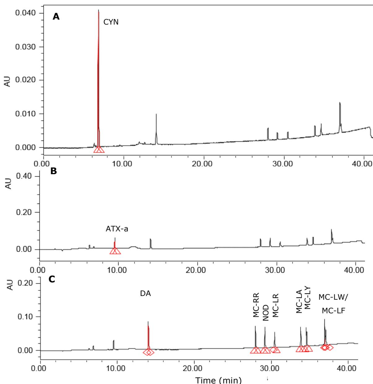
**Figure 2. 9** Separation of DA and nine cyanotoxins utilising HPLC-PDA gradient separation (Table 2. 12). CYN monitored at 262 nm (A) ATX-a monitored at 228 nm (B) DA, MCs, and NOD monitored at 238 nm (C)
