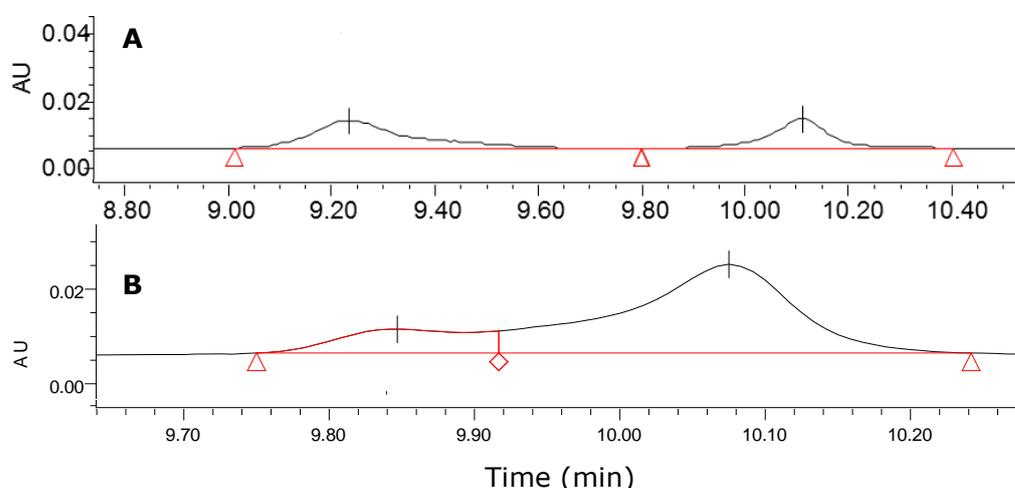
**Figure 2. 11** ATX-a ( $10 \mu\text{g mL}^{-1}$ ) after re-suspension in MeCN (A) and 50% aqueous MeCN (B) monitored at 228 nm.
