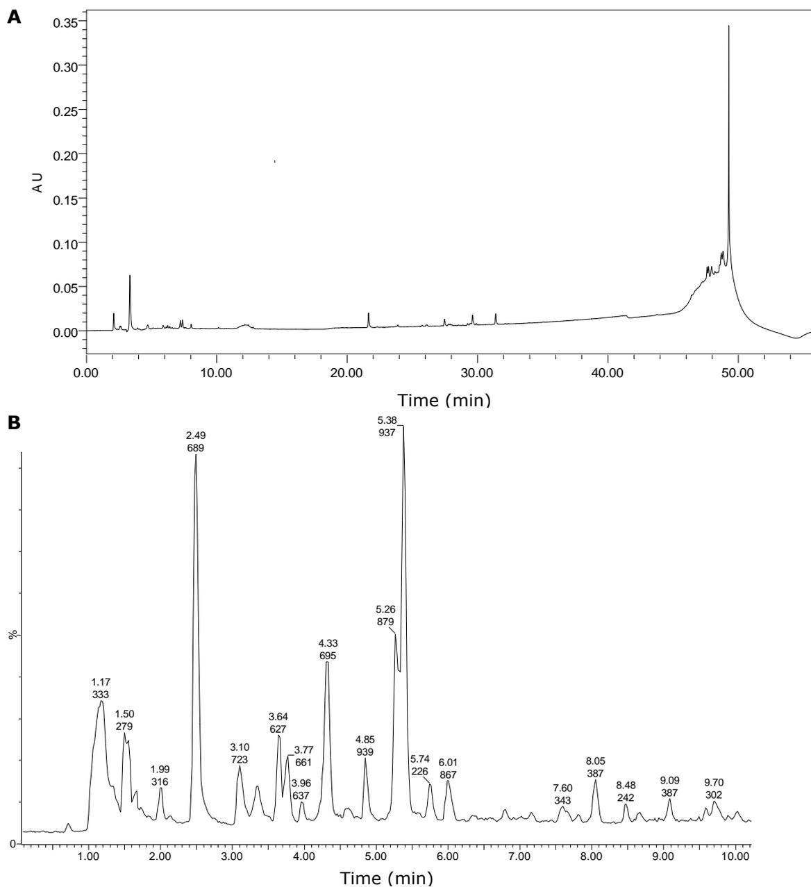
**Figure 2. 29** HPLC-PDA chromatogram monitored at 238 nm (A) TIC UPLC-QToF-MS chromatogram of *M. aeruginosa* CCAP 1450/3 (B).
