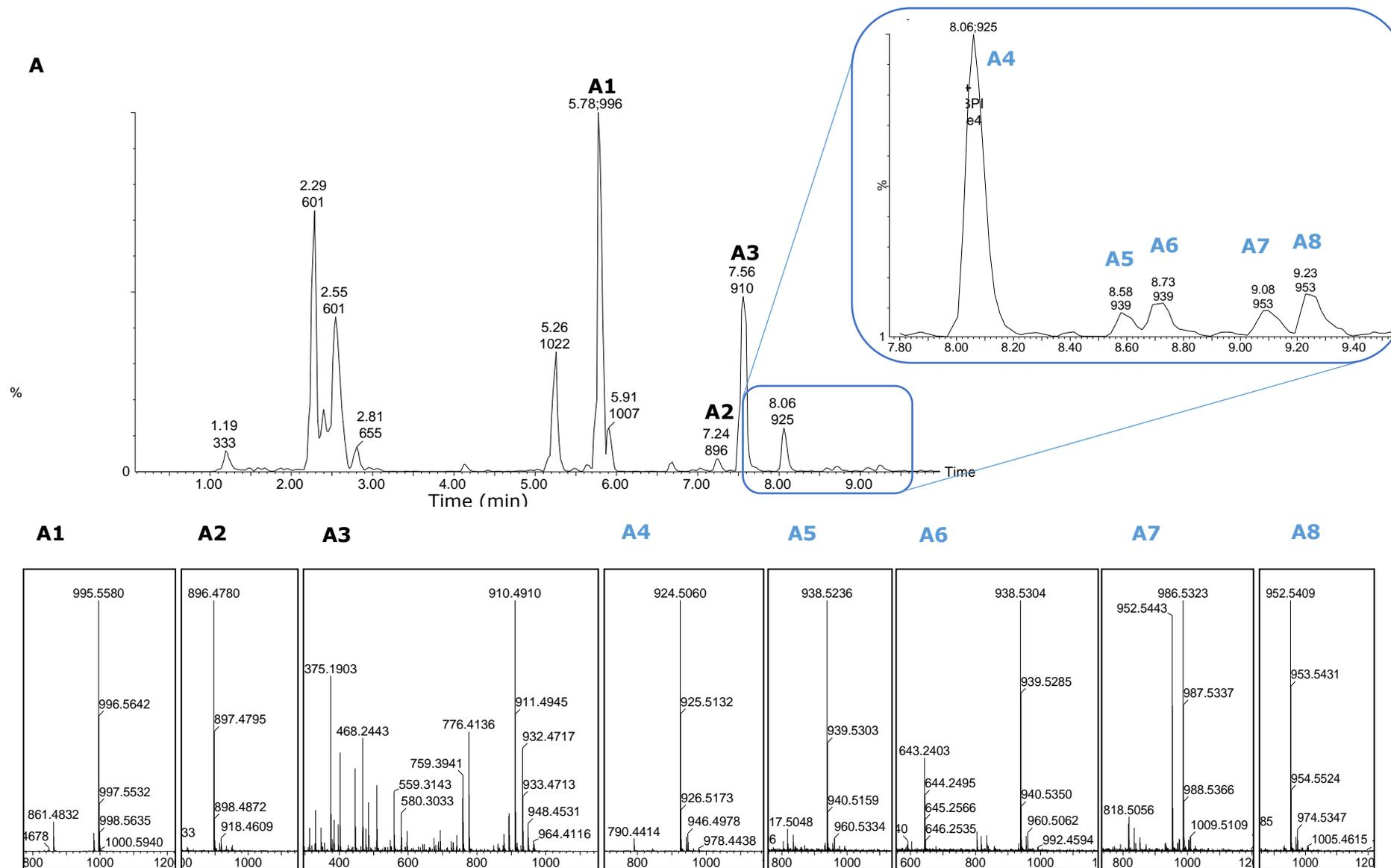
**Figure 2.** 28 TIC UPLC-QToF-MS chromatogram (A) and mass spectrum (base peaks) of MC-LR (A1), dmMC-LA (A2), MC-LA (A3), [D-Glu(OCH<sub>3</sub>)<sup>6</sup>, D-Asp<sup>3</sup>] MC-L(Aba) (A4), dmMC-LL (A5, A6), co-eluting MC-LL and MC-LF (A7), and MC-LL (A8) detected in *M. aeruginosa* UTEX B2666.
