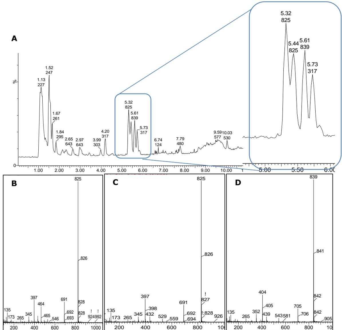
**Figure 2. 20** TIC UPLC-QToF-MS chromatogram of *N. sphaerocarpa* PCC 7804 (A) and mass spectrum (base peak) of peaks at  $t_r$  5.32 min (B), 5.44 min (C), and 5.61 min (D)
