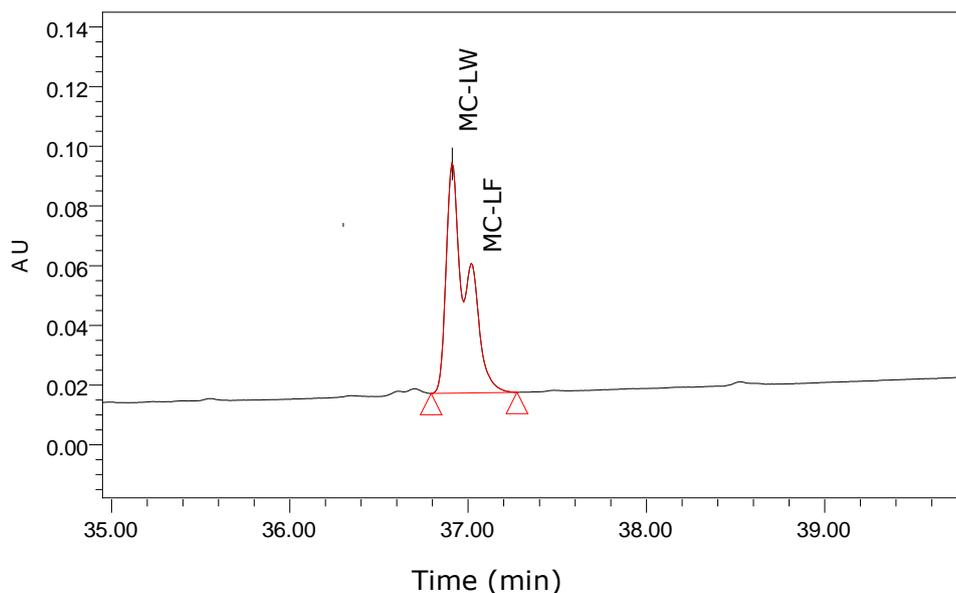
**Figure 2. 10** HPLC-PDA chromatogram of incomplete MC-LW and MC-LF ( $10 \mu\text{g mL}^{-1}$ ) monitored at 238 nm utilising the optimised gradient for the separation of DA and nine cyanotoxins
