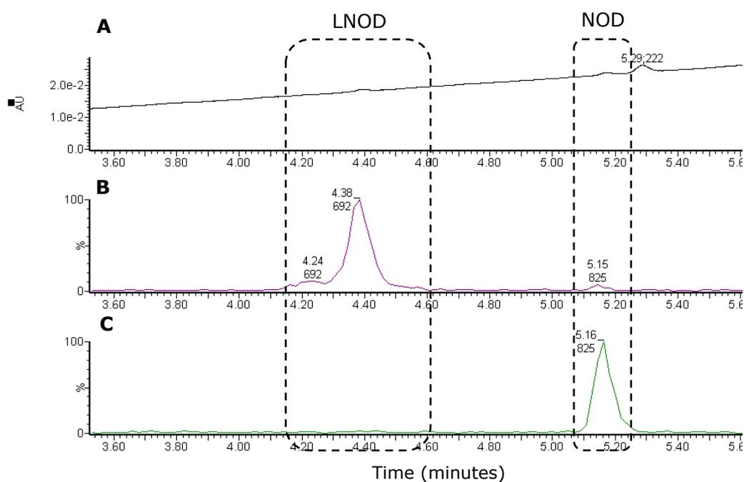
**Figure 3. 18** Intracellular NODs detected in water sample following the exposure of *M. edulis* to *N. spumigena* KAC66. Samples were analysed utilising UPLC-PDA (238 nm; A) and UPLC-QToF-MS recorded at m/z 692 (LNOD; B) and m/z 825 (NOD; C)
