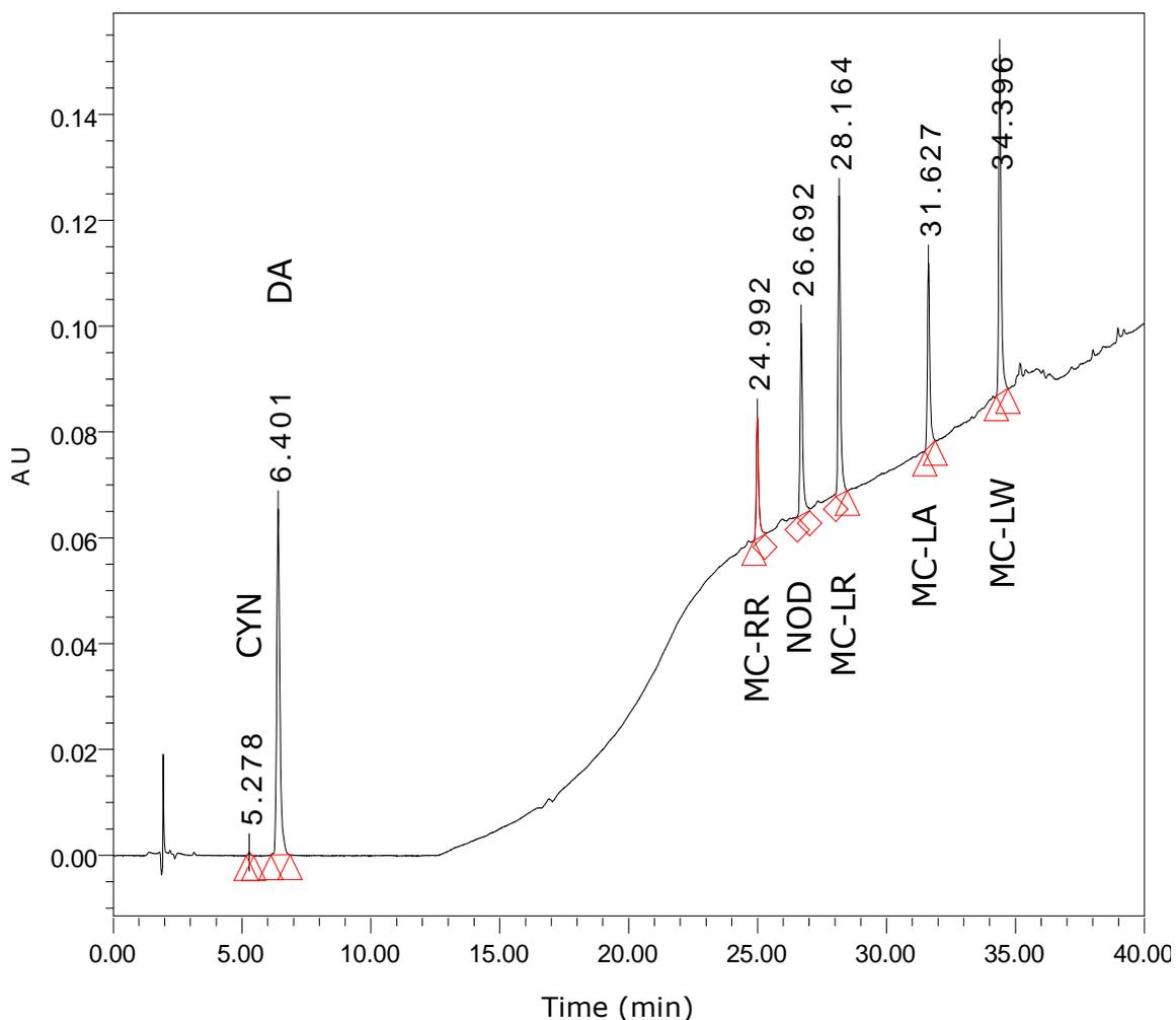
**Figure 2. 7** HPLC-PDA analysis of DA and six cyanotoxins (monitored at 240 nm) using initial isocratic 10 min DA method (Cefas) followed by a 30 min gradient from 32.5% to 100% MeOH.
