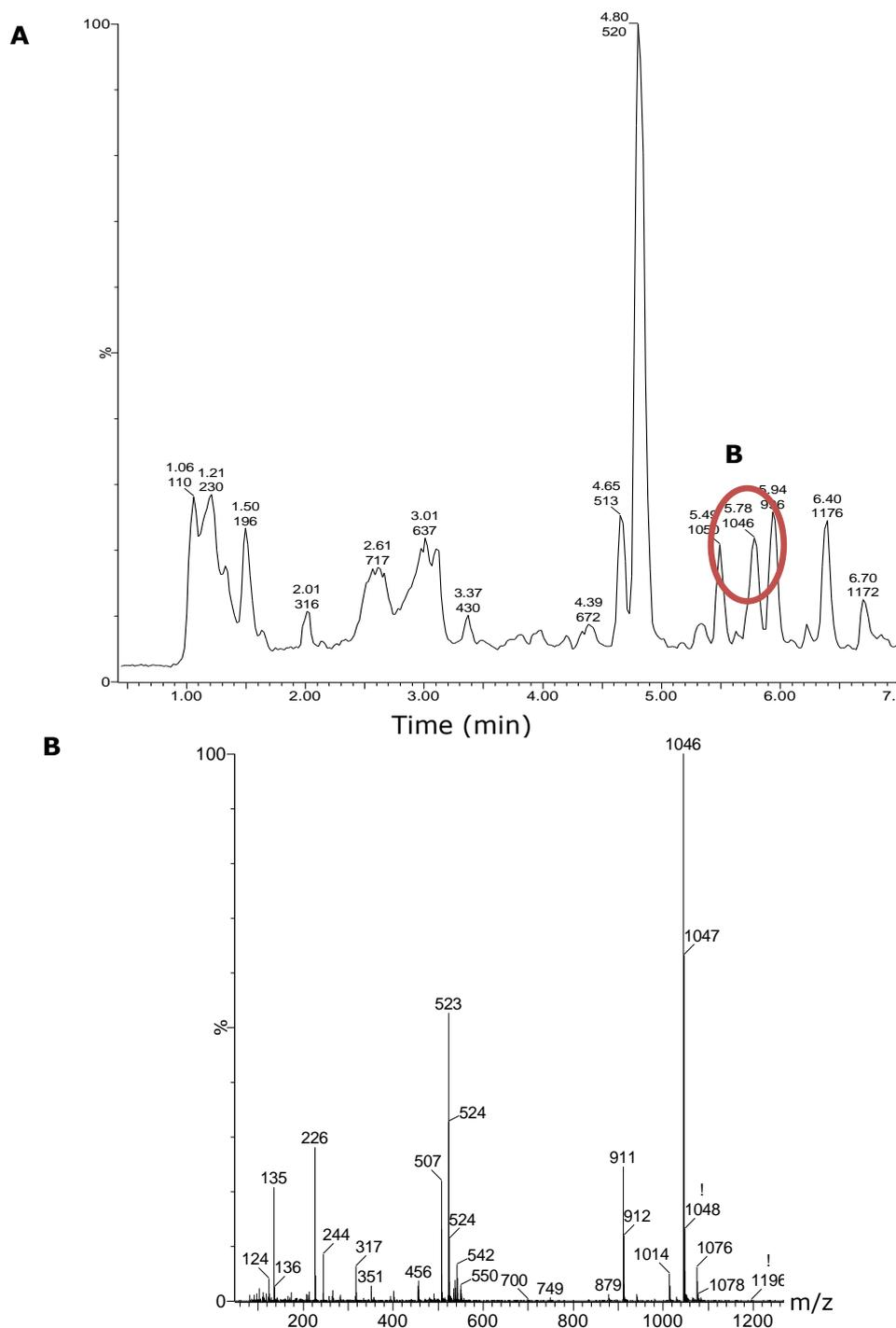
**Figure 2.17** TIC UPLC-QToF-MS chromatogram of *M. aeruginosa* NIES 1099 (A). Mass spectrum corresponding to MC-YR extracted at  $t_R = 5.78$  min (B).
