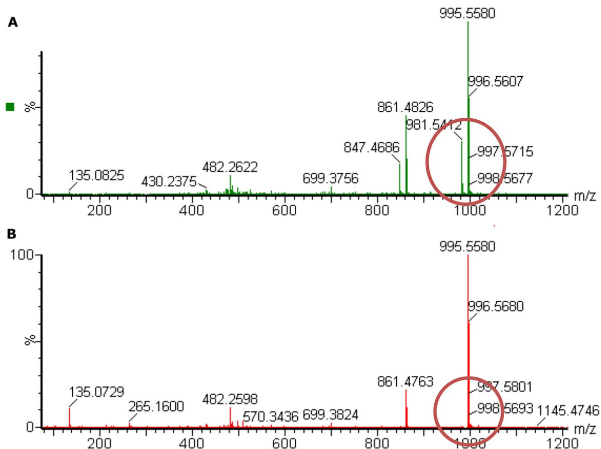
**Figure 2. 15** Mass spectrum of MC-LR detected in *M. aeruginosa* NIES 1071 (A) and a 10 µg mL<sup>-1</sup> standard (B) illustrating the different intensities of the 981 fragment indicating the presence of dmMC-LR in the cyanobacterial extract.
