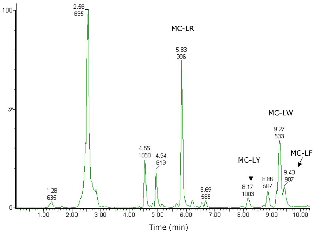
**Figure 4. 3** Example UPLC-QToF-MS base peak intensity chromatogram of *M. aeruginosa* PCC 7813 extracts.
