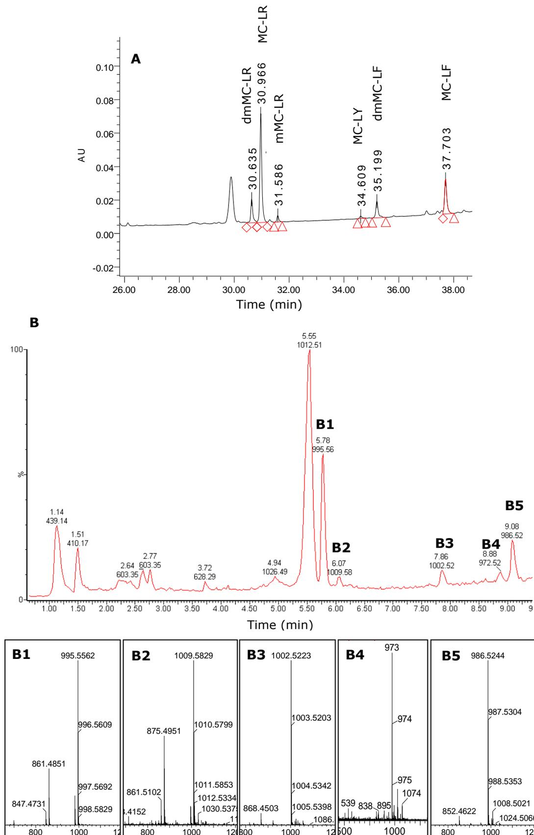
**Figure 2. 30** HPLC-PDA chromatogram monitored at 238 nm A). TIC UPLC-QTOF-MS chromatogram (B) and mass spectrum (base peak) of MC-LR (B1), mMC-LR (B2), MC-LY (B3), dmMC-LF (B4) and MC-LF (B5) detected in *M. aeruginosa* CCAP 1450/10 extracts.
