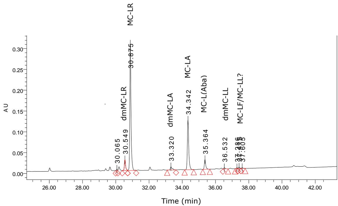
**Figure 2. 27** HPLC-PDA chromatogram of *M. aeruginosa* UTEX B2666 monitored at 238 nm. The presence of demethylated MCs and MC-L(Aba) was tentatively suggested based on variants reported in the literature and shifts in  $t_R$  observed.
