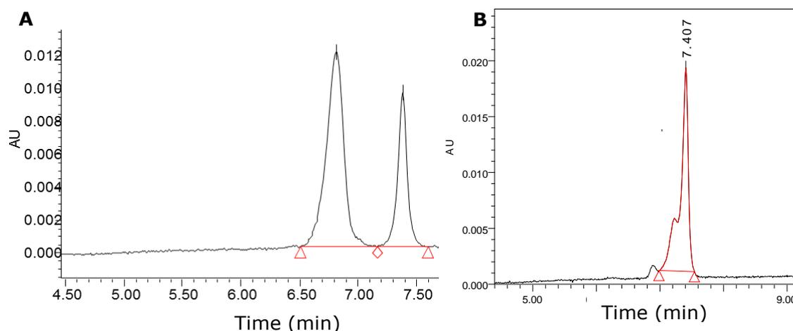
**Figure 2. 12** CYN ( $10 \mu\text{g mL}^{-1}$ ) after re-suspension in 50 % aqueous MeCN (A) and 100% MeOH (B) monitored at 262 nm.
