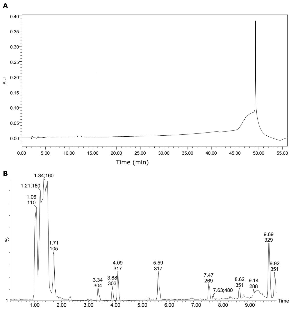
**Figure 2. 40** HPLC-PDA chromatogram monitored at 238 nm (A) TIC UPLC-QToF-MS chromatogram of *P. autumnale* CCAP 1462/6 (B).
