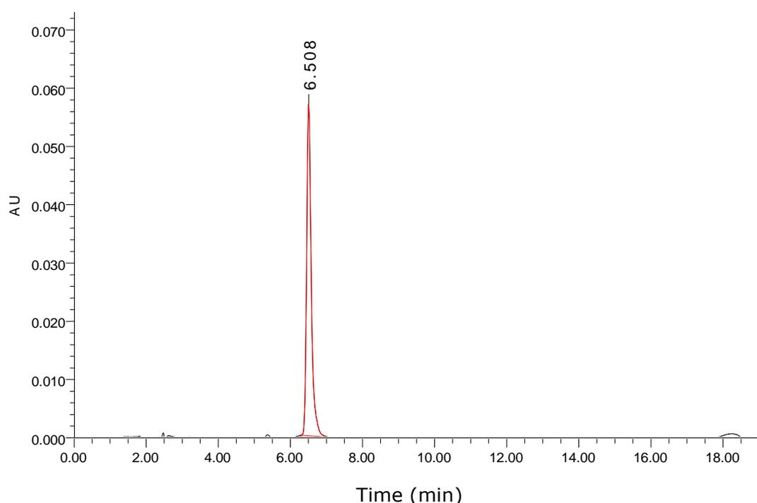
**Figure 2. 4** HPLC-PDA chromatogram of DA ( $10 \mu\text{g mL}^{-1}$ ) in 5 % aqueous MeCN monitored at 240 nm ( $V_{\text{inj}}= 10 \mu\text{L}$ ).
