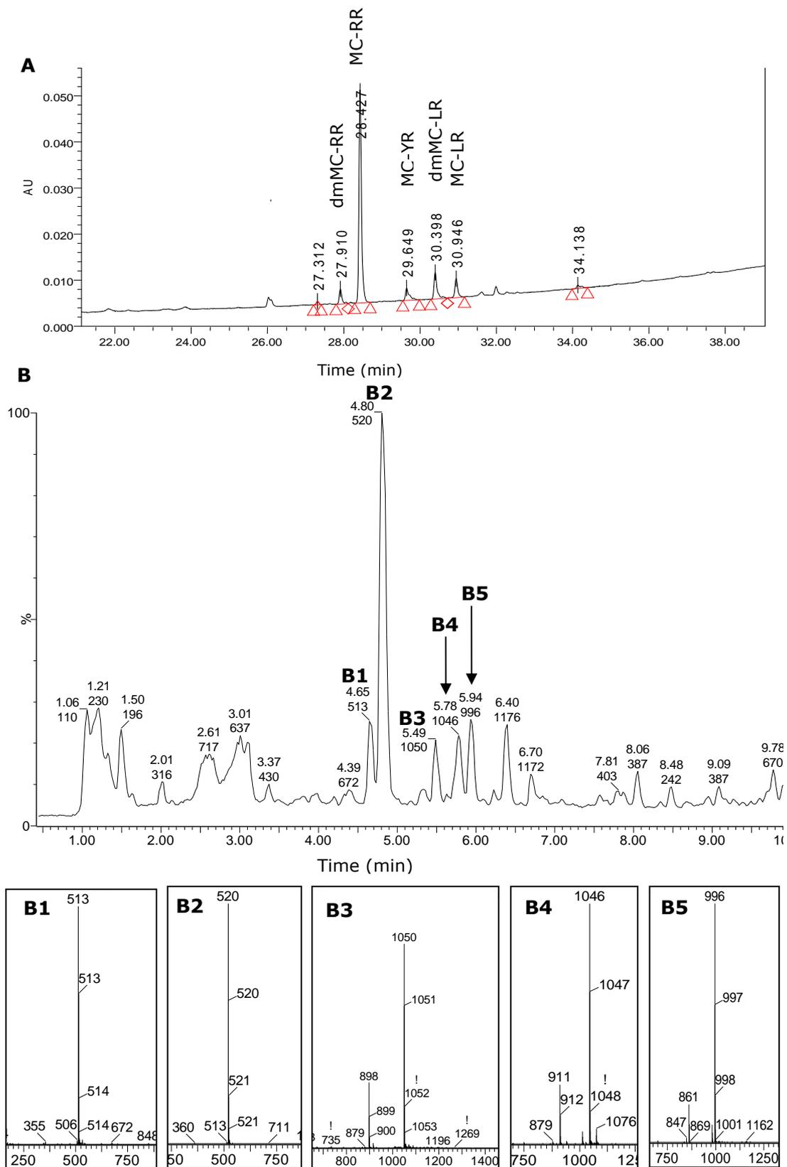
**Figure 2. 32** HPLC-PDA chromatogram monitored at 238 nm (A) TIC UPLC-QToF-MS chromatogram (B) and mass spectra (base peak) of dmMC-RR (B1), MC-RR (B2), MC-YR (B3), and MC-LR (B4) detected in *M. aeruginosa* NIES 1099.
