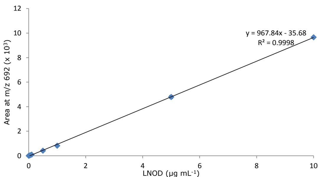
**Figure 3. 7** Calibration of LNOD in 80 % aqueous MeOH utilising UPLC-QToF-MS at m/z 692. Error bars represent standard deviation (n=3).
