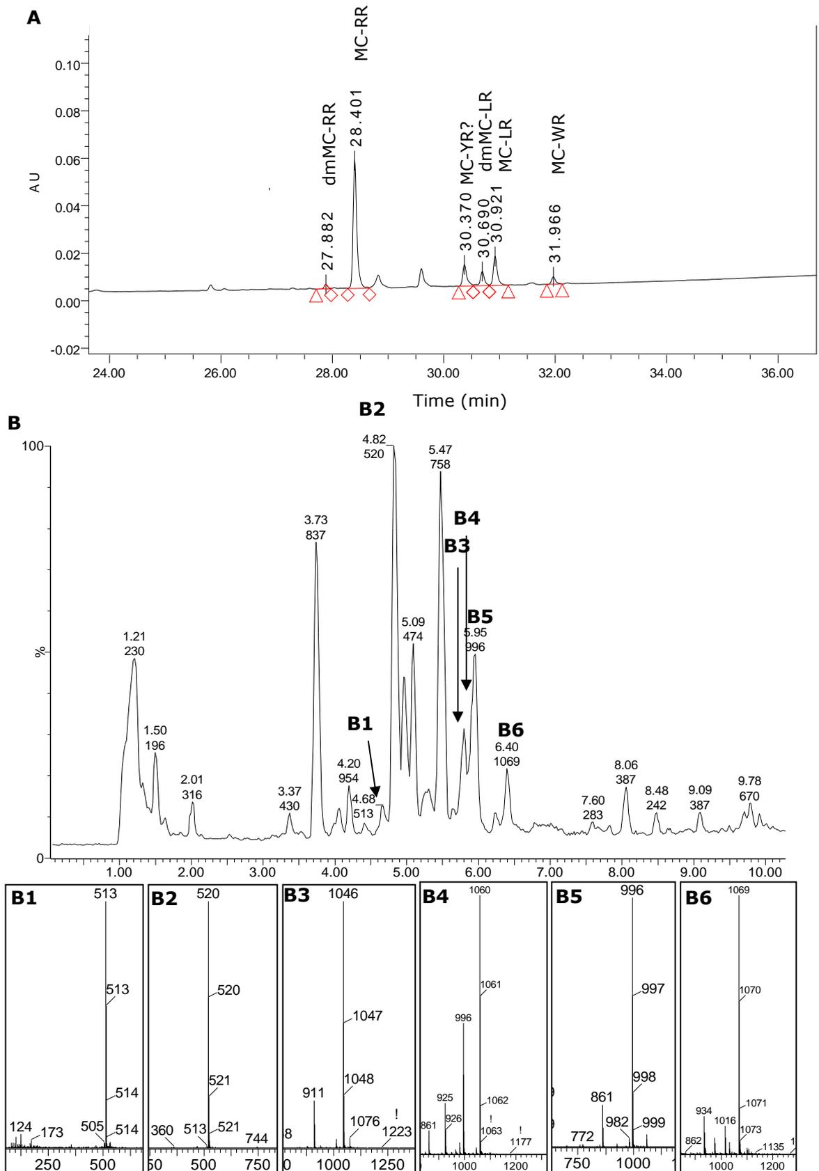
**Figure 2.35** HPLC-PDA chromatogram monitored at 238 nm (A) TIC UPLC-QToF-MS chromatogram (B) and mass spectrum (base peak) corresponding to dmMC-RR (B1), MC-RR (B2), MC-YR (B3), MC-HtyR (B4)MC-LR (B5), and MC-WR (B6) detected in *M. aeruginosa* SCIENTO.
