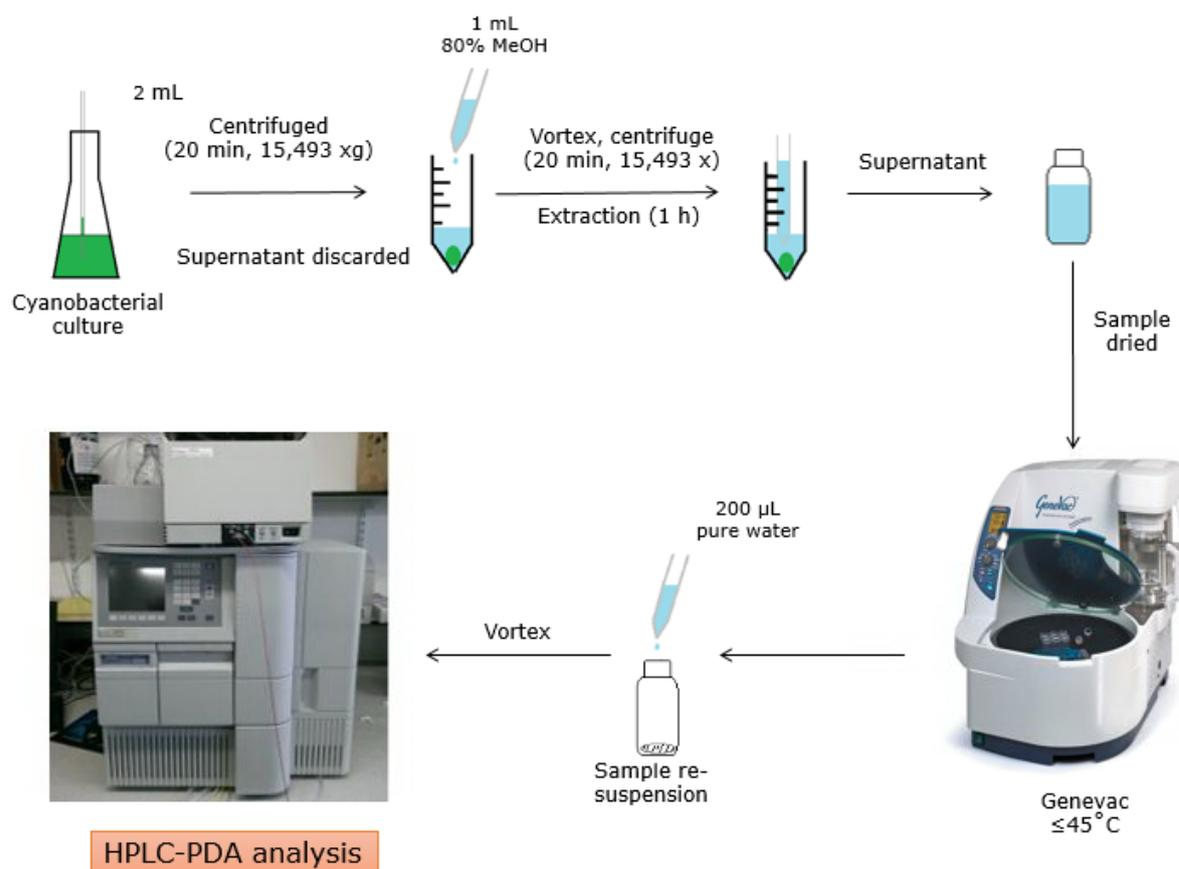
**Figure 2. 3** Cyanotoxin extraction from laboratory cultures (2 mL) which were centrifuged (20 min, 15,493 xg) and extracted with 80% aqueous MeOH. The supernatant was dried and the cyanotoxin content determined utilising the optimised HPLC-PDA method (section 2.2.2).
