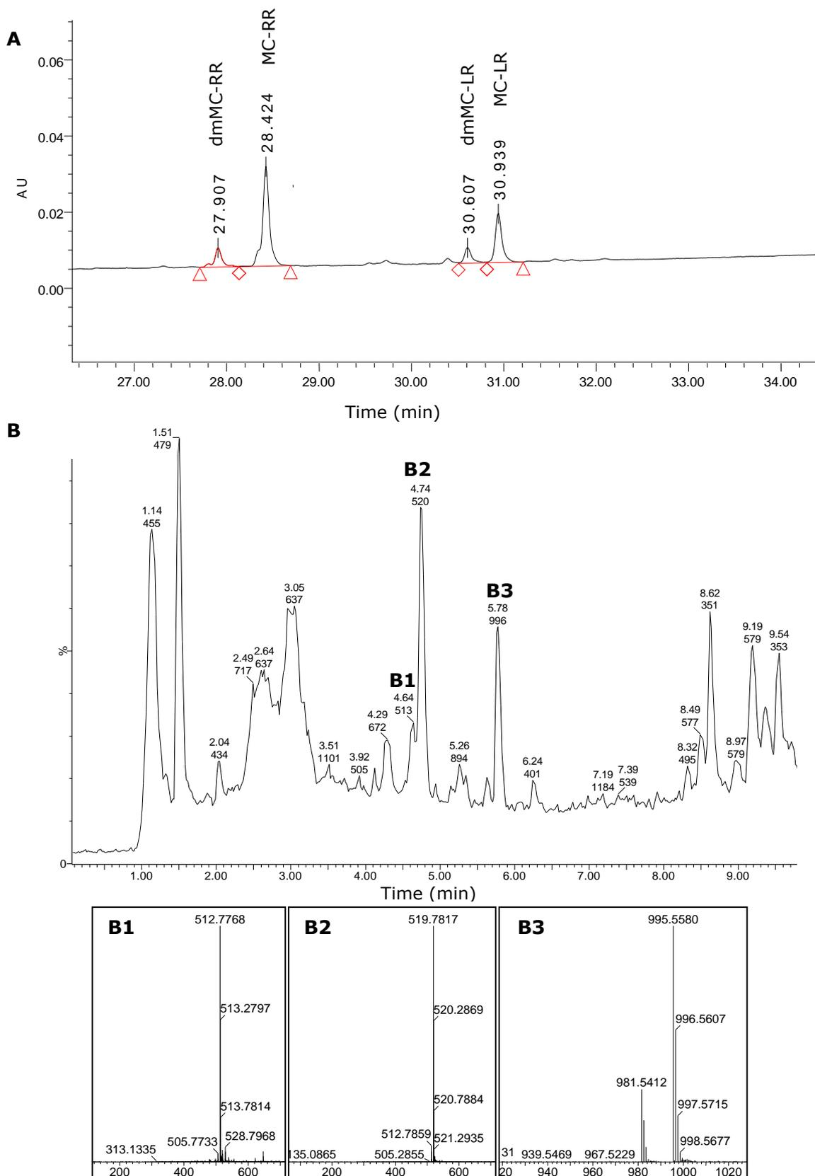
**Figure 2. 31** HPLC-PDA chromatogram monitored at 238 nm (A) TIC UPLC-QToF-MS chromatogram (B) and mass spectrum (base peak) of dmMC-RR (B1), MC-RR (B2), and MC-LR (B3) detected in *M. aeruginosa* NIES 1071.
