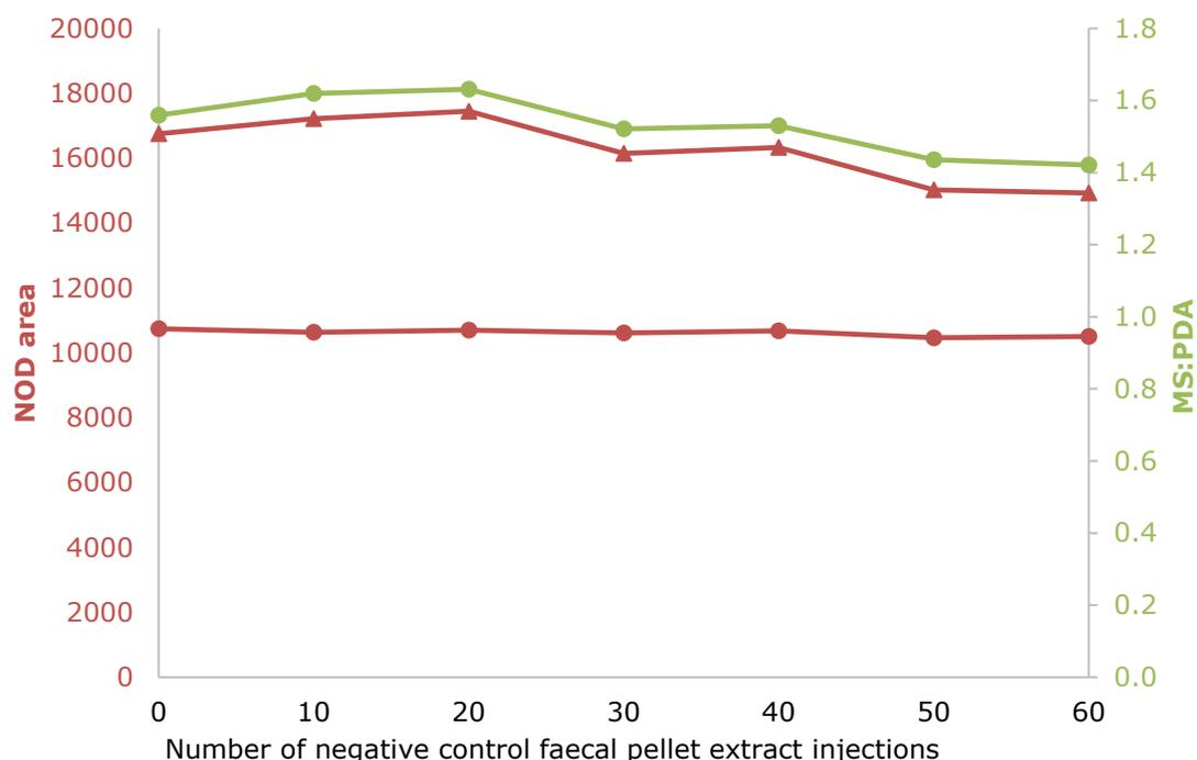
**Figure 3. 10** Change in NOD ( $10 \mu\text{g mL}^{-1}$ ) signal after injecting negative control faecal pellet extracts. Analysis was performed utilising UPLC followed by PDA (238 nm; red circles) and QToF-MS ( $m/z$  825; red triangles) detection. In addition, the ratio of MS to UV signal was determined (green circles).
