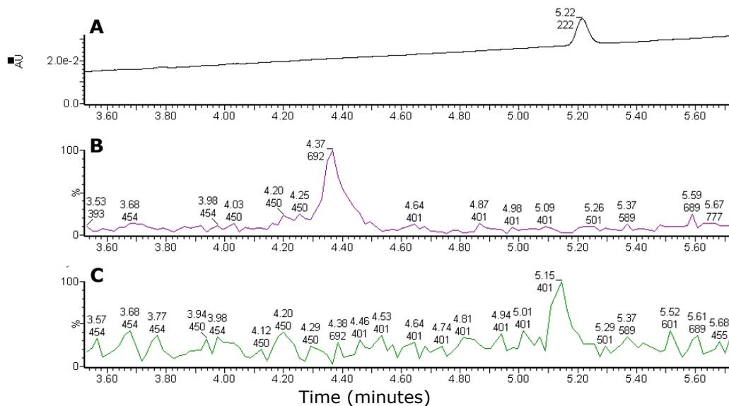
**Figure 3. 22** Free NODs detected in water sample following the exposure of *M. edulis* to *N. spumigena* KAC66. Samples were analysed utilising UPLC-PDA (238 nm; A) and UPLC-QToF-MS recorded at m/z 692 (LNOD; B) and m/z 825 (NOD; C)
