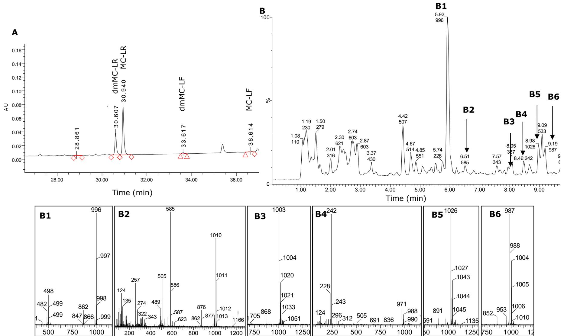
**Figure 2.33** HPLC-PDA chromatogram monitored at 238 nm (A) TIC UPLC-QToF-MS chromatogram (B) and mass spectra (base peak) of MC-LR (B1), mMC-LR (B2), MC-LY (B3), dmMC-LF (B4), MC-LW (B5) and MC-LF (B6) detected in *M. aeruginosa* PCC 7820.
