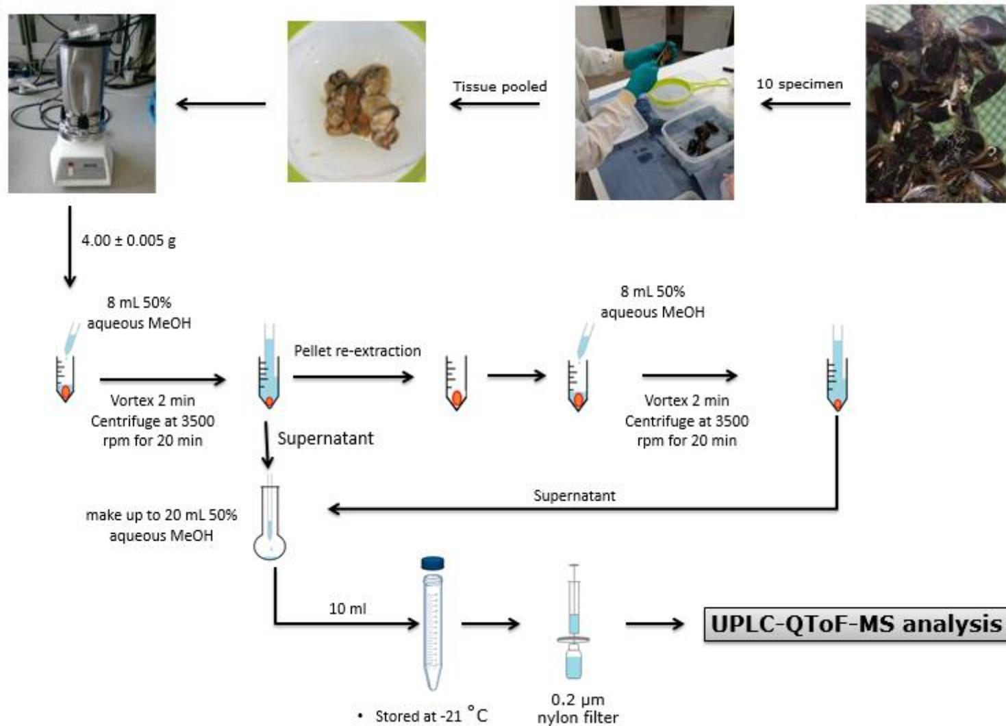
**Figure 3. 4** Double 50% aqueous MeOH extraction of NODs from *M. edulis* exposed to *N. spumigena* KAC66 or shellfish diet. Mussels (n=10) had been shuck, pooled, and pulse blended. All samples were analysed utilising UPLC-QToF-MS (n=3)
