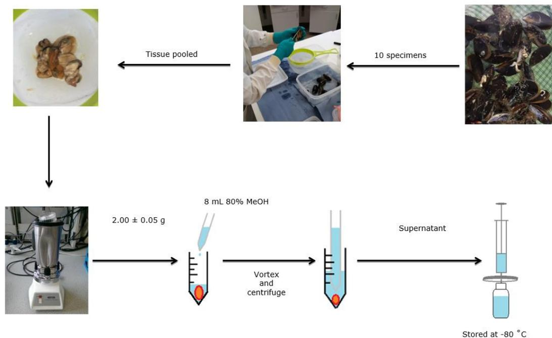
**Figure 5. 5** Extraction procedure for the analysis of *M. edulis* exposed to *N. spumigena* KAC66 and *M. aeruginosa* PCC 7813. Ten specimen were pooled, pulse blended and extracted in 80% MeOH. Thereafter samples were vortexed (2 min; 2,300 rpm), centrifuged (10 min; 2,279 xg) and supernatants transferred into UPLC vials. Extracts were stored at -80 until analysis.
