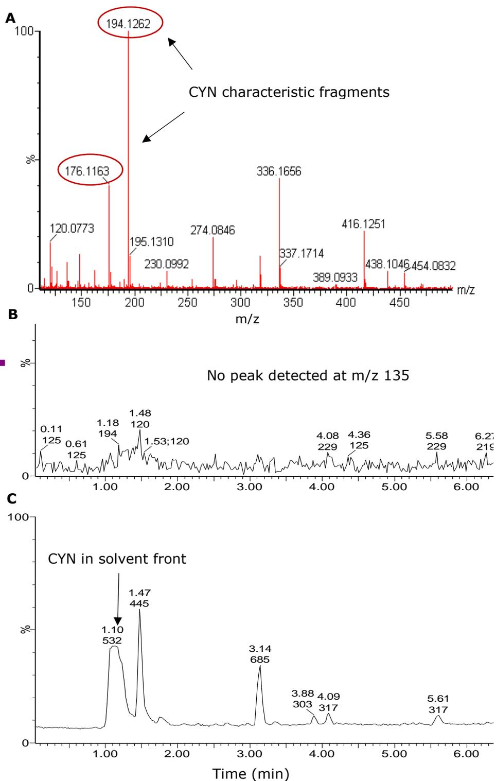
**Figure 2. 13** UPLC-QToF-MS analysis of *A. flos-aquae* PCC 7905 extracts. Extracted mass spectrum at  $t_R=1.27$  showing the CYN characteristic fragments at  $m/z$  176 and 194 (A)  $M^E$  chromatogram extracted at  $m/z$  135 which could not confirm the suspected presence of a polar MC (B). TIC chromatogram (C)
