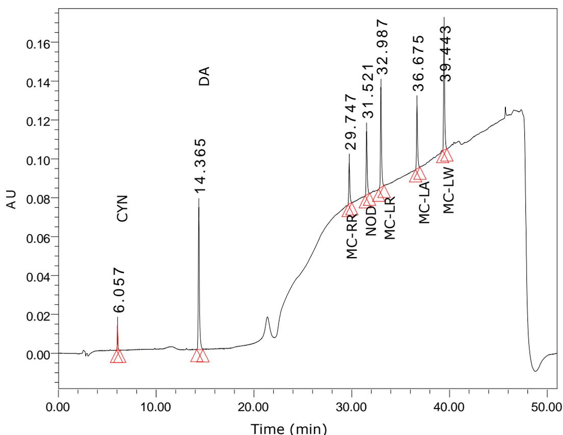
**Figure 2. 8** Improved HPLC-PDA separation of DA and six cyanotoxins with adjusted gradient (240 nm)
