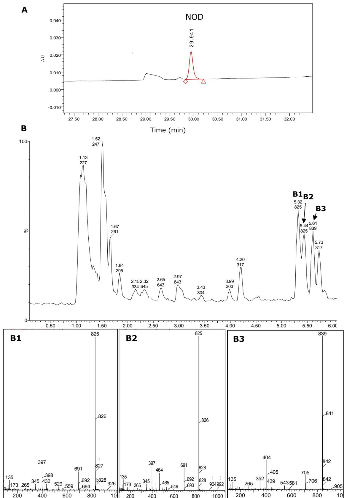
**Figure 2. 37** HPLC-PDA chromatogram monitored at 238 nm (A) TIC UPLC-QToF-MS chromatogram (B) and mass spectrum corresponding to NOD (B1), NOD (B2), and mNOD (B3) detected in *N. sphaerocarpa* PCC 7804.
