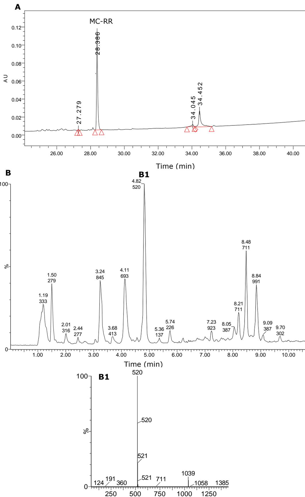
**Figure 2. 36** HPLC-PDA chromatogram monitored at 238 nm (A) TIC UPLC-QToF-MS chromatogram (B) and mass spectrum corresponding to MC-RR (B1) detected in *M. aeruginosa* SAT.
