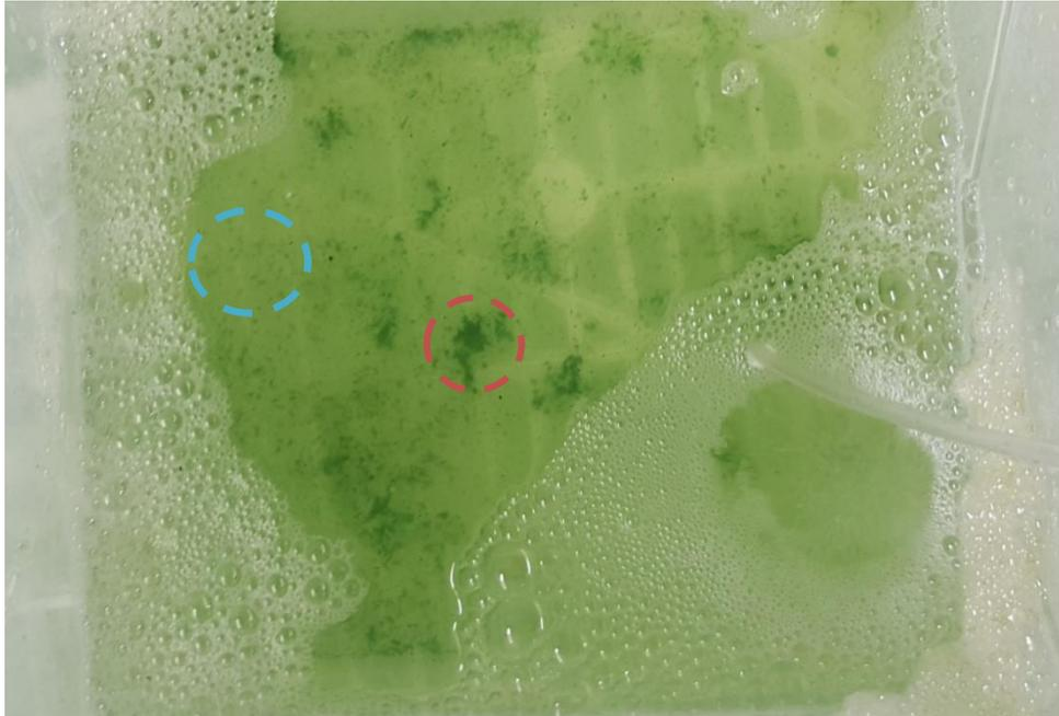
**Figure 5. 8** Experimental tank on day three (7:24 am) illustrating the observed lower clearance of *M. aeruginosa* PCC 7813 associated with the combined effect of aggregation and settling of *M. aeruginosa* PCC 7813 cells.
