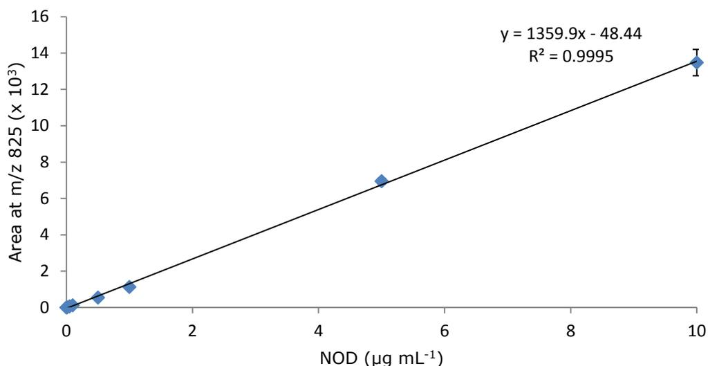
**Figure 3. 6** Linear calibration graph for NOD in 80% aqueous MeOH by UPLC-QToF-MS (m/z 825). Error bars represent standard deviations (n=3)
