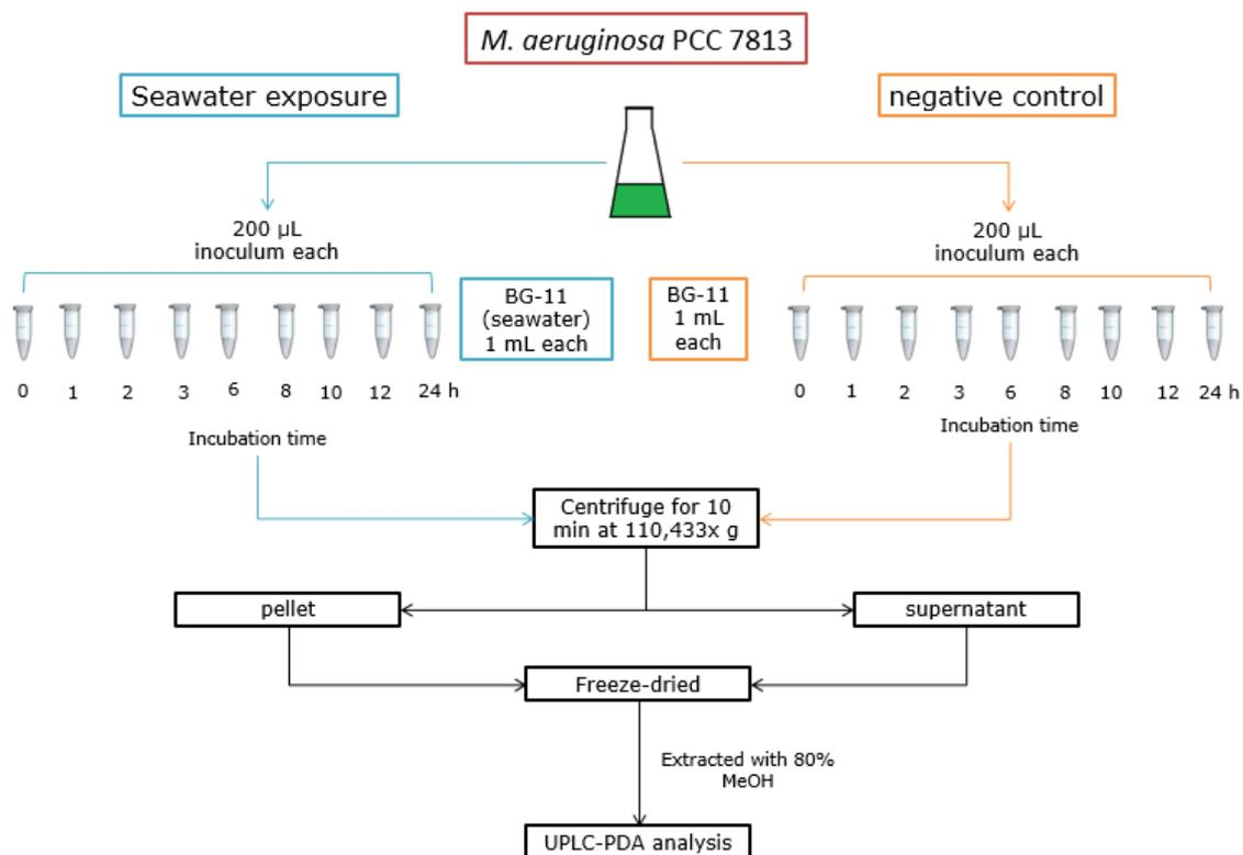
**Figure 4. 1** Schematic illustration of *M. aeruginosa* PCC 7813 salinity tolerance experiment. Following inoculation into BG-11 and BG-11 prepared with seawater, the intracellular and extracellular MC content was determined at different time points. Samples were centrifuged and supernatant and cell pellet freeze-dried, extracted with 80% aqueous MeOH and analysed utilising UPLC-PDA.
