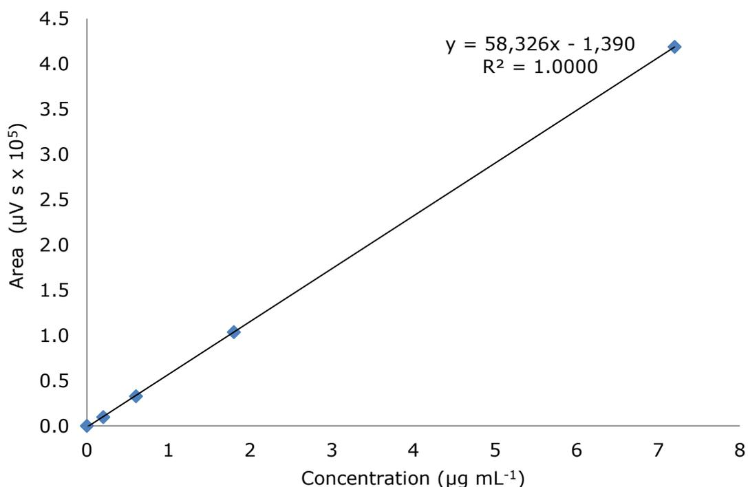
**Figure 2. 5** Calibration of DA in 5% aqueous MeCN obtained by HPLC-PDA monitored at 240 nm
