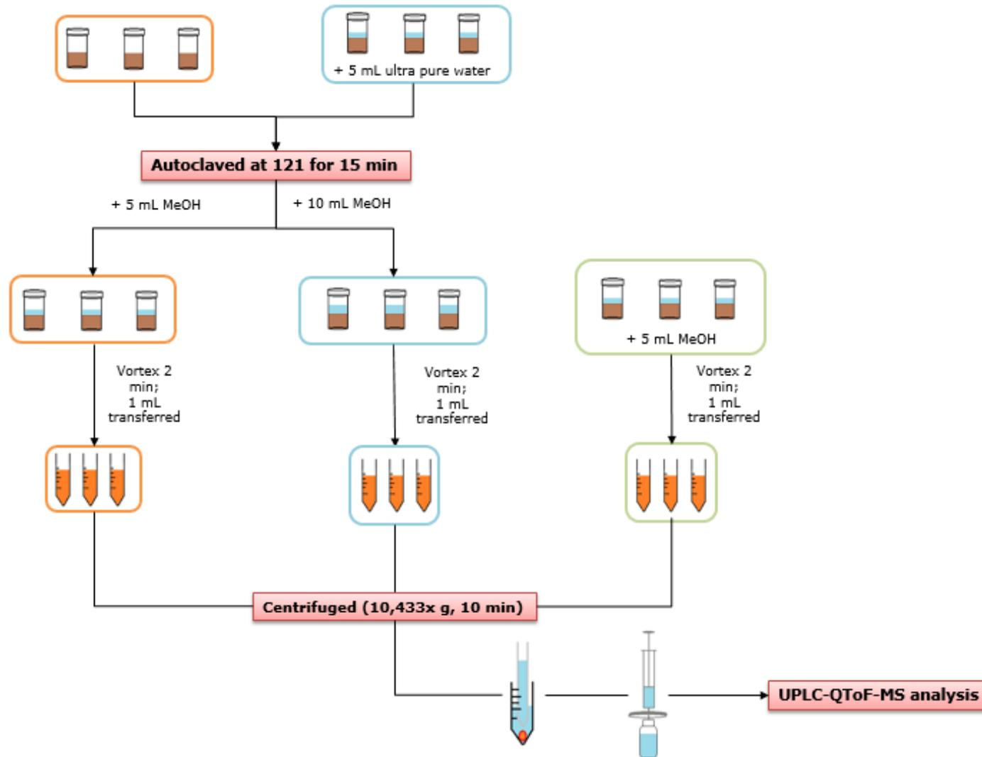
**Figure 5. 1** Different extraction procedures utilised for the detection of NOD and MCs in mussel homogenate by UPLC-QToF-MS analysis.
