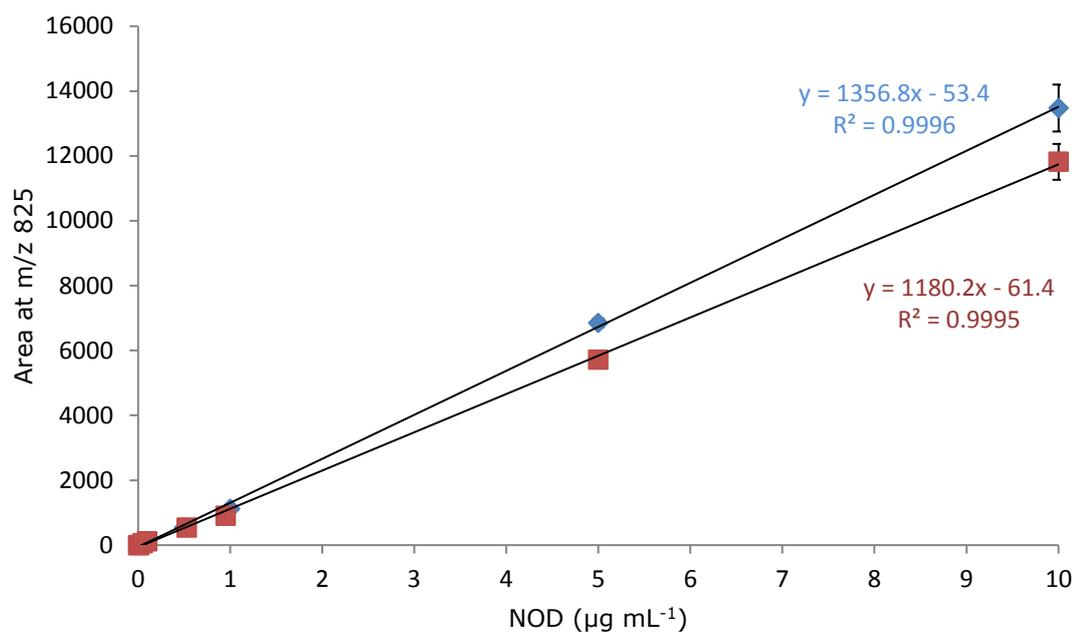
**Figure 3. 12** Calibration of NOD in 80% aqueous MeOH (blue) and negative control faecal pellet extracts (red) utilising UPLC-QToF-MS at m/z 825. Error bars represent standard deviation (n=3).
