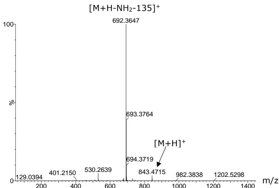
**Figure 3. 8** Mass spectrum of LNOD detected at  $t_R = 4.459$  min utilising UPLC-QToF-MS analysis.
