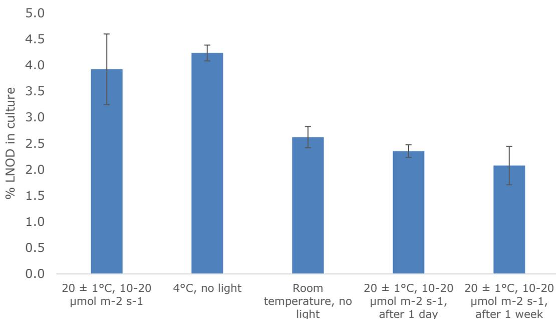
**Figure 3. 3** Percentage of combined intracellular and extracellular LNOD (m/z 692) compared to NOD (m/z 825) detected following sequential storage of *N. spumigena* KAC66 at varying storage conditions. Values are shown  $\pm$  standard deviation (n=2) as determined after UPLC-QToF-MS analysis.
