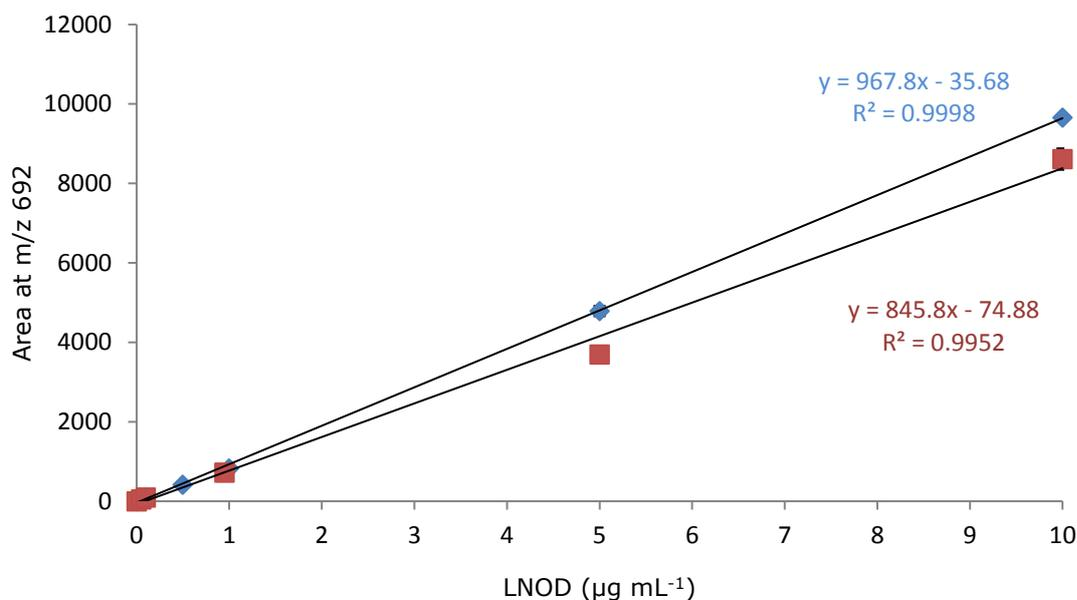
**Figure 3. 16** Calibration of LNOD in 80% aqueous MeOH (blue) and negative control faecal pellet extracts (red) utilising UPLC-QToF-MS at m/z 692. Error bars represent standard deviation ( $n=3$ )
