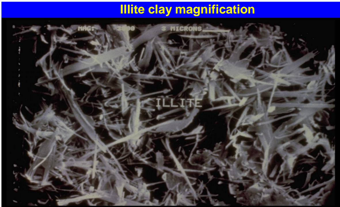
Figure 2.2: Fines particles at different scales: illite and feldspar
