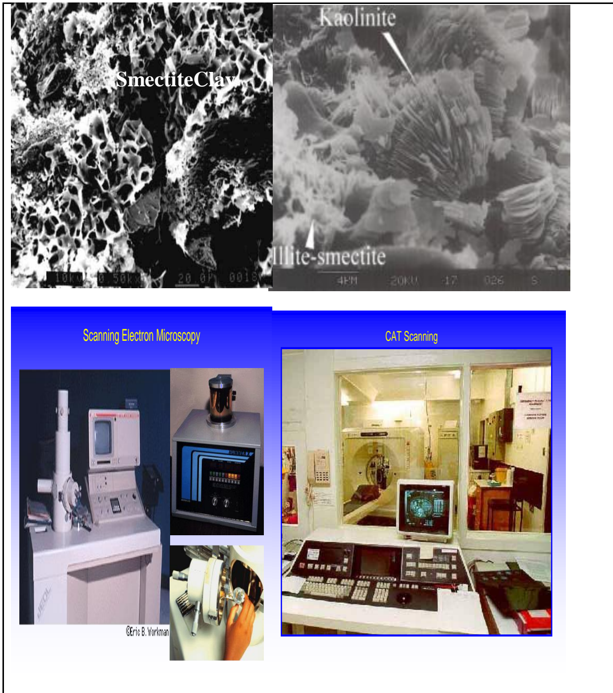
Figure 2.1 : Images of kaolinite, illite-smectite fines and measuring devices
