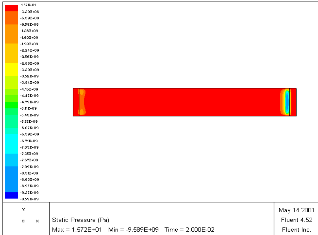
Figure 3.16: Pressure profiles when 10 \mu\text{m} fines flow in a multiphase fluid was simulated.
