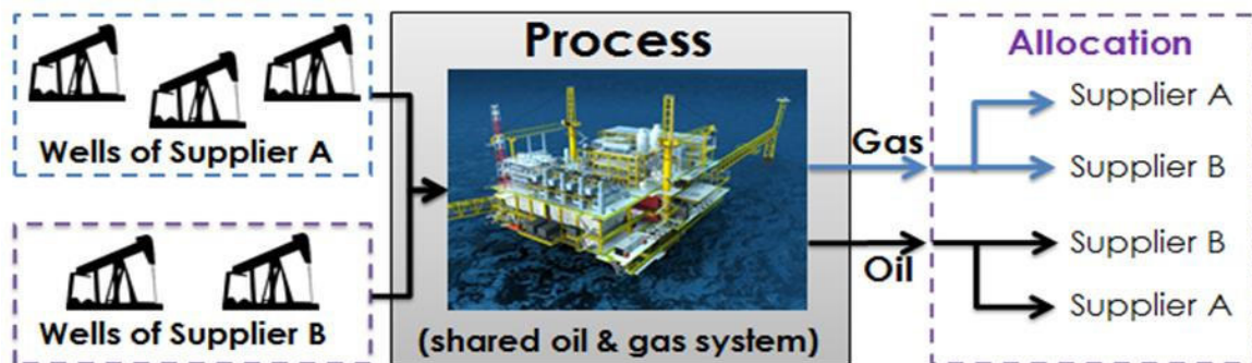
Fig. 2.3 Hydrocarbon Allocation - Suppliers A and B wish to know what fraction of the Export Gas and Oil produced is theirs
