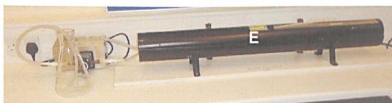
Figure 5.2: Completed fixed film flow reactor. (A) Sample reservoir; (B) pump; (C) glass spiral coated with catalyst; (D) UV tube light and (E) foil lined coil casing as closed during operation.
