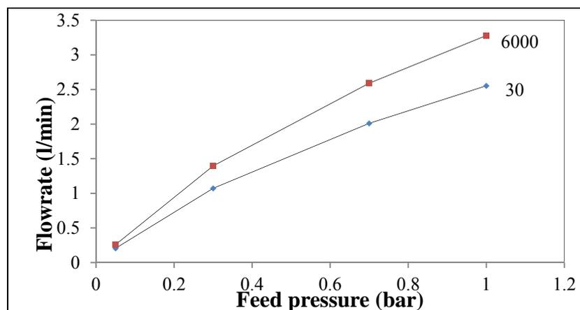
Figure 2.  $\text{H}_2$  flow rate as a function of feed pressure for 30 and 6000 nm at 298 K.
