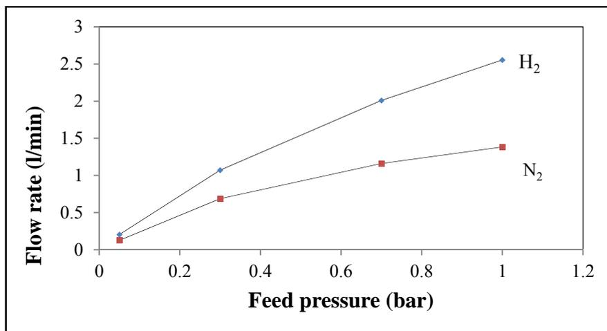
**Figure 4.** H<sub>2</sub> and N<sub>2</sub> flow rate as a function of feed pressure for 30 nm at 298 K.
