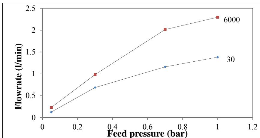
**Figure 3.** N<sub>2</sub> flow rate as a function of feed pressure for 30 and 6000 nm at 298 K.
