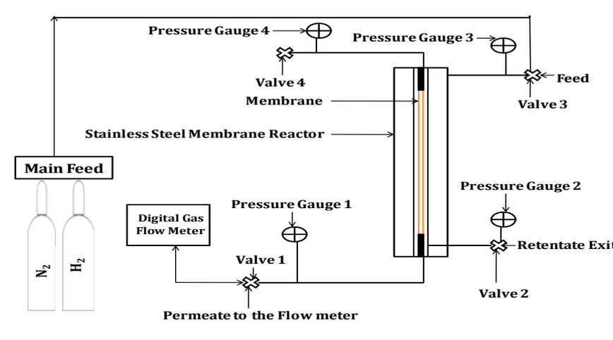
Figure 1: Permeation test experimental system.
