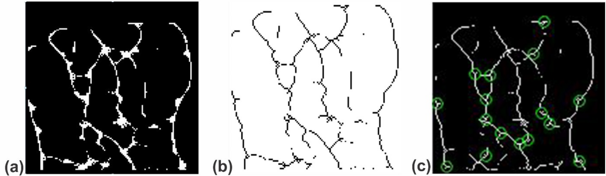
Fig. 5(a) shows the pattern obtained using maximum curvature method (b) the vein pattern after thinning operation (c) the output image with extracted minutia (bifurcation)
