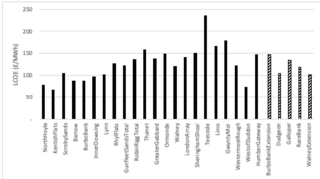
Figure 2: LCOE for all projects, chronological order by commissioning (authors' analysis). (NB solid bars show data for wind farms with full accounts-based and historic production data, striped where assumptions are used on capacity factor, OFTO transfer and operating costs)
