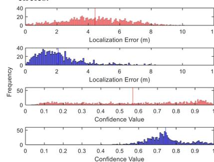
Fig. 4. Histograms of localization error and confidence value of a single node in both a non-optimal case ( $x_1=0.9$  and  $x_2=6.35$ ; red) and the optimal case ( $x_1=0.7$  and  $x_2=26$ ; blue) over 1000 localization period with mean localization error of 4.42 m and 2.08 m and mean confidence value of 0.56 and 0.74 in the non-optimal and the optimal cases respectively.
