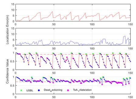
Fig. 5. Traces of typical localization errors and confidence values of a single node over the first 150 localization period in the non-optimal case (red) and the optimal case (blue). The red dashed horizontal lines represent confidence thresholds.
