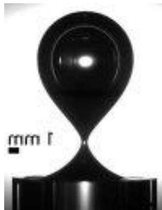
**Figure 2.8** : Photography of an air bubble just before pinch-off from a nozzle (59)
