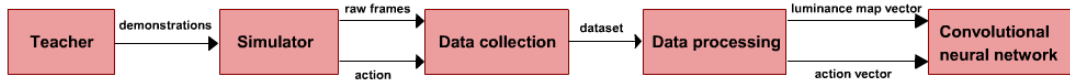
Figure 4.2: Workflow of the learning representation process. The process starts by a teacher providing demonstrations on a given simulator. The demonstrations are collected and processed into a dataset that is fed into a deep convolutional neural network. The network learns high level representations of the raw input features as well as mapping to the action space.
