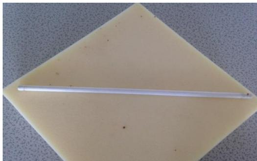
Figure 1: Porous tubular alumina support.
