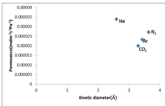
Figure 6: Permeance against gas kinetic diameter at 25 °C.
