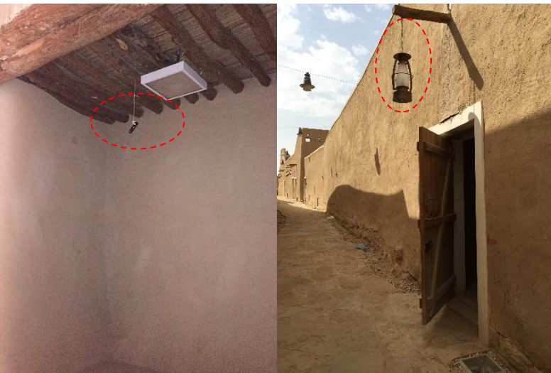
Figure 9. Historical Ad Diriyah block B8-2 indoor/outdoor, showing data logger (red circle).
