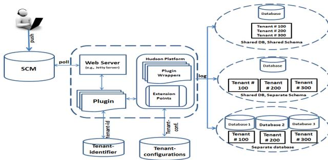
Figure 2. Multitenancy Data Isolation Architecture
