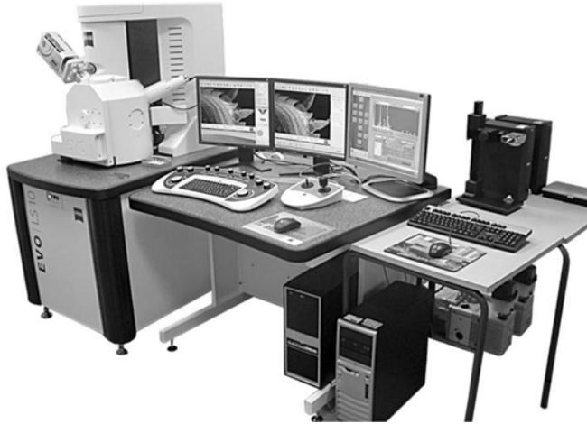
Fig. 2. Pictorial diagram of the SEM-EDXA
