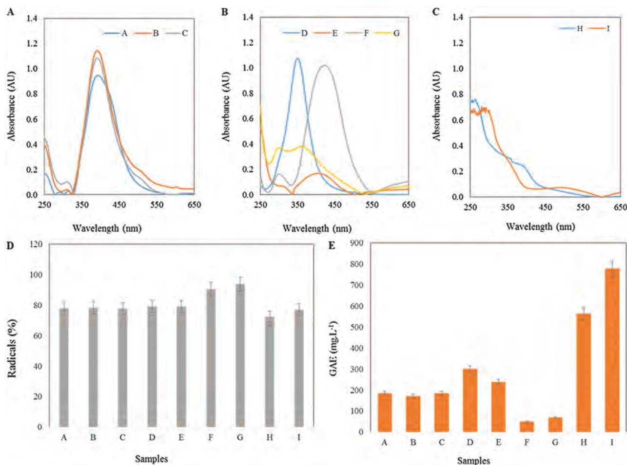
**Figure 4.** (A–C) UV-vis absorbance spectra of prepared AgNPs over the range from 250 to 650 nm. The concentration of analysed nanoparticles was 2 mg/mL. (D) Graph of DMPD radicals quenched by AgNPs (2 mg/mL) expressed as the percentage of remaining radicals. (E) Graph of antioxidant activity of AgNPs (2 mg/mL) measured by FR method. Further details are described in the materials and methods section.
