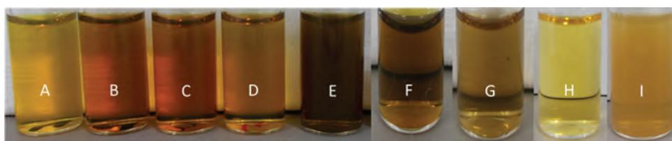
**Figure 2.** AgNPs formed by two ways of chemical synthesis using different reduction agents (A–C)  $\text{NaBH}_4$  and (D–G) gallic acid at various pH. Samples H and I are AgNPs produced by the green synthesis using tea and coffee extracts. The preparation protocol for each AgNPs are shown in materials and methods.
