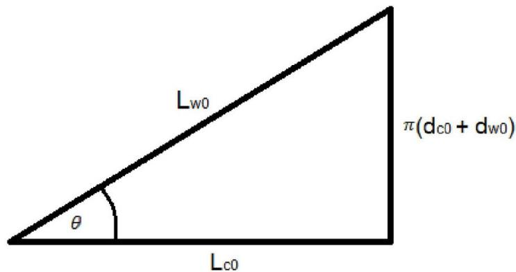
**Figure 1.** Right-angled triangle formed if the wrap was unravelled from the core (adapted from ref. [14]).
