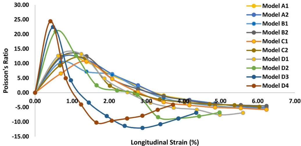
**Figure 4.** Graph of longitudinal strain vs. Poisson's ratio of HAY for all finite element computational models tested using ANSYS® Workbench [figures appear in colour in the online version].
