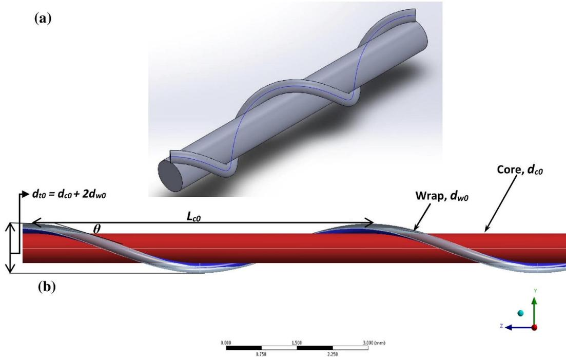
**Figure 2.** (a) Two cycle model of HAY created in SOLIDWORKS® 3D CAD software, and (b) HAY connections showing the contact region between the wrap and core, highlighted in blue and red, respectively.
