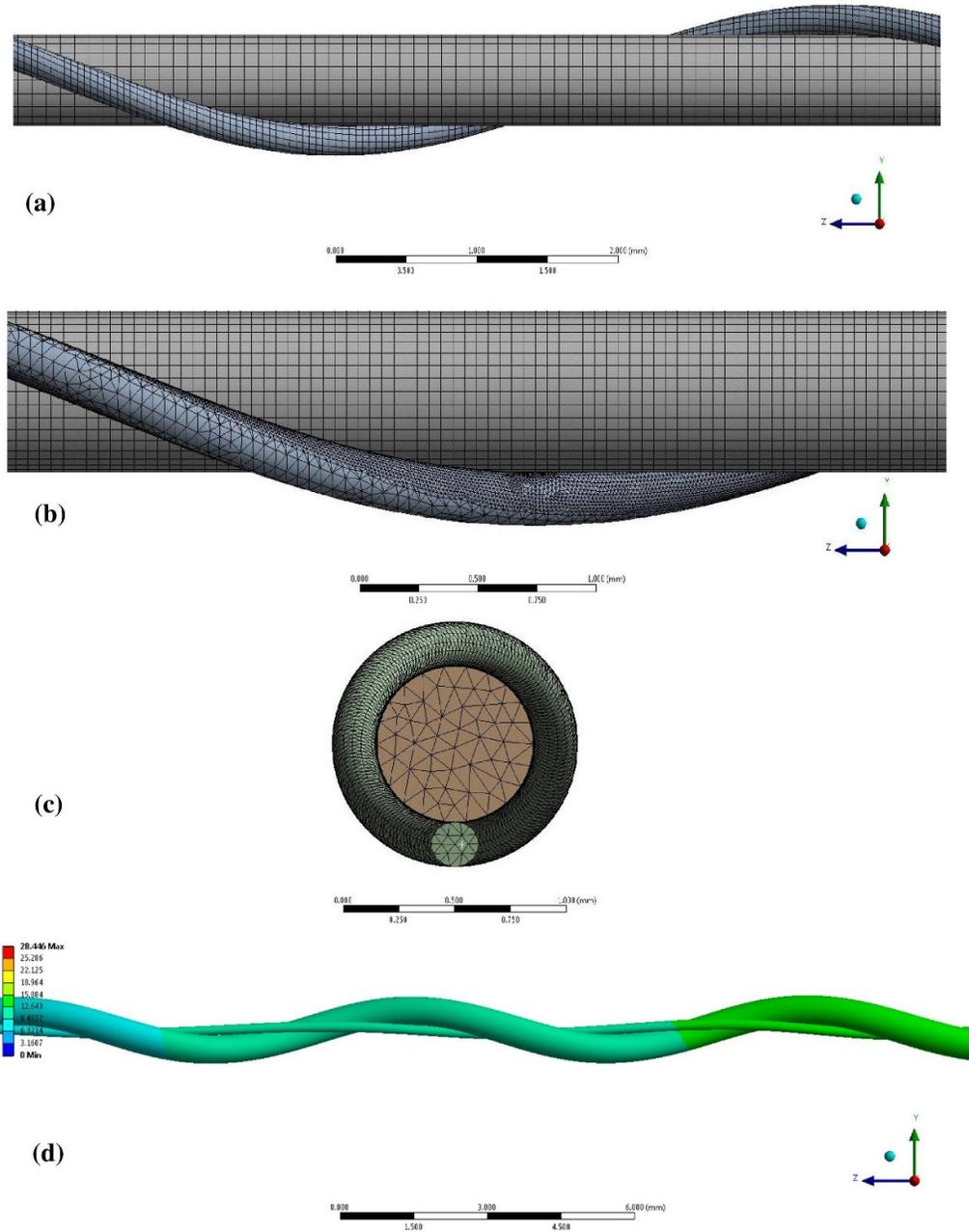
**Figure 3.** (a) Final mesh sizing of largest surface areas of HAY components, (b) invalid model with refined mesh on contact region of wrap, (c) cross-sectional area of mapped face meshing applied to model, and (d) fully deformed HAY after tensile test had been simulated.
