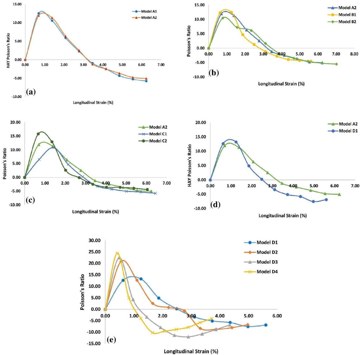
**Figure 5.** Graph of HAY Poisson's ratio vs. longitudinal strain (finite element computational models using ANSYS® Workbench): (a) for Model A1 and Model A2, showing the point at which both designs' maximum NPR values were achieved, (b) for Model A1, B1 and B2, (c) for Model A2, C1 and C2, (d) for Model A2 and D1, and (e) for models used in critical angle test [figures appear in colour in the online version].
