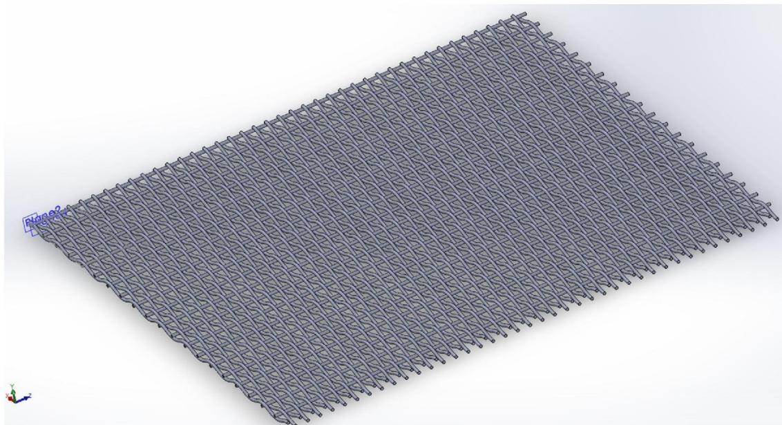
*Figure 6. Unused conceptual model of high velocity impacts resistant blanket created in SOLIDWORKS® 3D CAD software.*
