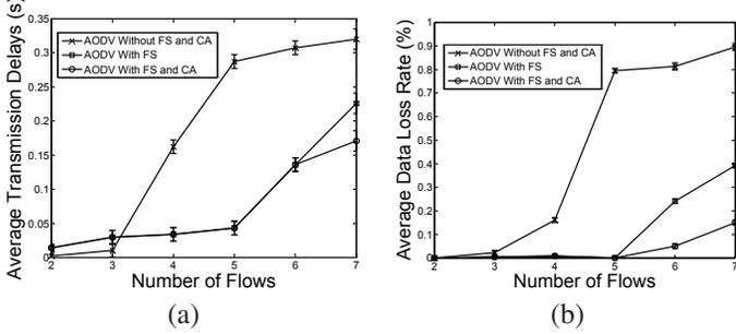
Fig. 10. The average delays (a) and the average data loss rates (b) achieved in the 4-hop simulations when the number of video flows increases.
