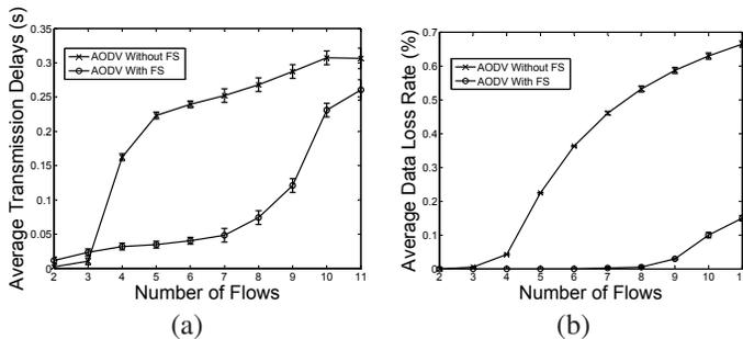
Fig. 7. The average delays (a) and the average data loss rates (b) achieved by the single-hop simulations when the number of flows increases.
