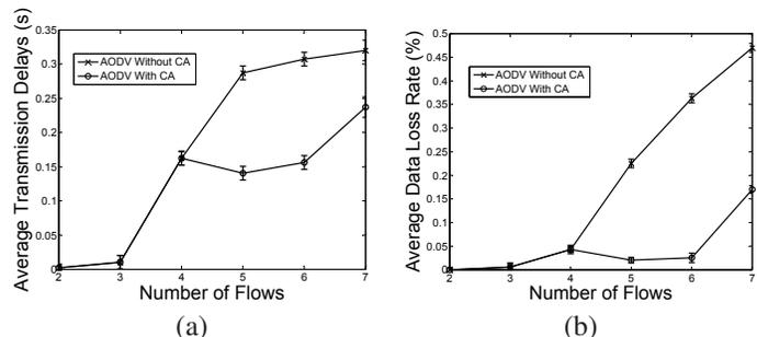
Fig. 9. The average delays (a) and the average data loss rates (b) achieved by the single-hop simulations when the number of video flows increases.
