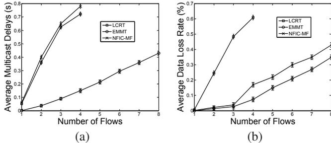
Fig. 12. The average multicast delays (a) and the average data loss rates (b) of EMMT and LCRT in the single-channel network when the number of multicasting flows increases.
