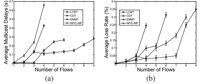
Fig. 13. The average transmission delays (a) and the average packet loss rates (b) of the three schemes in the multi-channel network when the number of flows increases.
