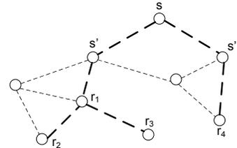
Fig. 6. An example of multicasting flows with the EMMT algorithm.
