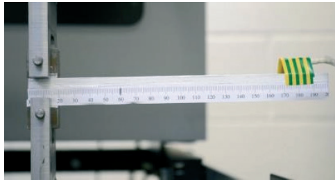
Figure 1: DCB experimental set-up2.
