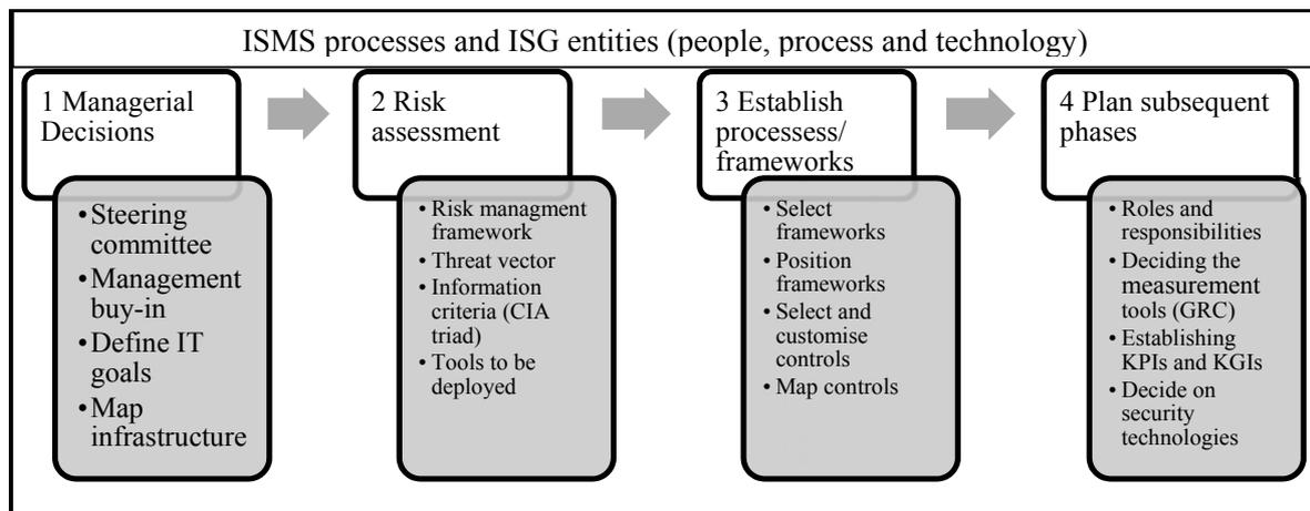
Figure 2. Plan stage of the ISG process
