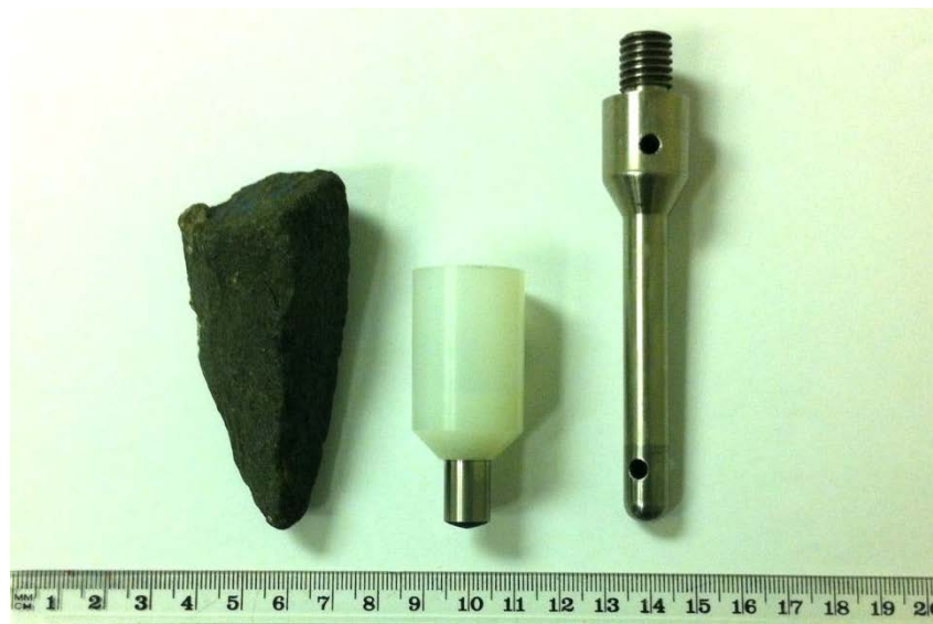
Figure 5 - Road stone, projectile and impactor
