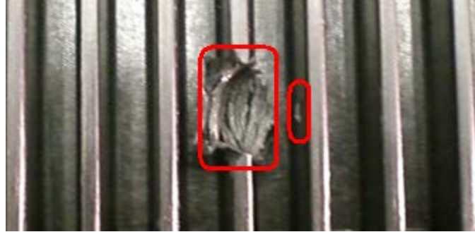
Figure 16 - Rib crushed after impact on rib at 7 J (PA66-i-Gf35)
