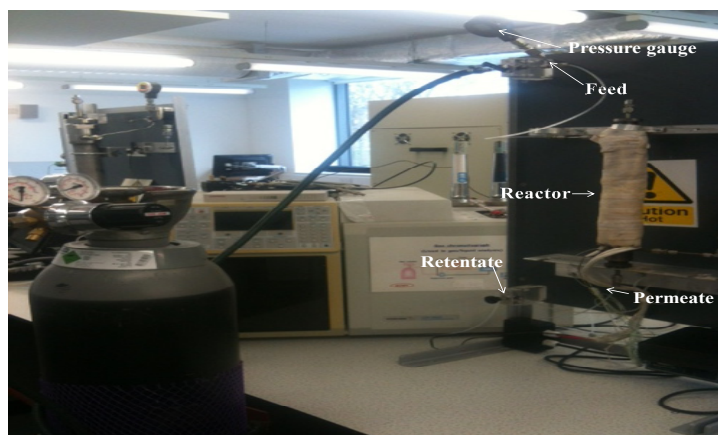
Figure 6. Experimental arrangement for the membrane reactor
