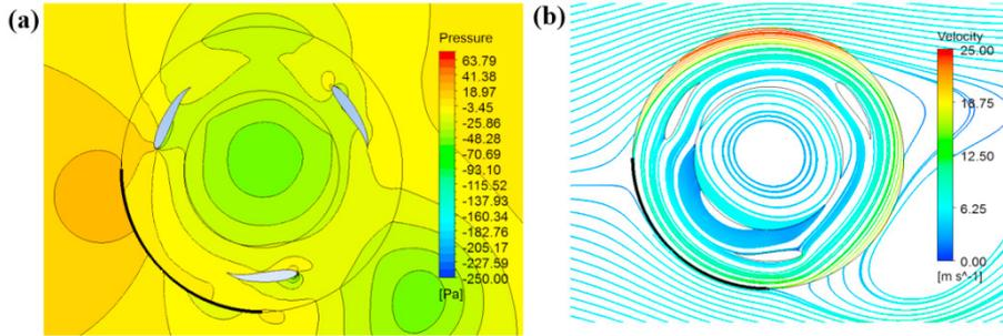
Fig. 3. Setup A ( $\phi = 90^\circ$ ): (a) Pressure contours, (b) Velocity streamlines.
