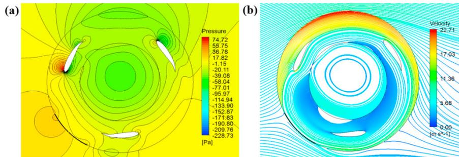
Fig. 6. Setup D ( $\phi = 36^\circ$ ): (a) Pressure contours, (b) Velocity streamlines.
