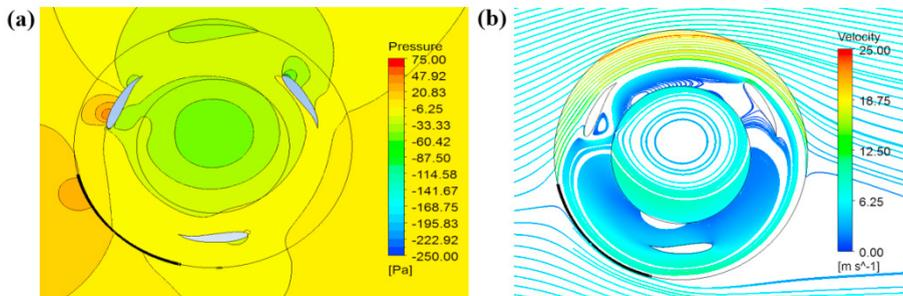
Fig. 4. Setup B ( $\phi = 63^\circ$ ): (a) Pressure contours, (b) Velocity streamlines.
