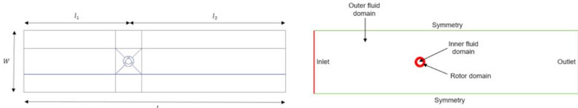
Fig. 1. (a) Computational domain; (b) Boundary conditions.
