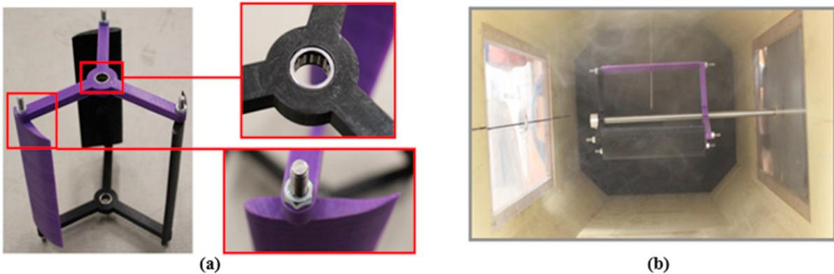
Fig. 8. Experimental Model (a) Fully Constructed (b) Position within Wind Tunnel.
