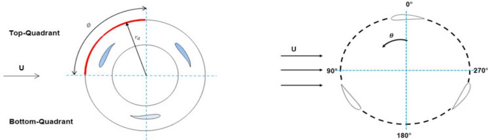
Fig. 2. Deflector Modelling (a) Dimensions (b) Azimuth Angle Measurement Method.
