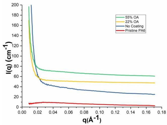
Figure S3. Background corrected SAXS intensities  $I(q)$  as a function of the scattering vector ‘ $q$ ’ for all the samples studied.
