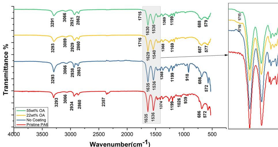
Fig. 3. ATR-FTIR spectra of pristine PA6, PNC containing uncoated NPs and PNC containing NPs with varying proportions of OA coatings.
