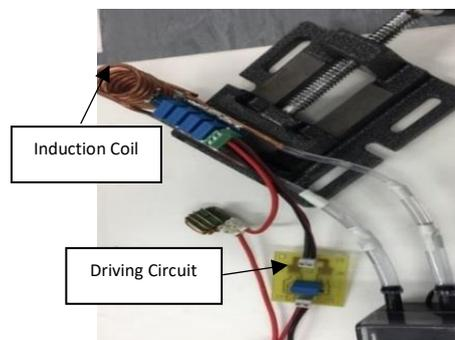
Figure S4. Magnetic coil setup for melt-characteristic testing.
