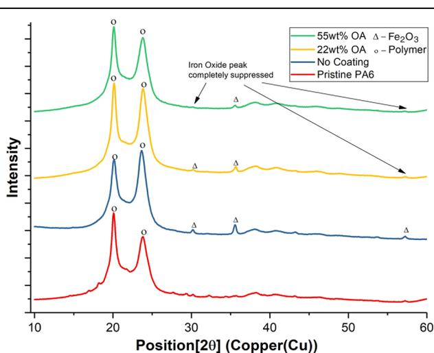
Fig. 6. XRD patterns of the PA6 samples with varying percentages of OA loading of coatings on the NPs. The triangle ( $\Delta$ ) and circle ( $\circ$ ) represents the peaks related to iron oxide and polymer, respectively.
