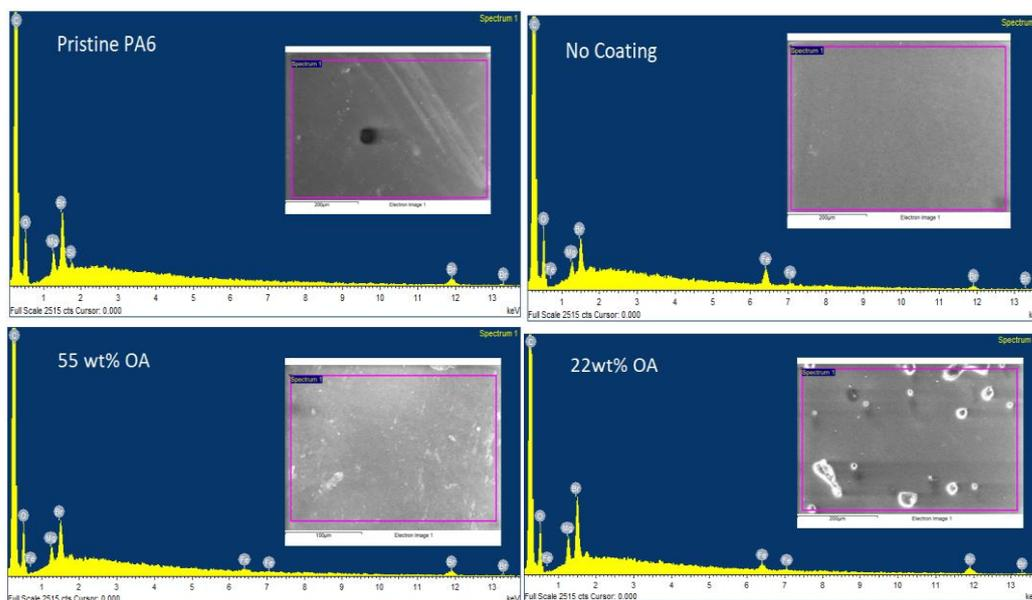
**Figure S2. EDX spectra demonstrate the Fe peaks are observed in all samples, except the Pristine PA-6 sample. (Clockwise from top-left: (a) Pristine PA6, (b) No Coating, (c) 22 wt% OA and (d) 55 wt% OA)**
