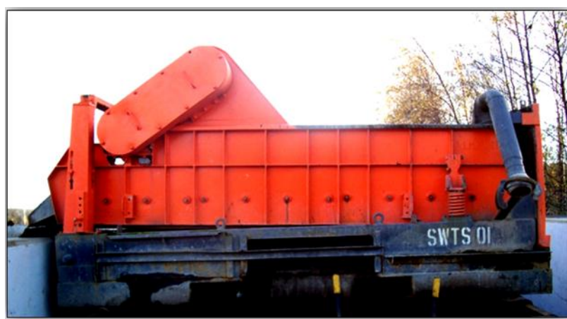
Figure 4-4 A photo of Sureclean shale shaker (previously known as SWTS 01), which removes heavy solids from liquid waste streams.
