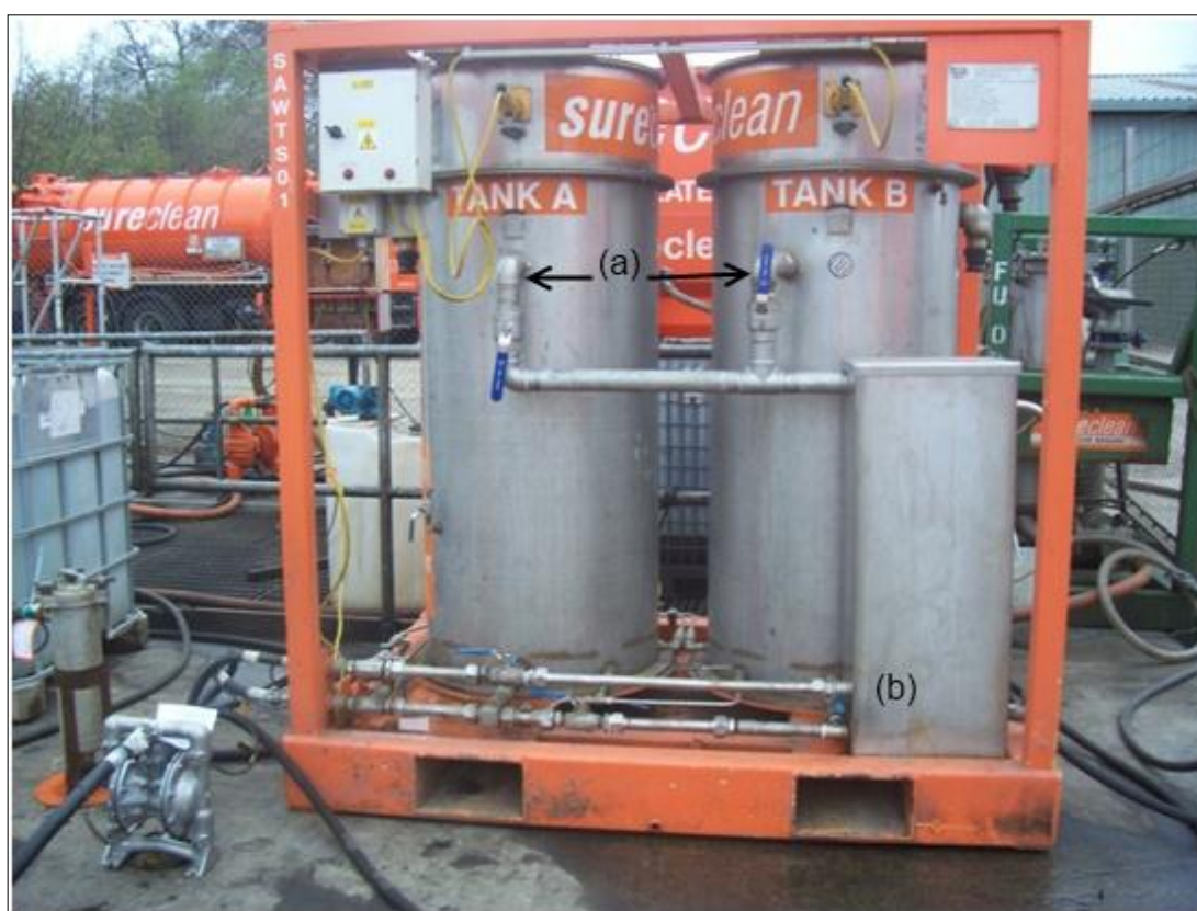
Figure 7-24 shows the refurbished SAWTS with (a) an enlarged outlet for SAWTS and (b) extra tank to enable effluent collection.
