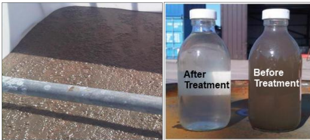
Figure 7-7 shows (Left) Formation of contamination 'float' in IBC; (Right) before and after effluent samples of Alness Interceptor Effluent.
