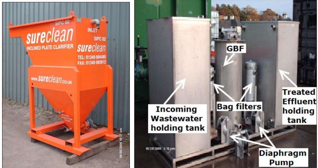
Figure 4-25 photograph of the individual components inside the SWTS01: an inclined plate clarifier (left) and the glass media filter (right) with two bag filters and two holding tanks).
