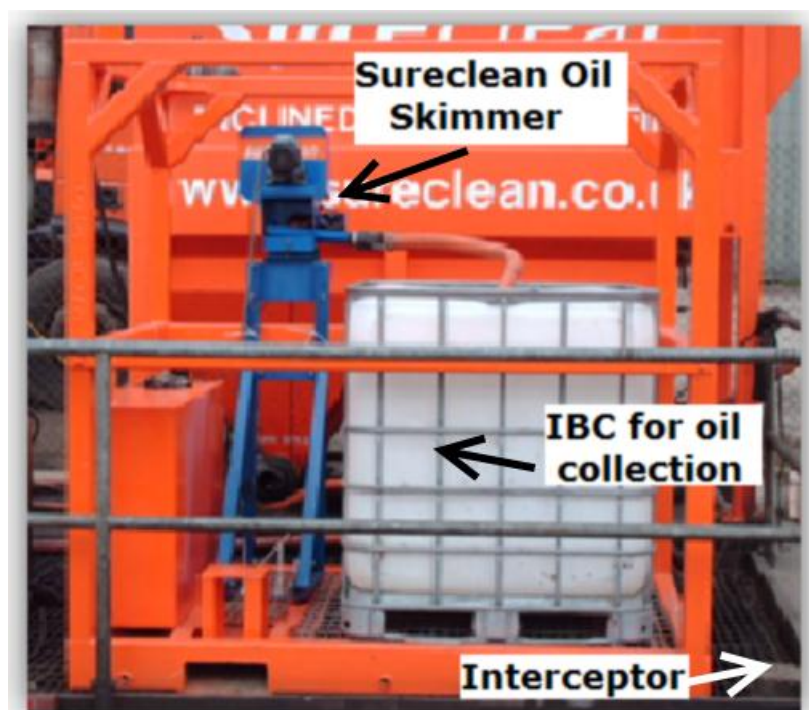
Figure 4-2 A photo of the Sureclean Oil Skimmer (painted in blue) that recovers oil from the interceptor underneath the unit; recovered oil was collected in an IBC (white container on the right of the skimmer).
