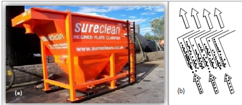
Figure 4-3 displays (a) a photo of the Sureclean Inclined Plate Clarifier; (b) the mechanism of the clarification: solid accumulate at the bottom of the inclined plate, and the clean water move upwards and out of the plates (Guyer 1998).
