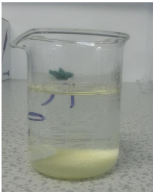
Figure 3.5 : Chitosan settled in naphthalene solution
