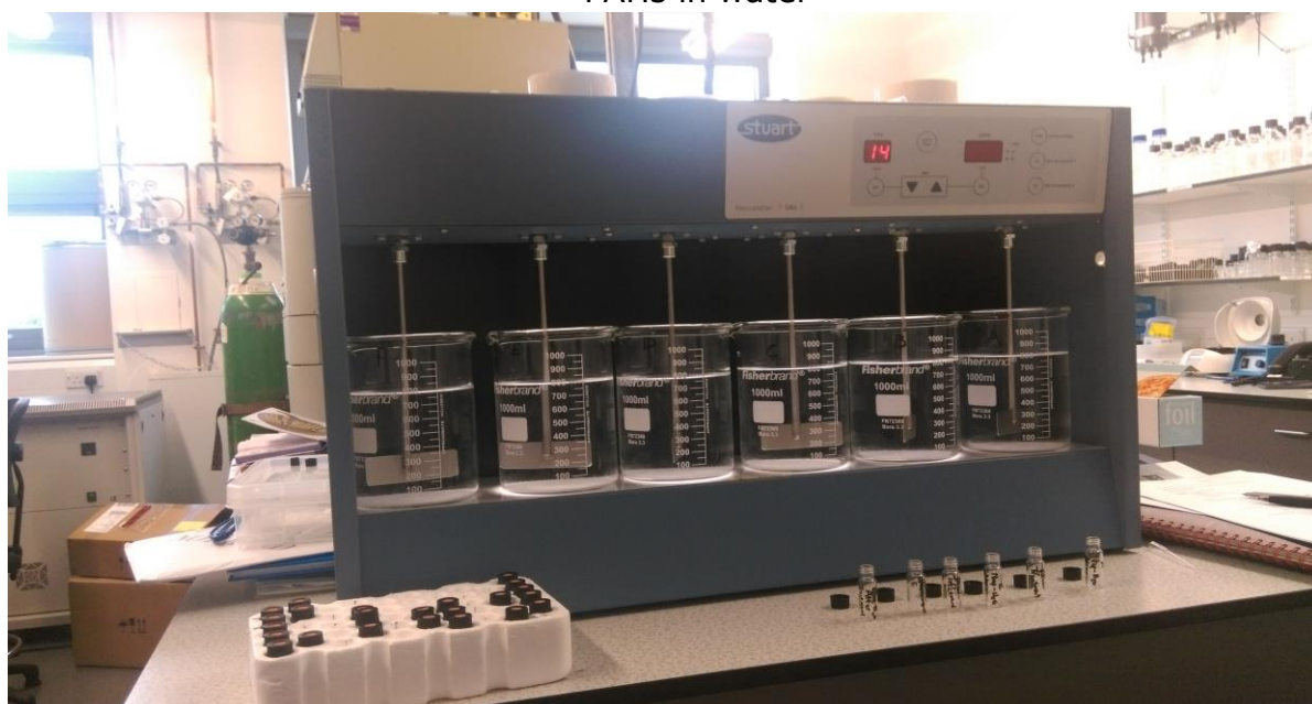
Figure 3.3 – Experimental protocol for powder chitosan for the adsorption of PAHs in water
