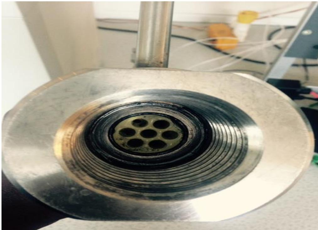
Figure 4.17 - Pictorial view of membrane with the stainless steel reactor showing the graphite ring seals.
