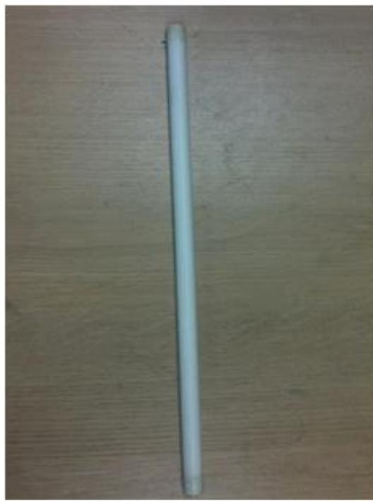
Figure 3.3 - Pictorial view of commercial tubular ceramic support.
